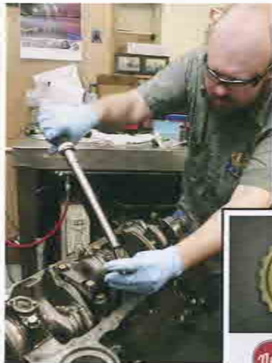
10 Between the first and second day of assembly, builder Ken Troutman fell ill so other members of the shop took over. Here, Kevin Troutman finishes the short-block, torquing the rod bolts to 65 ft-lb to achieve the proper bolt stretch.
