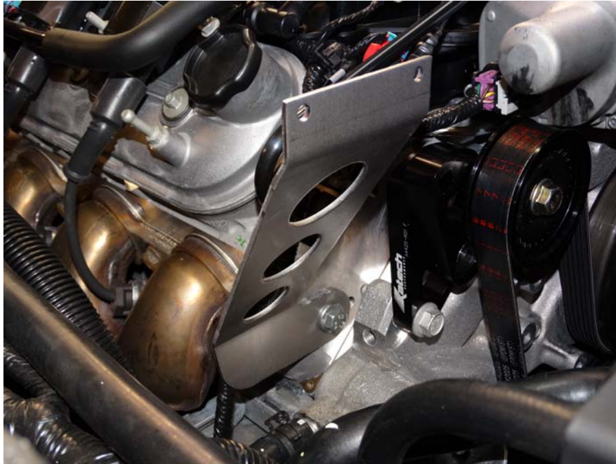
Step 7: Install stainless mounting bracket as shown using M10x20 HHCS.
