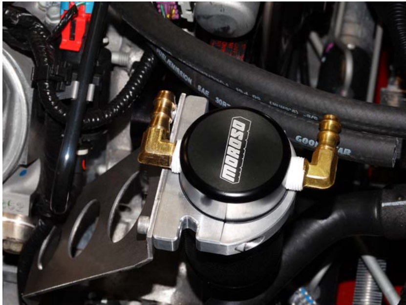
Step 10: Assemble billet clamp to stainless mounting bracket using (2) ¼-20x5/8 SHCS, be sure that reliefs in billet clamp are facing down. Insert Air Oil Separator into billet clamp.
