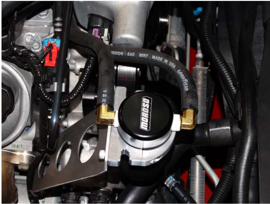
Step 13: Trim hose as needed and assemble to Air Oil Separator.
