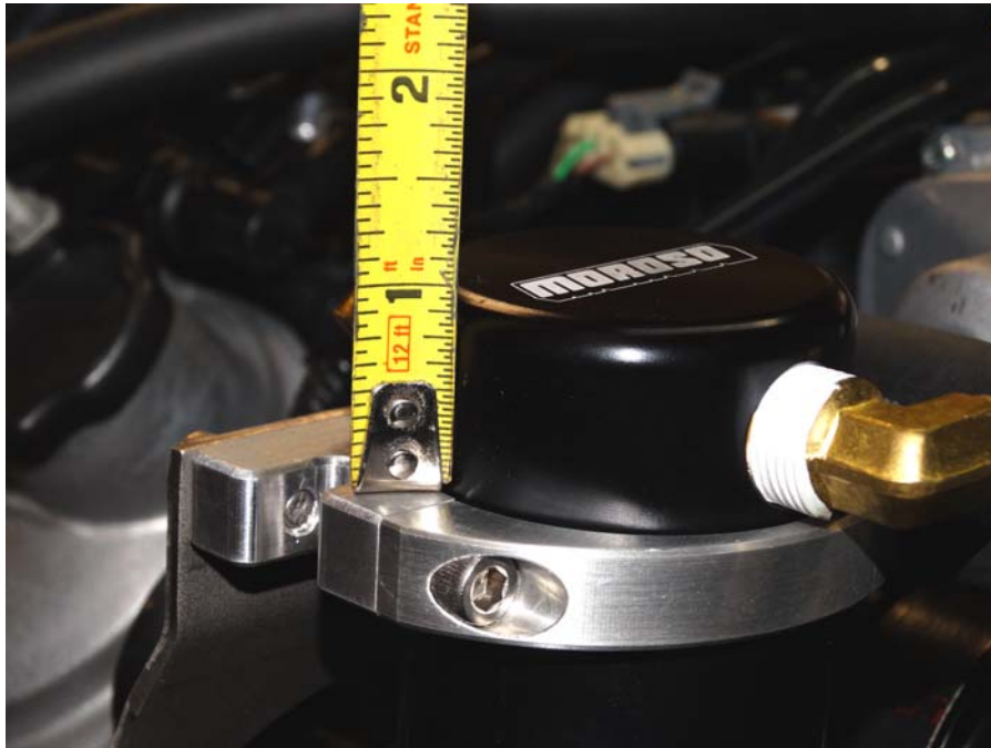
Step 11: Set height to 1-1 1/8 and tighten bile clamp.
