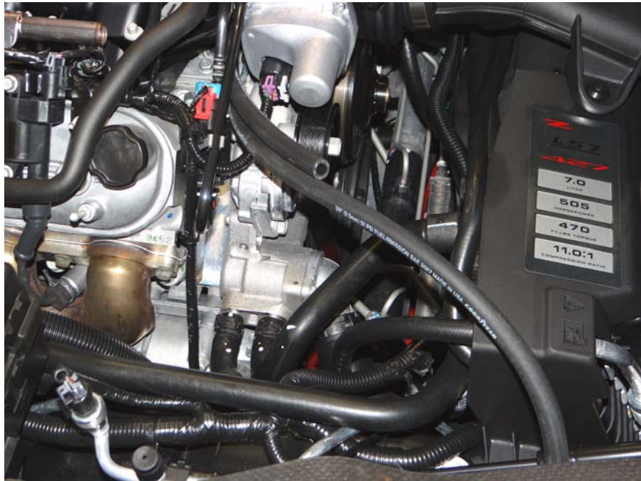
Step 5: Insert 2nd length of hose provided in kit to intake nipple.
