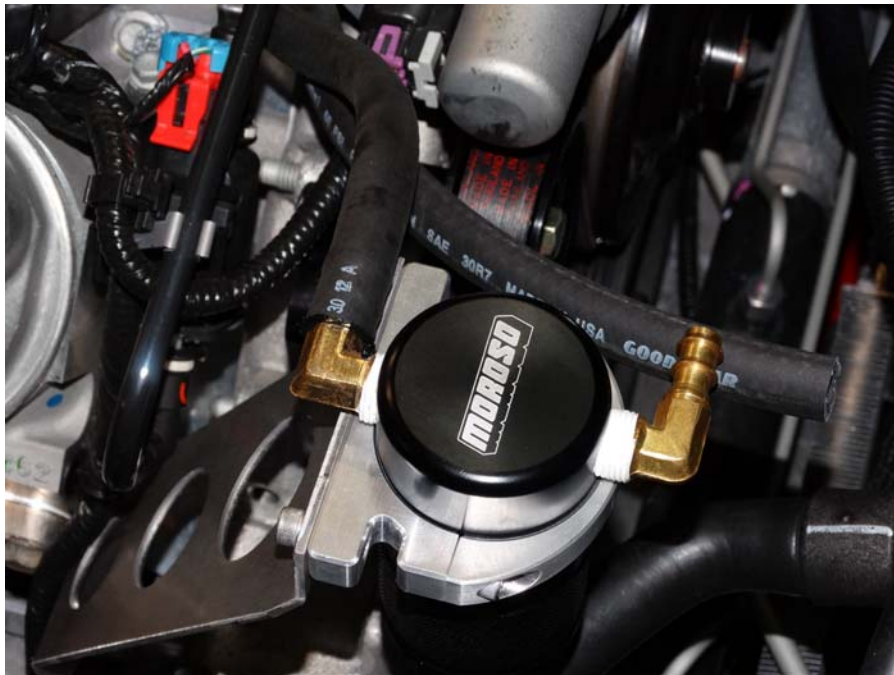
Step 12: Trim hose as needed and assemble to Air Oil Separator.
