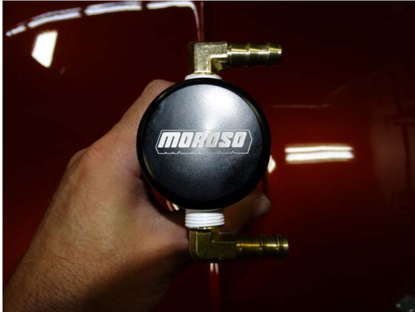
Step 9: Assemble Air Oil Separator as shown using Teflon tape on brass fittings.
