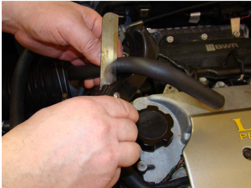
Step 19: Route line #2 to fitting as shown, mark and cut to correct length.
