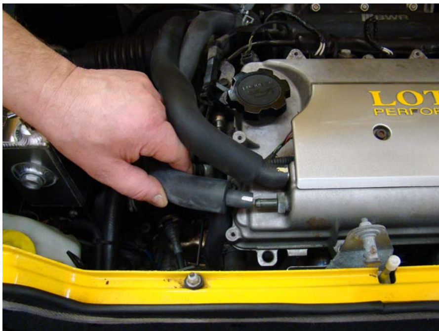
Step 1: Remove vacuum line shown and label as line #1.
