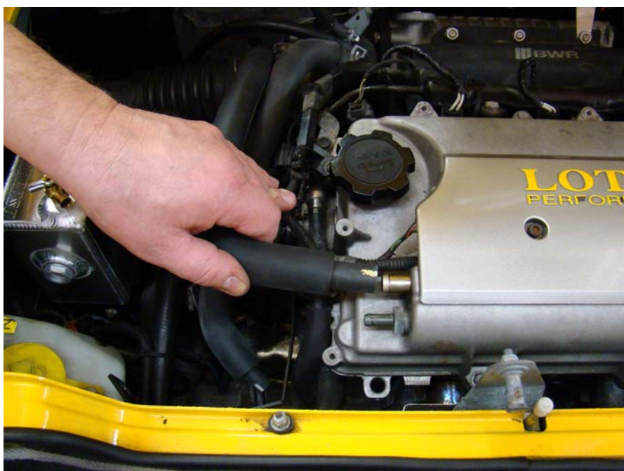
Step 2: Remove vacuum line shown and label as line #2.
