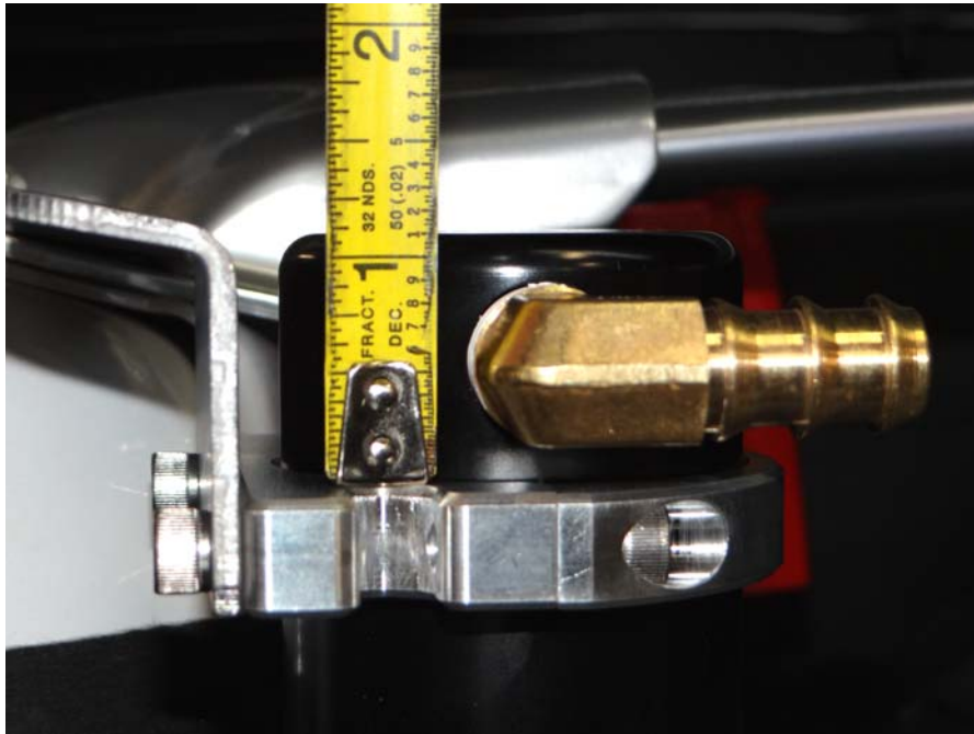
Step 17: Set height to approximately 1" and tighten clamp.
