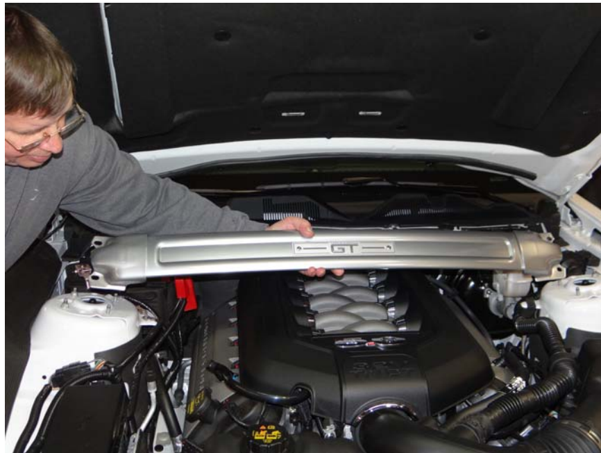
Step 1: Remove strut tower brace.
