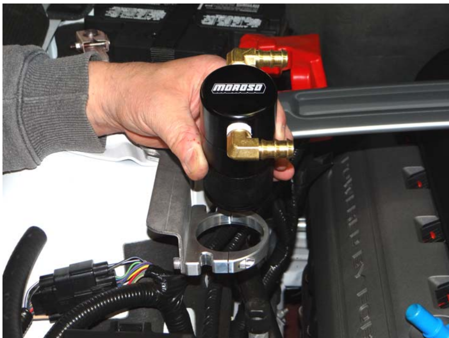
Step 15: Insert Air Oil Separator into clamp assembly.
