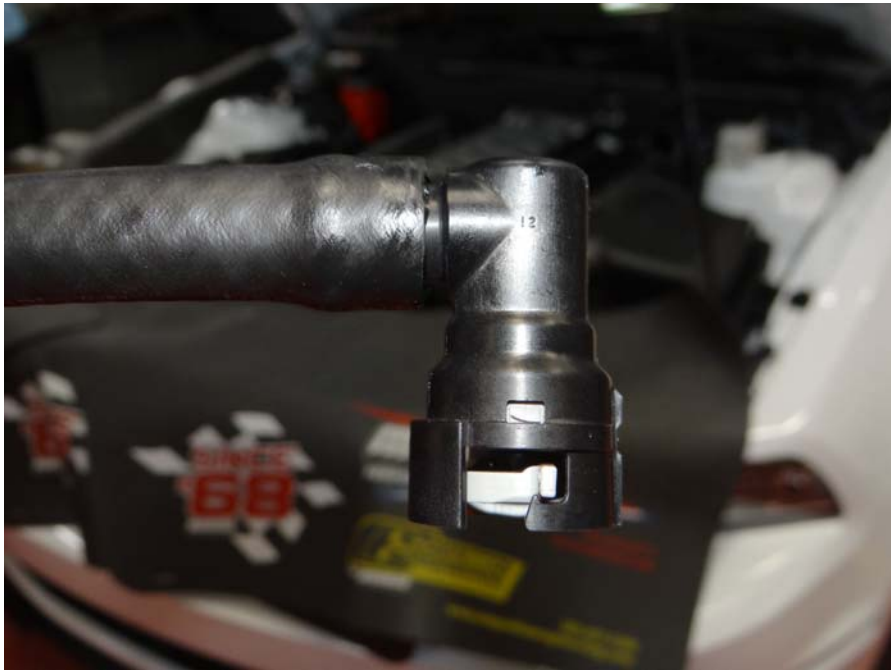
Step 7: Insert (1) 90 degree fitting into ½" hose.
