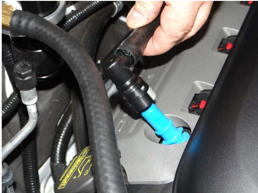
Step 21: Insert 90 degree fitting over valve cover nipple.
