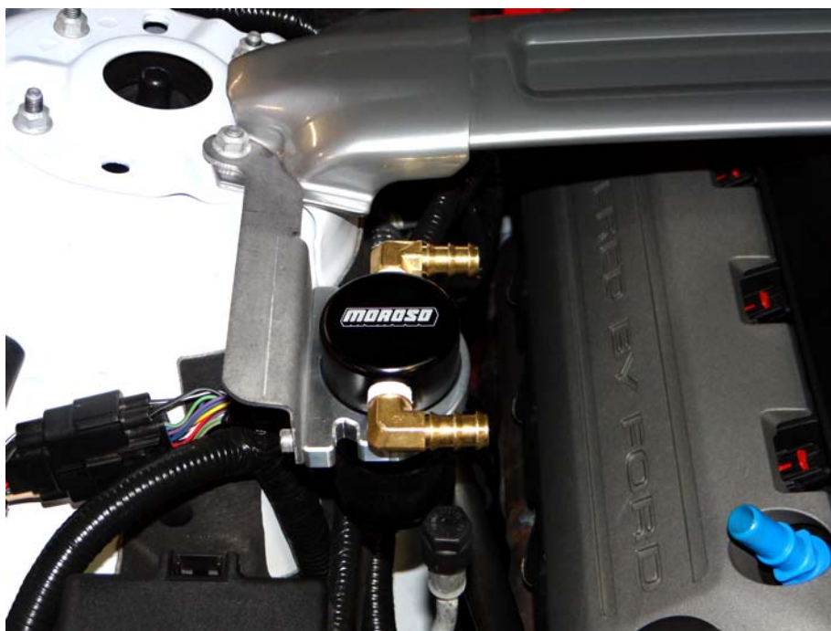
Step 16: Orientate fittings towards engine as shown.
