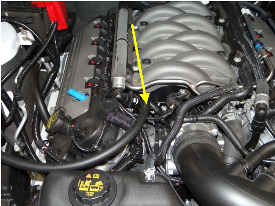
Step 8: Install 90 degree fitting to intake nipple.
