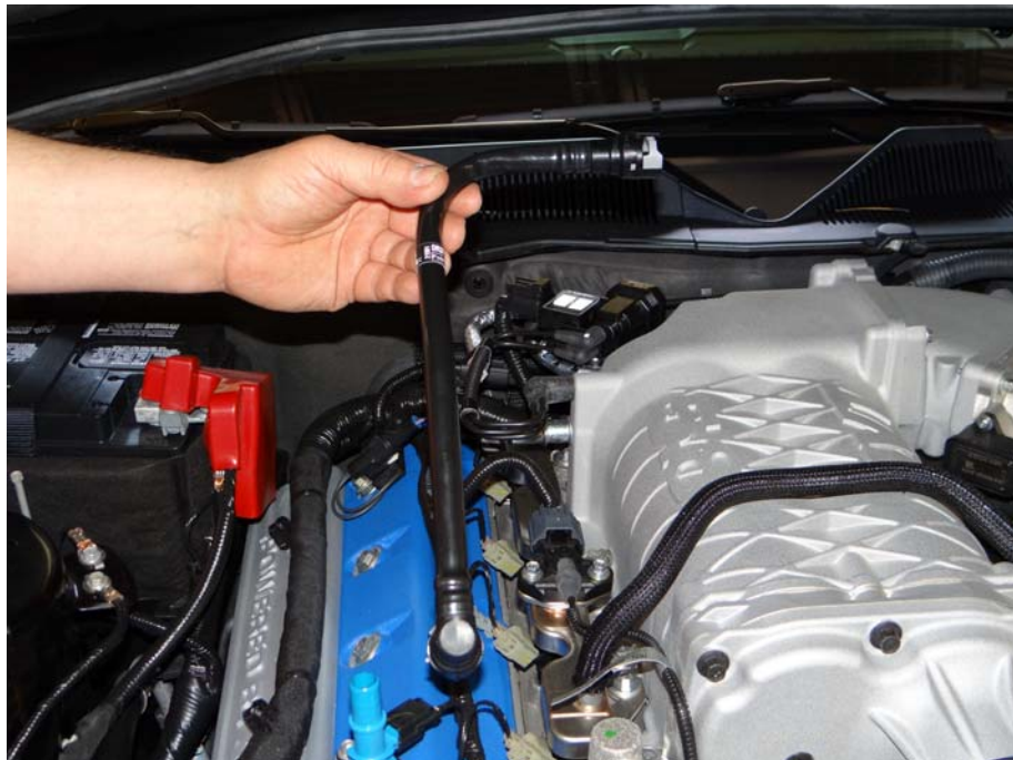
Step 4: Remove PCV line from vehicle.
