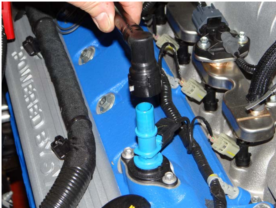
Step 2: Remove from valve cover.
