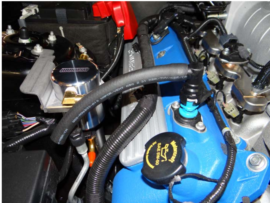
Step 14: Install 90 degree fitting to valve cover.
