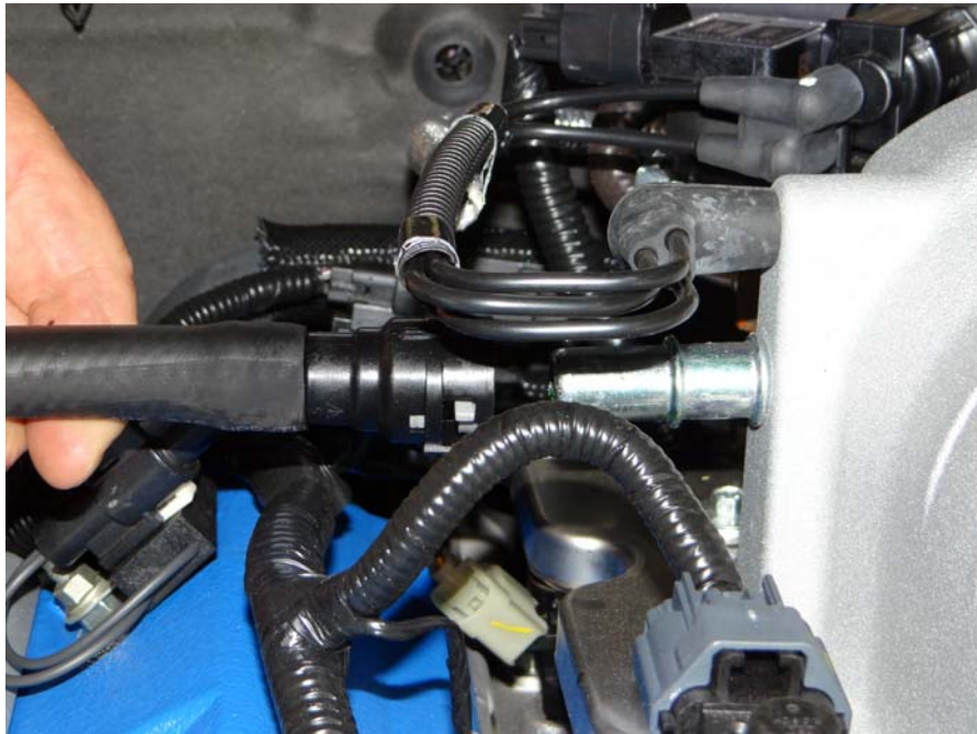
Step 13: Install straight fitting to intake.
