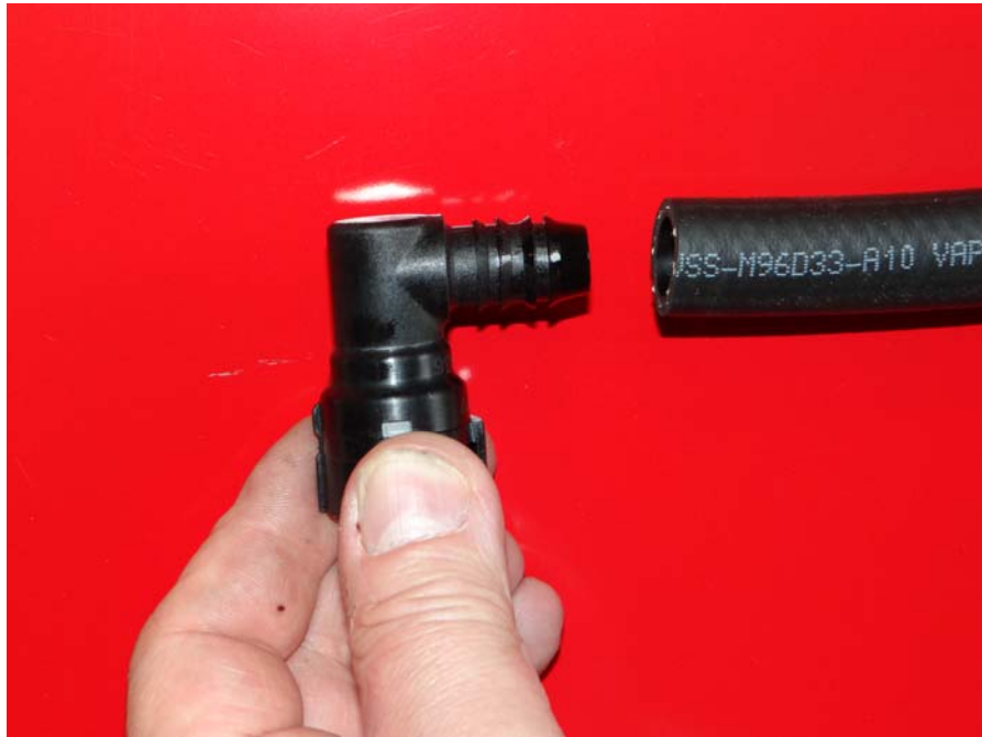
Step 11: Insert 90 degree fitting into 8" long ½" hose.
