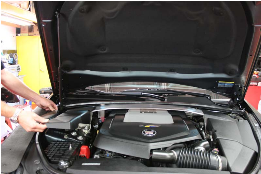
Step 1: Remove engine covers.
