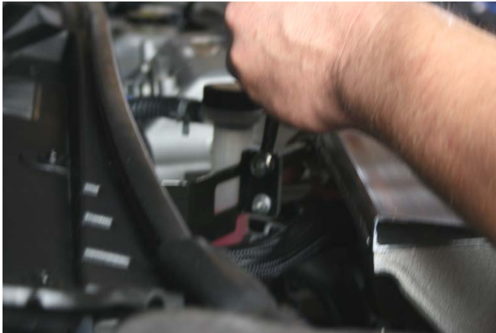
Step 3: Remove filler neck mount bolts.
