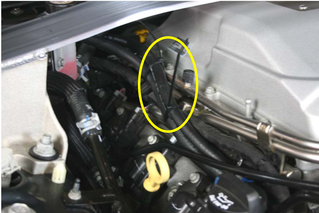
Step 19: Wire tie hoses as needed.
