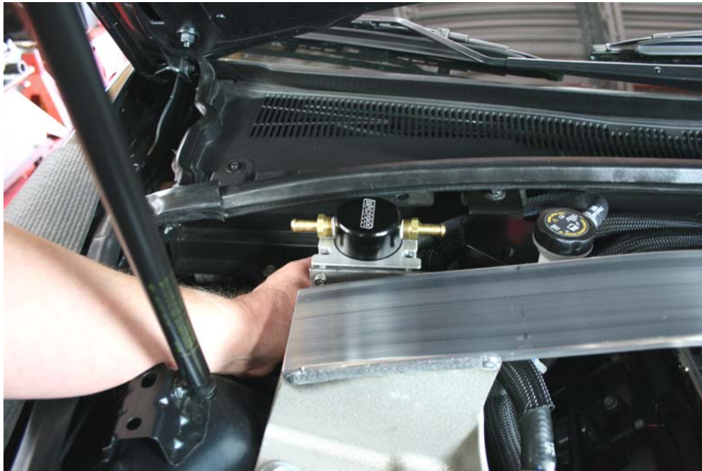
Step 9: Assemble Air Oil Separator to Stainless Bracket using (2) 1/4-20x5/8 SHCS.
