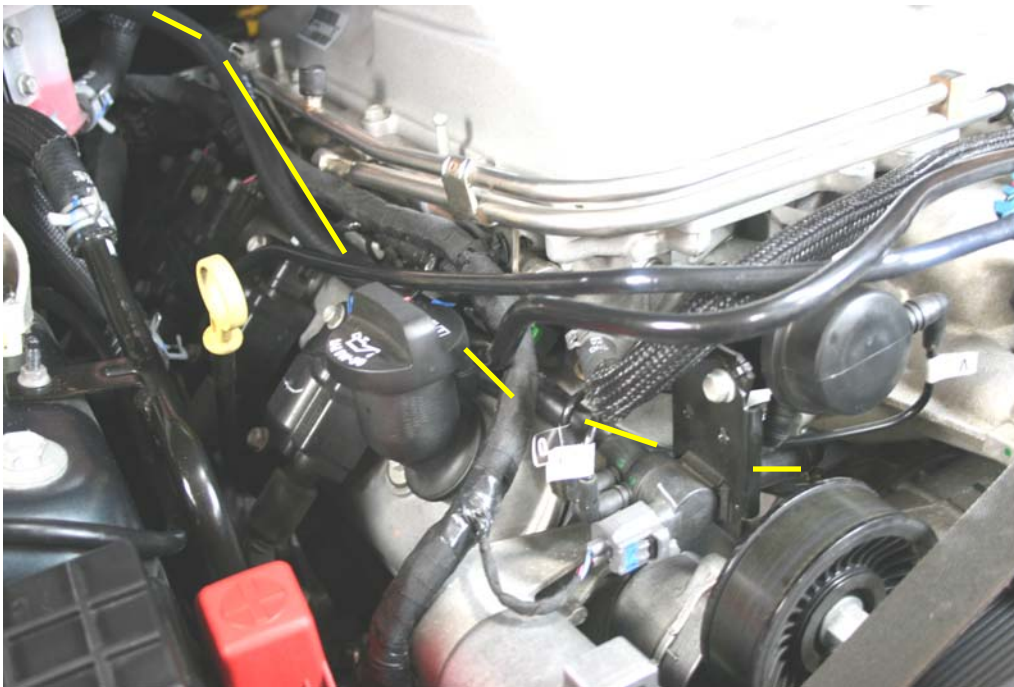
Step 14: Route hose from block valley to air oil separator.
