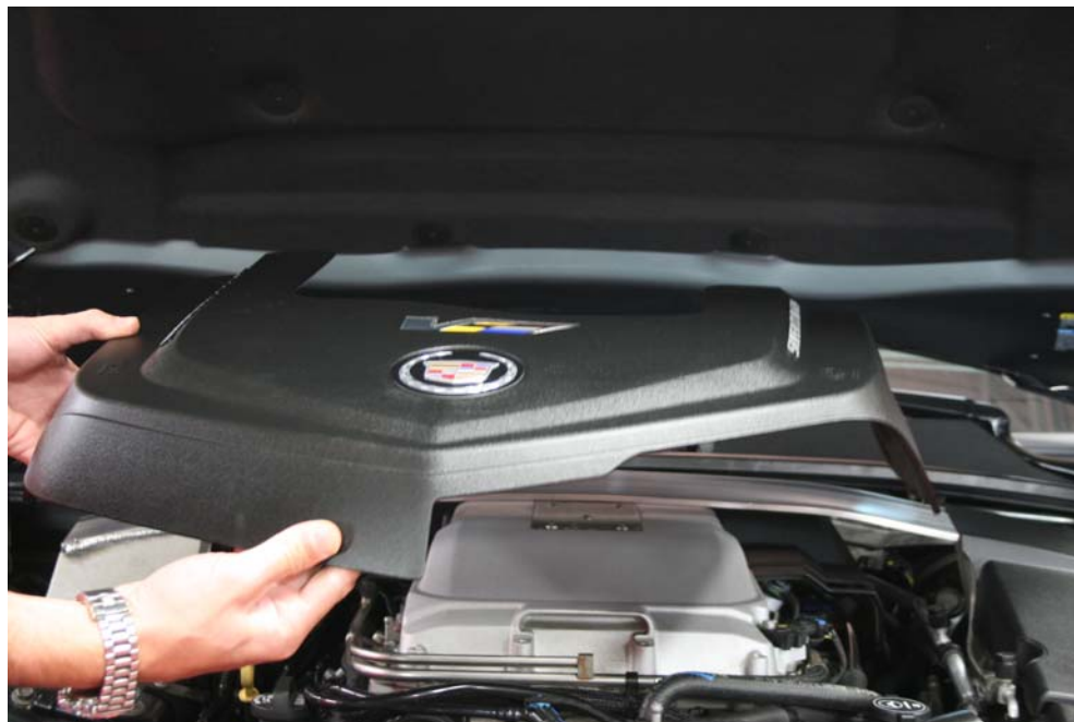
Step 1: Remove engine covers.
