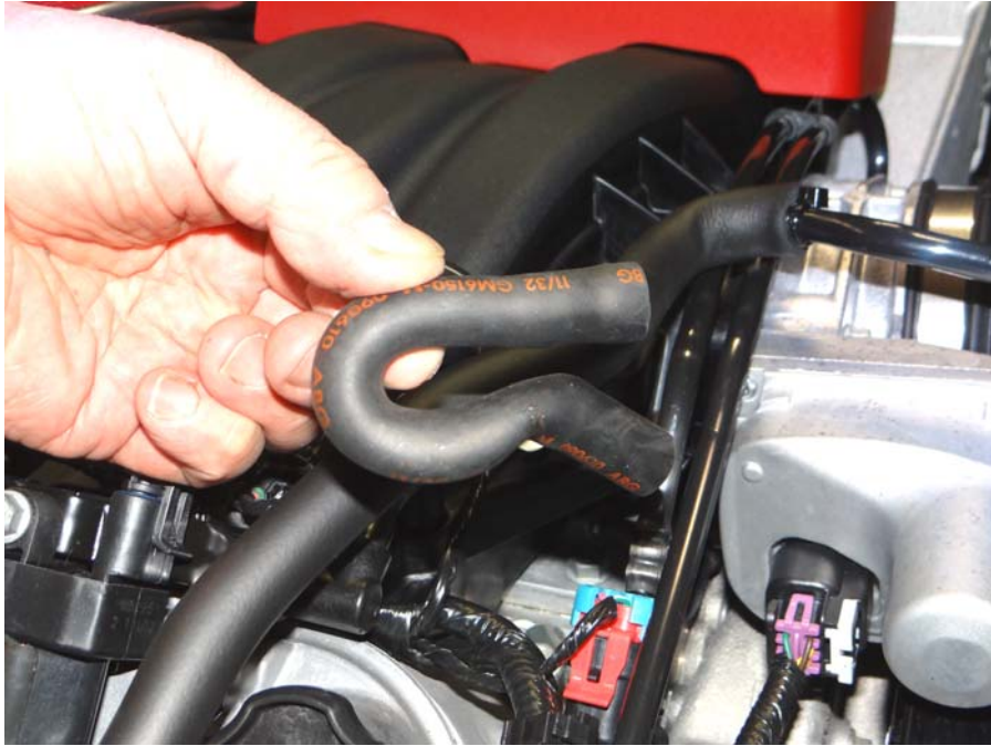
Step 3: Remove PCV line from vehicle.
