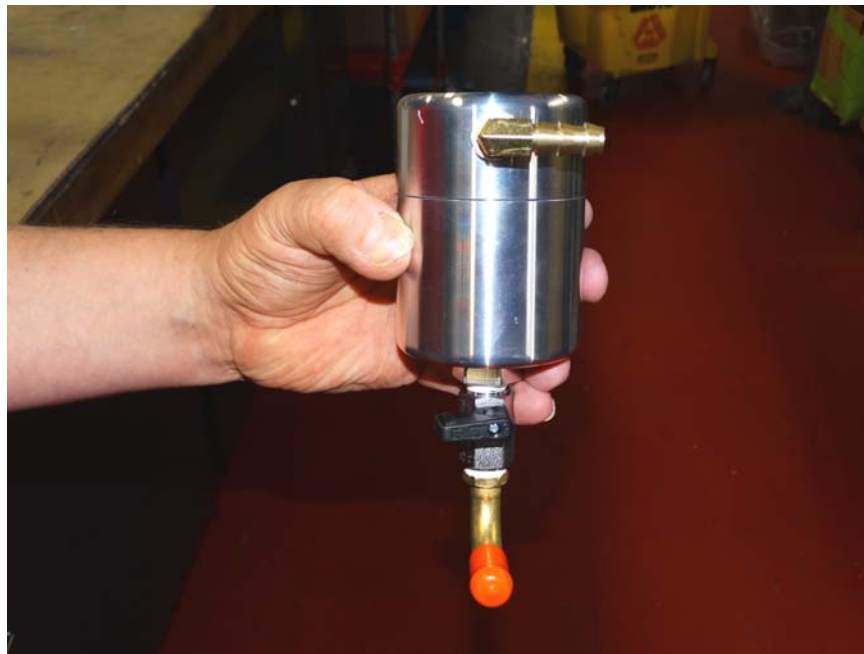
Step 9: Assemble air oil separator as shown using Teflon tape on all fittings.
