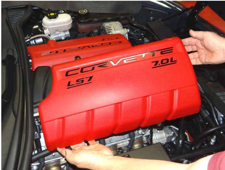
Step 1: Remove passengers side engine cover.
