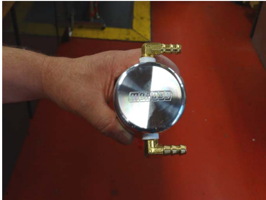
Step 9: Assemble air oil separator as shown using Teflon tape on all fittings.
