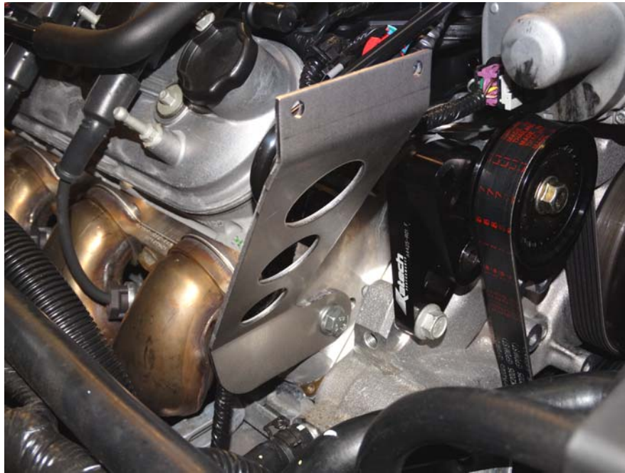
Step 7: Install stainless mounting bracket as shown.
