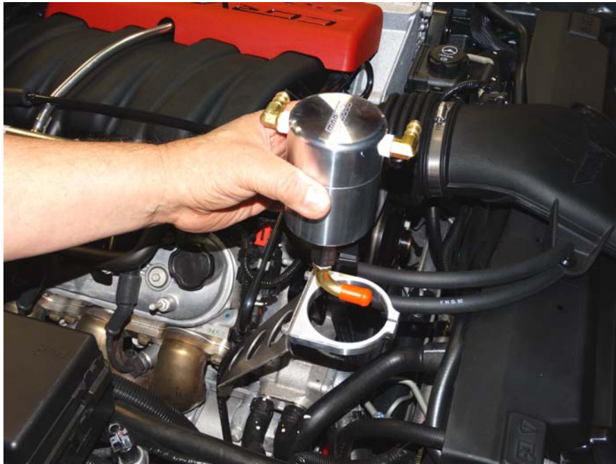
Step 10: Insert Air Oil Separator into billet clamp.
