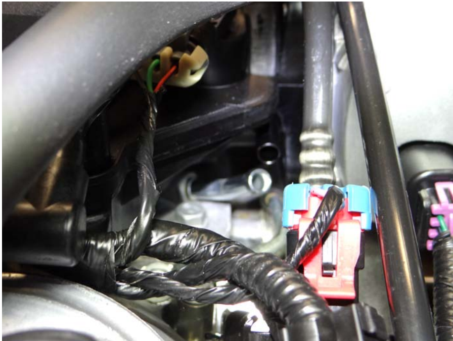
Step 3: Remove PCV line from vehicle.
