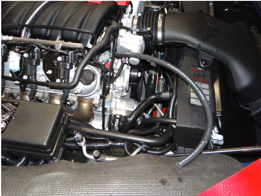
Step 4: Insert length of hose provided in kit to lifter valley nipple.
