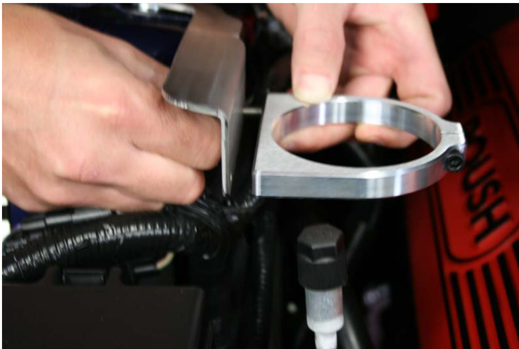
Step 17: Assemble billet clamp to stainless steel bracket using (2) ¼-20x5/8.
