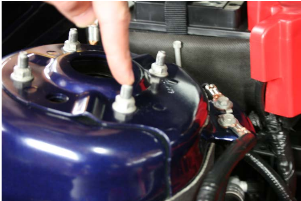
Step 12: Locate strut tower mount shown on passenger side.
