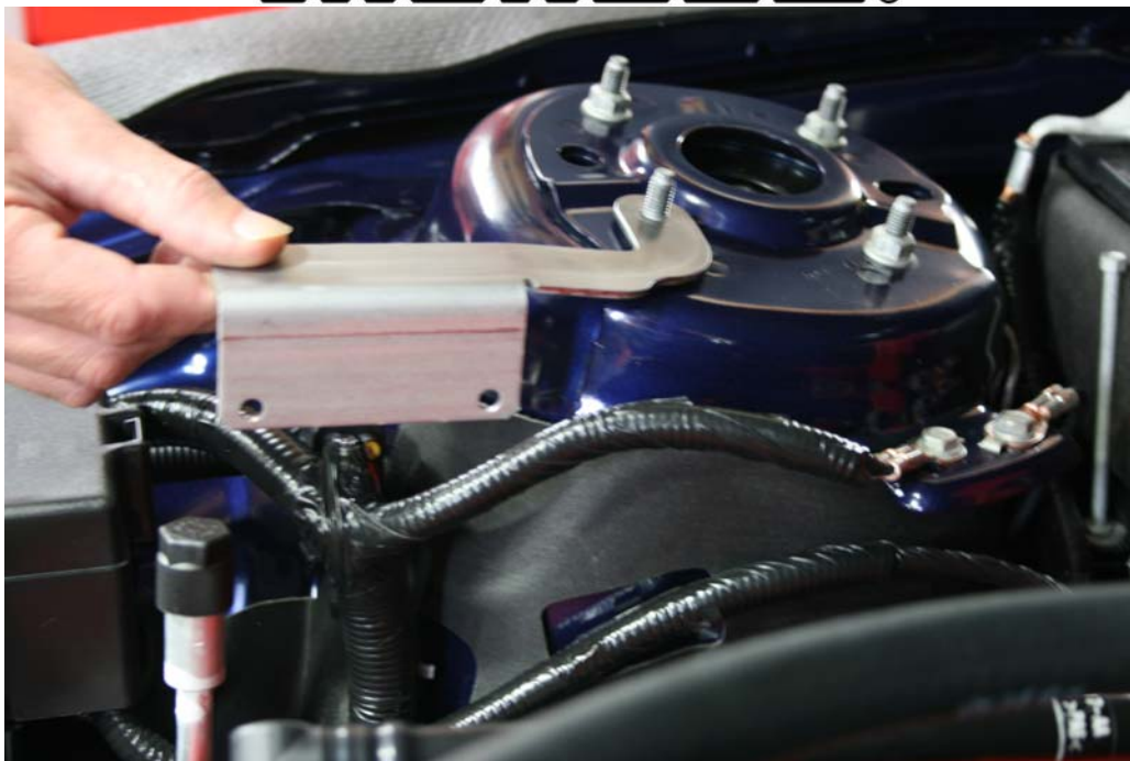
Step 14: Place stainless steel bracket over strut tower stud as shown.
