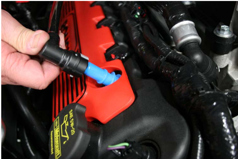
Step 8: Re-install valve cover fitting.
