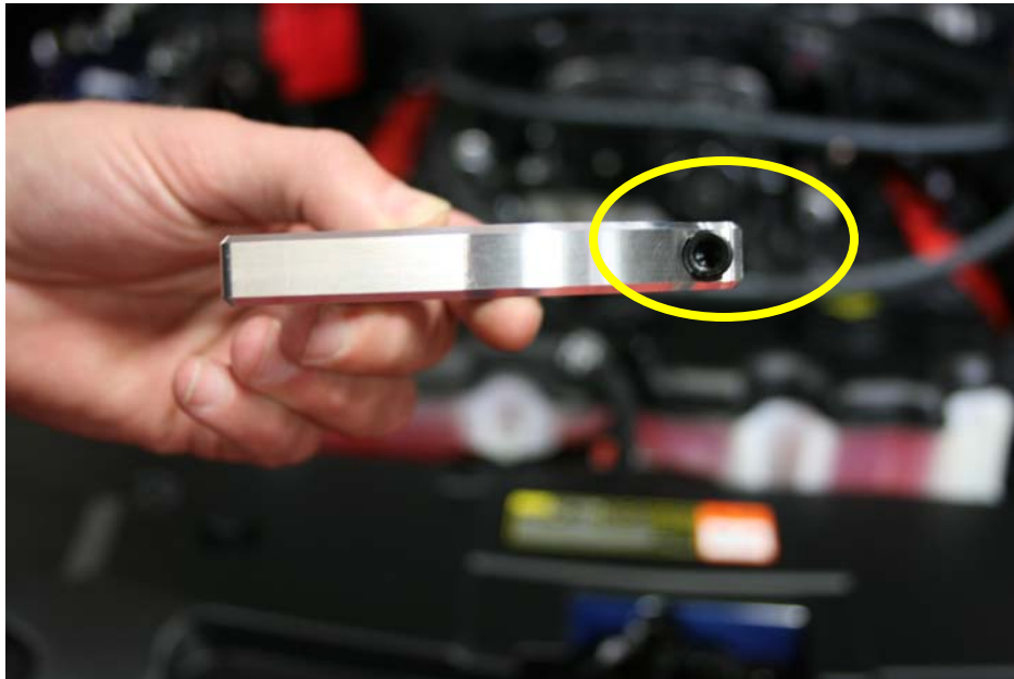
Step 16: Thread ¼-20x1 SHCS into billet clamp do not tighten.
