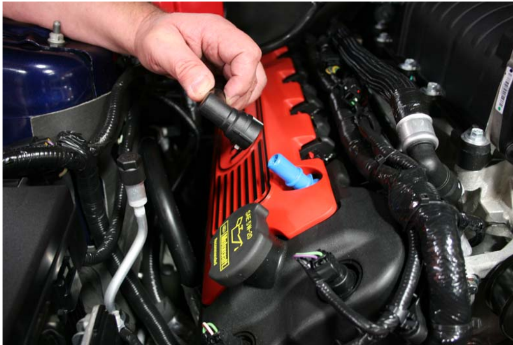
Step 3: Remove PCV line from valve cover.
