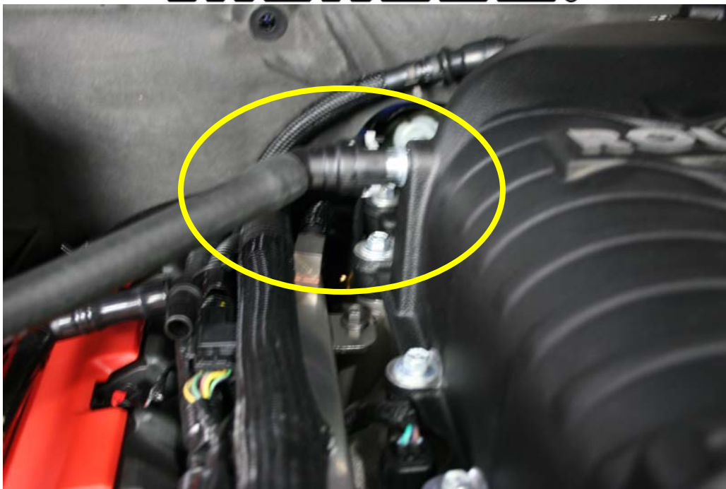
Step 10: Re-install 45 degree Super Charger fitting.
