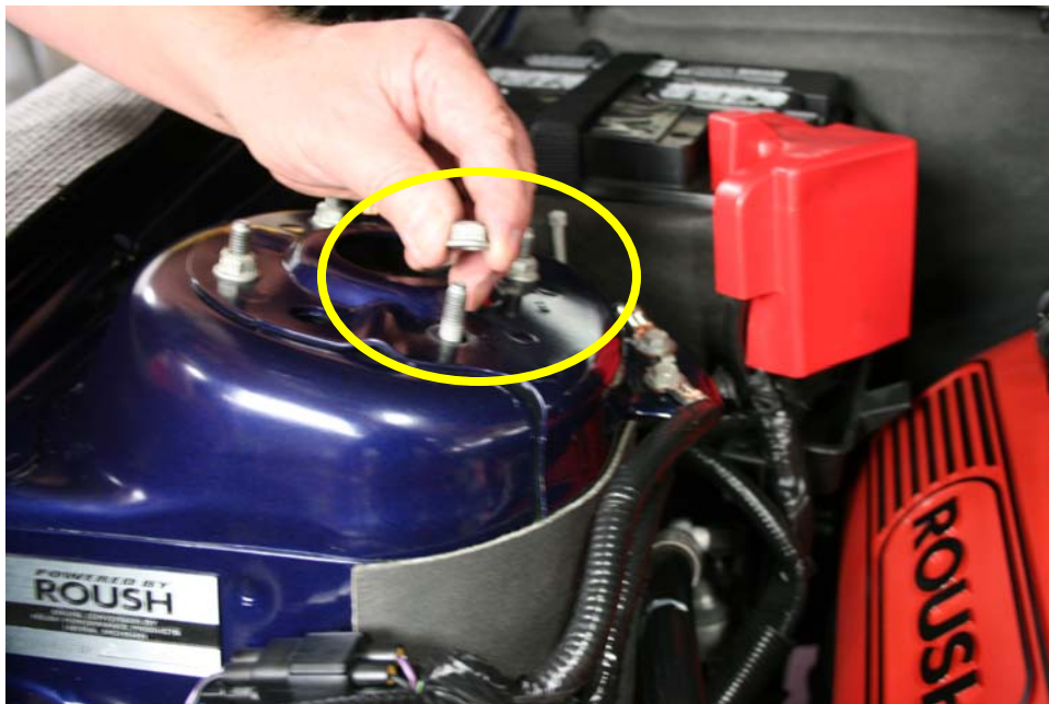
Step 13: Remove strut tower nut.
