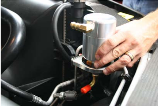
STEP 12 INSTALL AIR/OIL SEPARATOR INTO BILLET CLAMP
