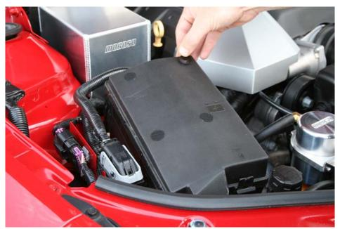
Step 2: Place Velcro hooks on top of Velcro loops previously installed
