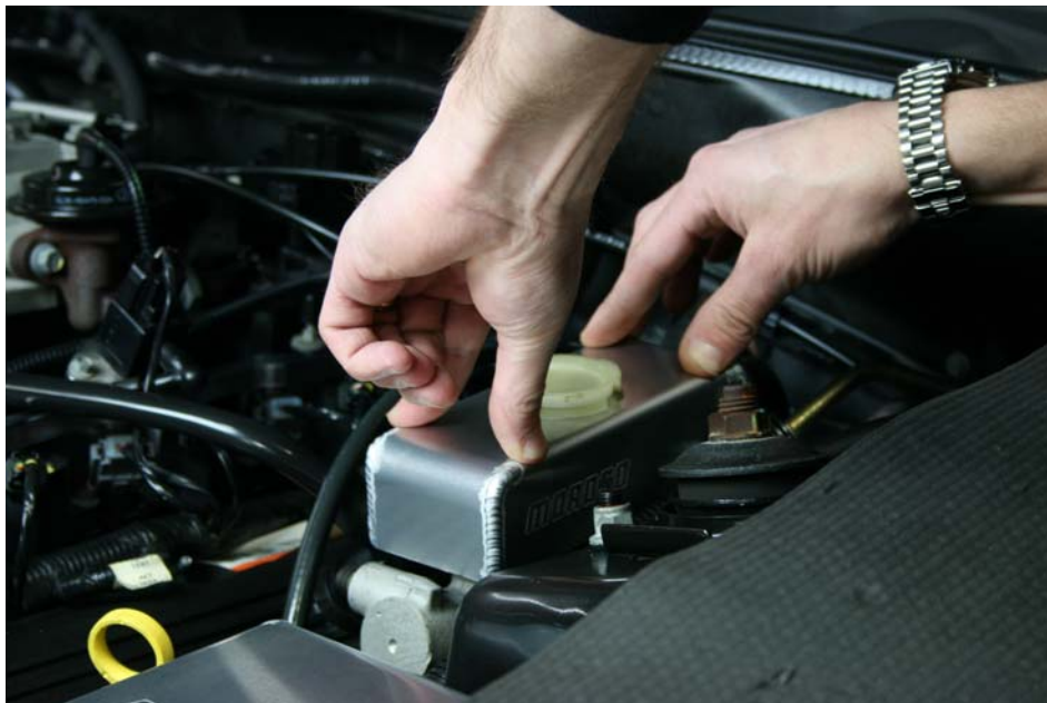
Step 4 Press firmly down on cover to secure Velcro dots to inside of cover
