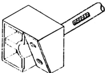
3. Insert the cut end of the wire into the back of the stripper.
