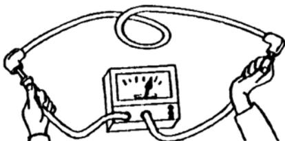
6. Check the wire's continuity with a test light or preferably an ohm meter. The meter should read approximately 800 ohms per foot of wire.
