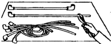
1. Determine the required wire length of each spark plug wire and choose the shortest wire that is long enough to reach. Cut the end of the wire to proper length with a side cutter or razor blade.
