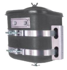
This cool can is designed and tested to have a maximum working pressure of 125 psi. The inlet/outlet ports on the Cool Can are -8AN for easy plumbing. The inlet and outlet ports are interchangeable, meaning the fuel can flow through the can in either direction.
