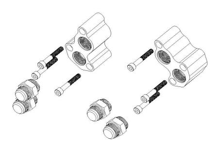
Moroso's 63616 water pump adapters can be used in any street, racing, or marine application where a remotely mounted water pump is used to cool an LS engine. Assemble the components of the kit as shown in the illustration above. RTV silicone or GM factory water pump gaskets can be used between the adapters and the engine block. Use –12AN hose to plumb your system. Below is a list of Moroso parts that can be combined to make a custom installation.
