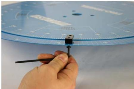
1-Attach the aluminum stands to the holes provided in the outer wheel. Insert the 10-32 screws into the deeper threaded hole while maintaining the flat side of the stand upward.
