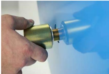
3- Take your Moroso Crankshaft Socket Hub (not included) and slide aluminum spacer provided over the threaded portion. Locate the Crankshaft Socket Hub through the back opening of the 20" degree wheel and the 18" degree wheel so the keyed hub is on the backside of the wheels. The 20" degree wheel will center up on the aluminum spacer, and the 18" wheel will center up on the threaded part of the hub.
