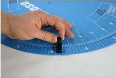
2- Place degree wheels on table as so markings are facing upward. The inner wheel will be held in place, but not centered yet by the four nylon set screws. Loosen the nylon thumbscrews so the outer wheel is free to turn.
