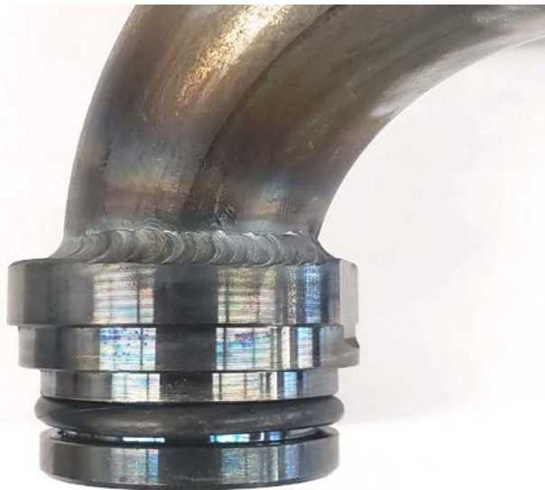
Step 6: Install the provided O-ring on the pickup and lubricate with engine oil before continuing.
