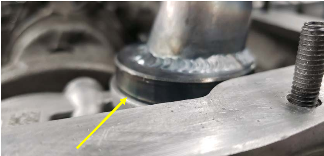
Step 8: Note: pickup must be fully seated in the oil pump.
