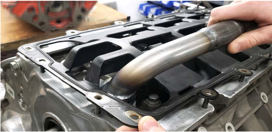
Step 7: Install the tray on the studs, and then lift the front of the tray while simultaneously inserting the pickup into the pump.
