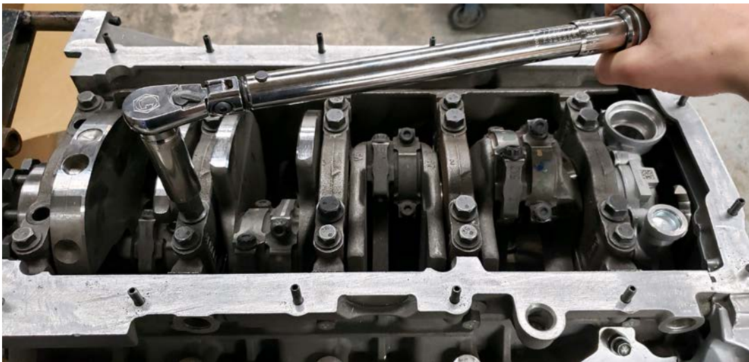
Step 5: Torque the standoff to 20 ft.-lbs.
