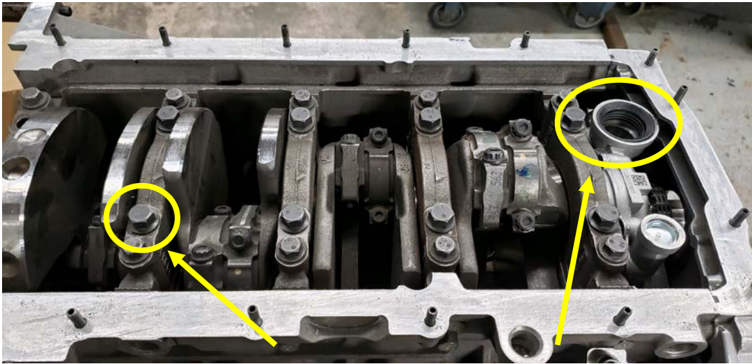
Step 1: Remove the highlighted main cap bolt, and O-ring from the pump.
