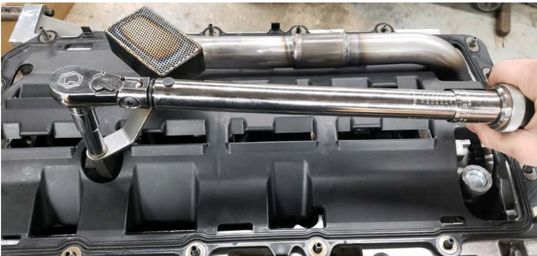
Step 9: Fasten the pickup bracket to the standoff using the provided 8mm flange head screw. Torque to 20 ft.-lbs.
