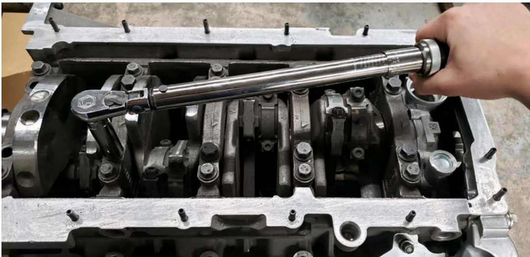
Step 3: Tighten the main cap bolt to factory specifications.
