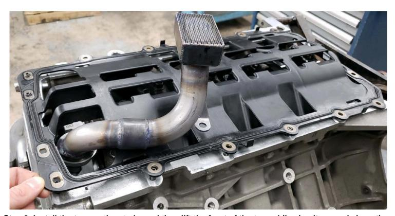
Step 6: Install the tray on the studs, and then lift the front of the tray while simultaneously inserting the pickup into the pump.
