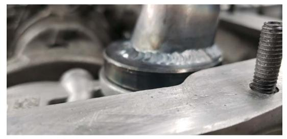
Step 7: Note: pickup must be fully seated in the oil pump.
