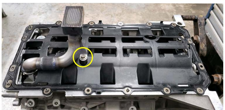
Step 8: Fasten the pickup bracket to the standoff using the provided 8mm flange head screw. Torque to 20 ft.-lbs.
