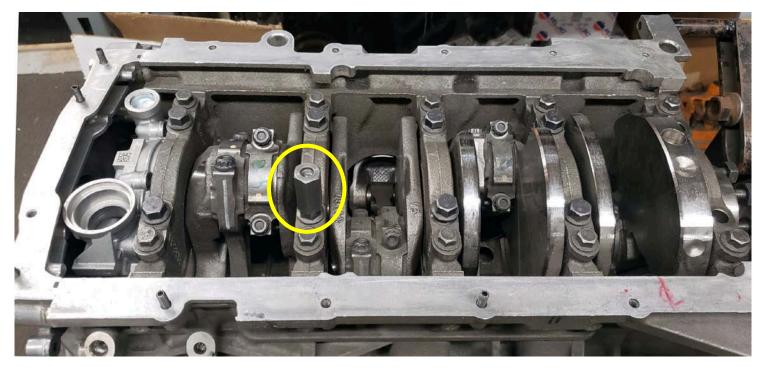
Step 4: Install and torque the standoff to 20 ft.-lbs.
