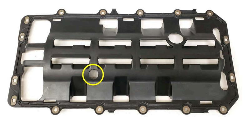
Step 2: Drill a hole in the scribed location using a 7/8" hole saw.
