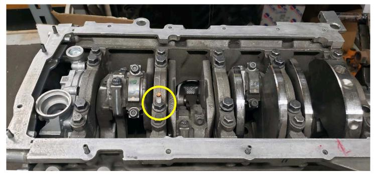
Step 3: Remove the factory main cap bolt and install the provided main cap bolt in the location shown above. Tighten the main cap bolt to factory specifications.
