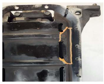
This photo shows a rough outline of where the rail is in-bound to the 16V tray. The orange line represents the basic area that needs to be removed.
