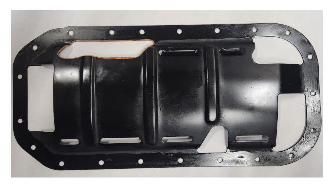
After clearancing, test fit the tray with the oil pan on the block. Proceed to deburr and clean the tray thoroughly. It is not recommended to clearance the oil pan rail as it could cause the rail to deform and no longer be flat.
