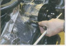
Next, the two holes are tapped to accept a 10x1.5mm bolt.
