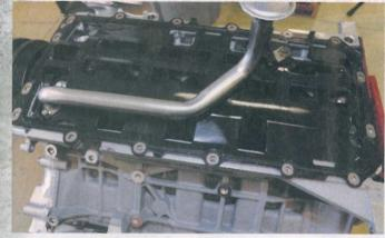
Interestingly, Ford decided to meld the oil pan gasket and windage tray into one unit. At around \$70, a replacement is a bit pricey, but the gasket is reusable. Since this engine has never been run and has never seen any heat cycles, we felt confident bolting the new oil pan right to the gasket.
