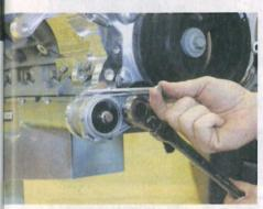
Vintage Air includes this belt tensioner. To keep it in the "loose" position so that the serpentine belt can be added later, pull it down using a 1/2-inch drive wrench in the square hole in the body of the tensioner. Then, a long 1/4-inch bolt can be used to hold the tensioner in position.
