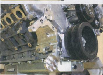
All the brackets are high-strength billet aluminum. This is the main bracket that locates the A/C and power-steering pumps as well as
