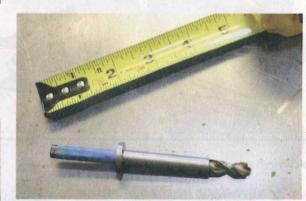
Two bosses on the front cover must be drilled and tapped. Vintage Air provides this sleeve guide and recommends using a Q-size drill bit (We used a 21/64 bit, since that's closest to the 8.433mm Q size.). The hole should be 1-inch deep, so the tape marks the point where the bit extends 1 inch past the sleeve guide.
