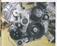
Both the power-steering pump and the A/C compressor are bolted up at this point. To make the alignment work, the power-steering pump is mounted up "backward" with the pulley facing toward the engine. All the mounting hardware provided by Vintage Air is high-quality 12-point
