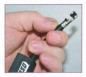
With the completed crimp shown. a quick glance at the insulation shows it to be squeezed tight, evidence of a proper crimp.
