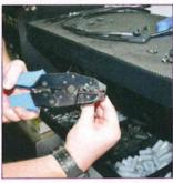
**Using Moroso's Super Duty Wire** Crimping tool complete with the correct jaw set for ignition wire terminals, the terminal end is finish crimped tight in place. Jaw sets are also available to be interchanged and used for standard primary wire terminals and perform the best tight crimp very similar to expensive factory crimp machines.
