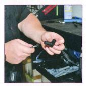
Using a small shot of WD-40 or dielectric grease inside the rubber boot, the crimped terminal and wire can be pushed into the boot.
