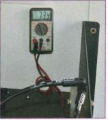
Not always necessary but checking each wire with an ohmmeter ensures that the connection is good. Moroso's Ultra 40 wire means each wire carries an ohmmeter reading of 40-ohms per foot. This particular wire was just under two-foot long and hence a reading of 73.9 ohms.
