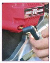
One last quick tip. When using MSD's popular HVC II Coil, due to the construction of the coil, a typical plug boot will not allow the wire terminal to fully seat. Hall's suggestion: "We cut back the boot slightly to allow the terminal end to fully engage the coil terminal."
