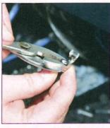
With the short portion of the wire bent over and a wire terminal install, pre-crimp the terminal to hold it in place.
