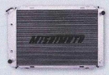
constructed using a lightweight two-row core made of 100-percent brazed aluminum and TIG welded polished end tanks. No cutting or additional modifications are required.
