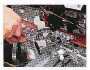
Setting the throttle stop rpm is a vital part of tuning your combination. With little time to test, we chose to fall back on Sunset's advice as to the setting as well as stop duration time. First run: An 8.92 at 185 mph in Super Comp trim proved they know what they're talking about.
