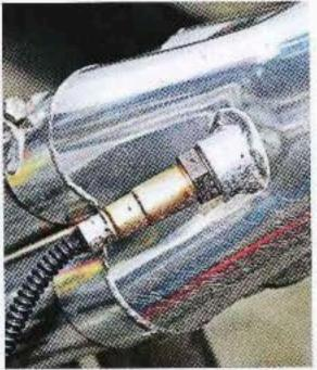
Using an Oxygen Sensor in our data logging system, we were able to notice the fuel system go extremely lean during the throttle stop period.
