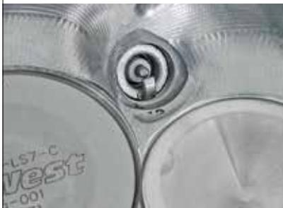
**This is the correct plug orientation according to most race engine builders. The side electrode gap faces up away from the piston dome, thereby achieving maximum clearance. If you run high-compression pistons and the gaps close up instead of widening as the plugs wear, index the plugs this way.**
