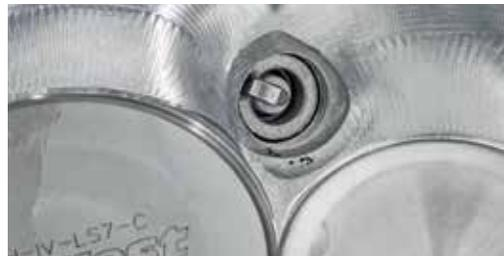
**Old-school thinking: The open end should face the hotter exhaust valve, making it easier to start the fire. This orientation also protects the plug from fuel wetting caused by a rich air/fuel charge. This isn't needed with modern chambers, ignition, and fuel management. On this Gen IV LS7 chamber, the plug is already biased toward the exhaust by design.**
