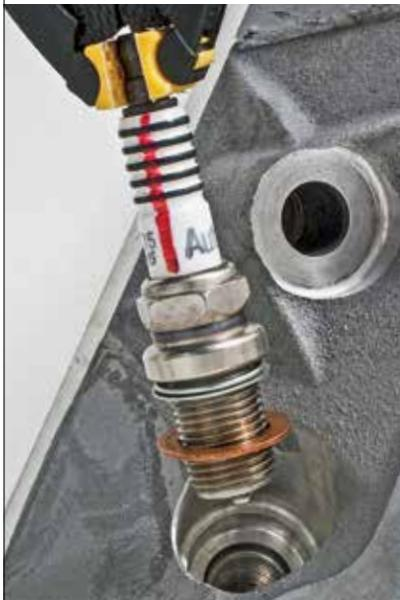
**Spark plug indexing may be needed to avoid side electrode contact with high-dome pistons. Moroso offers different thickness spark plug washer kits to accomplish this. Some theorists claim positioning the electrode in relation to the intake or exhaust valve may also be worth some power—at least on old-school chambers. To keep track of the electrode position, mark the plug's rear shell in line with the side electrode's open end.**
