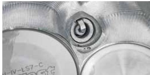
**Some ignition theorists claim that, for max power, the side electrode's open end should point down toward the squish area away from the path of maximum entrance turbulence. The squish air is said to be thrown right into the open, unhindered spark. Some even ricochets back off the side electrode and bounces into the spark again.**
