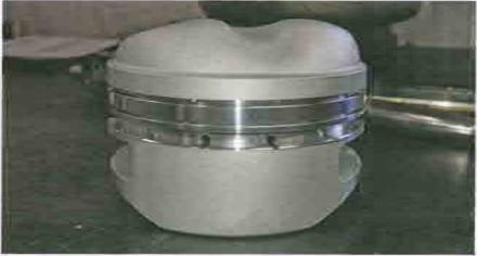
Before the Diamond pistons and rods are assembled, the pistons are bead blasted to "reflect the heat around all the edges," according to Bacalis.
