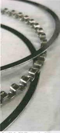
BES selected a custom Total Seal ring package for this build. The top ring is an .043-inch thick TNT top ring that uses Total Seal's hybrid ductile iron technology designed for the rigors of a nitrous-oxide application. The second ring is a ductile iron Napier ring measuring .043-inch, and in between you'll find a 3-piece oil ring combination. End gap specs are a shop secret, but it's typical to open up the end gap more with a nitrous build over a naturally-aspirated build.
