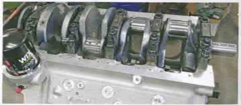
A Lunati Signature Series crankshaft with 4.5 inches of stroke is next to find a home in the block. A set of Clevite bearings (coated by Calico) are used with ARP studs and caps supplied by Brodix.
