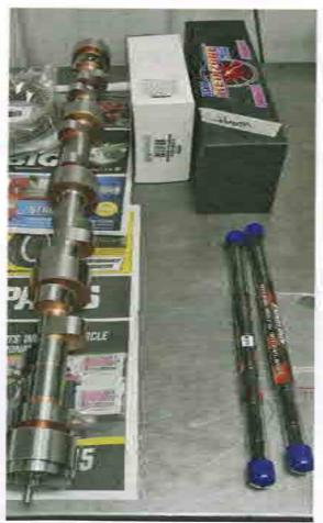
After the block is prepared, the first part to be installed is the camshaft. A Comp Cams solid roller was custom ground to BES specifications, and although we couldn't coax exact specifications from BES, "it has around an inch of lift," according to Johnson.
