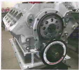
ATT's Super Damper takes its place on the front of the crankshaft. Bacalis noted BES has a good history with ATI, so it was a natural choice for this build.
