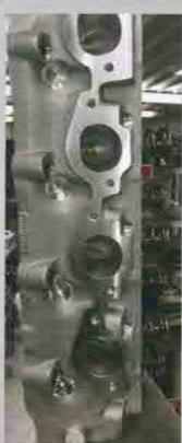
Breaking from a traditional build, Johnson selected a unique cylinder head from Brodix. "We've done some research and development with Brodix in the past," said Steve Johnson. "So they wanted to try this new cylinder head on the build. It is a crossover between a 68-3 XTRA and a Head. Hunter series, and features a smaller intake port than most builds of this nature." The heads were CNC finished by BME and BES softened the chambers.
