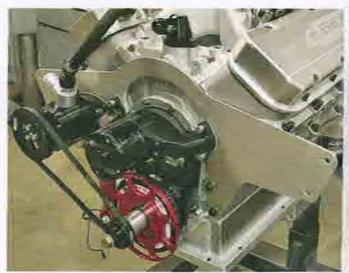
The final touches include bolting the carburetor and motor plate in place, as well as adding the MSD crank trigger, a Moroso vacuum pump and fittings, and a Meziere water pump.
