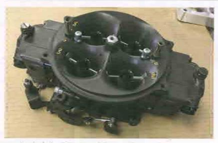
Metering the fuel and air mixture falls to a Holley 1250cfm Gen 3 Ultra Dominator carburetor. Featuring a refined main body and 20 percent larger capacity fuel bowls, the carburetor comes in at nearly four pounds lighter than previous Dominator models. Jon Bitler of IRD Racing Carburetors put his tweaks to it before it came to rest on top of the 588.
