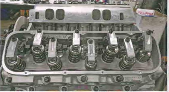
A T&D Machine Products shaft rocker assembly tops the cylinder heads with a 1.8:1 ratio working the Victory titanium intake valves and a 1.7:1 ratio addressing the exhaust side.
