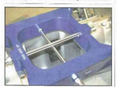
>> The NOS Crosshair plate is a modernization of the company's "Double Cross" design. Rated to flow 350-plus horsepower-worth of nitrous and fuel, we probably won't be THAT greedy on the dyno.
