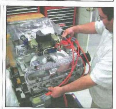
>> To get the spark from the distributor to the plugs, we went with MSD's 8.5mm Super Conductor wires. MSD offers them in pre-fit sets, meaning no building plug wires.
