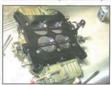
>> The 950 cfm rating is thanks in part to the 1-3/4-inch throttle blades. You can also see the billet aluminum base plate as well as the billet metering blocks peeking through.
