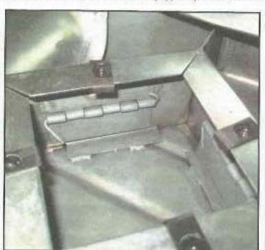
>>The internal baffling on the Moroso oil consists of these four "trap doors" along with another pair of baffles to keep the oil at the pickup even under hard acceleration and deceleration.
