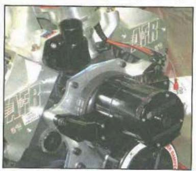
>> Not only does the 42 gph Meziere have a stout spec and capability sheet, but the parts really add to the aesthetics of the engine. Their pumps and water necks are available in a number of anodized colors.
