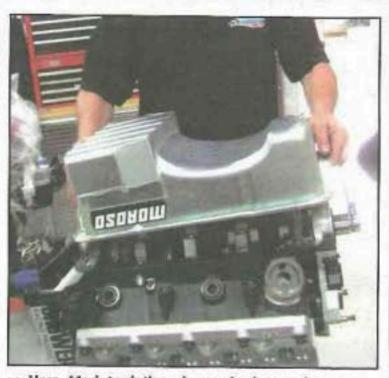
>> Here, Mark took the reins to check to make sure that there was enough clearance between the pickup and the pan. There was plenty, according to the modeling clay we used to check.
