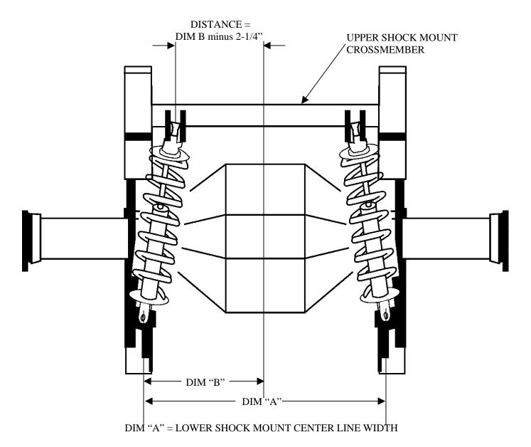
DIM "B" =  $\frac{\text{DIM "A"}}{2}$
