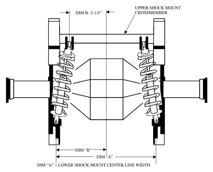
DIM "B" =  $\underline{\text{DIM "A"}}$
