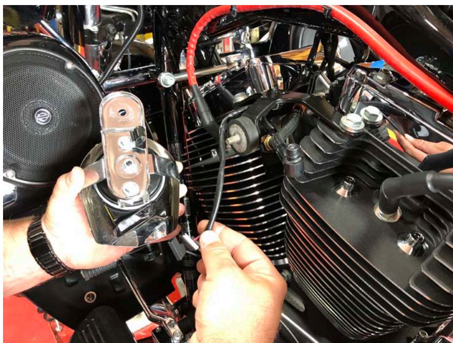
Step 27: Remove horn from motorcycle.
