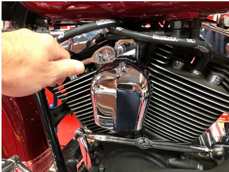
Step 8: Remove horn from motorcycle.
