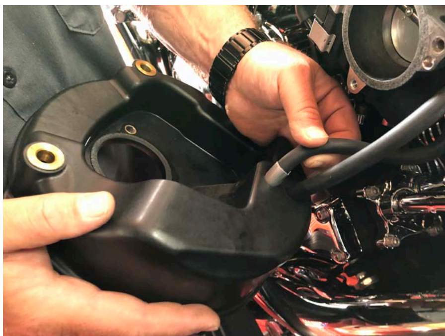
Step 15: Feed 2 nd line through top hole previously drilled in air pan.
