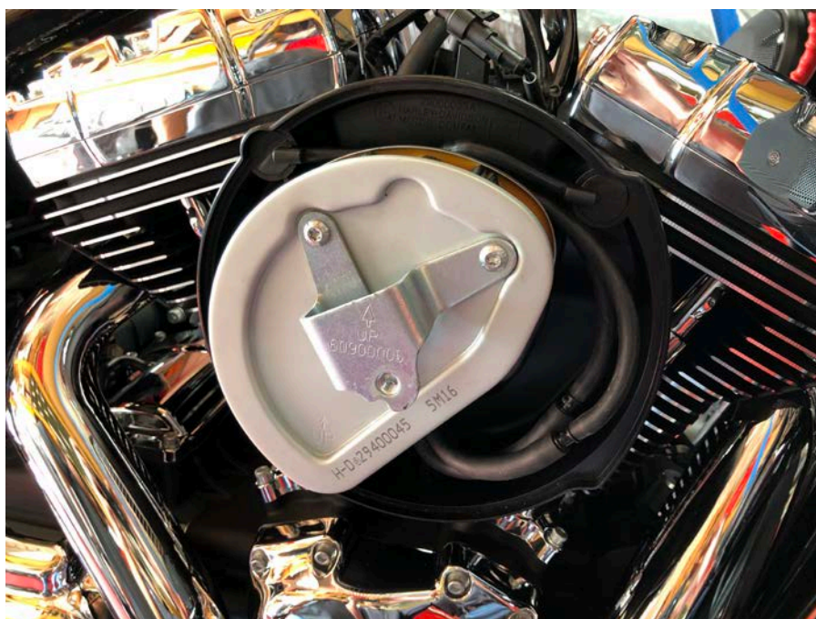
Step 25: Insert 90 degree end of return line into back of air filter and re-install air filter.
