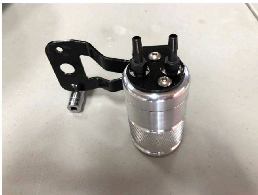
Step 29: Assemble Air Oil Separator to Air Oil Separator bracket using (2) \frac{1}{4} -20x \frac{1}{2} " button head bolts. Install (2) \frac{1}{4} " x \frac{1}{8} " NPT barbed fittings.
