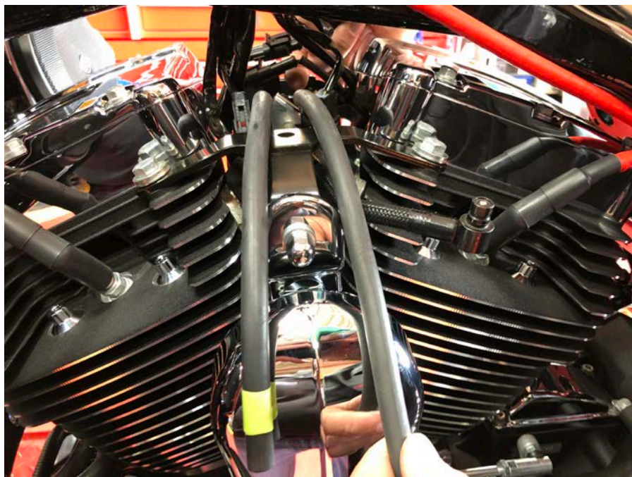
Step 11: Using ¼" I.D. line provided in kit cut (1) pc 28" long and route along side of first line installed.
