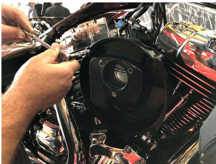
Step 3: Remove air pan.
