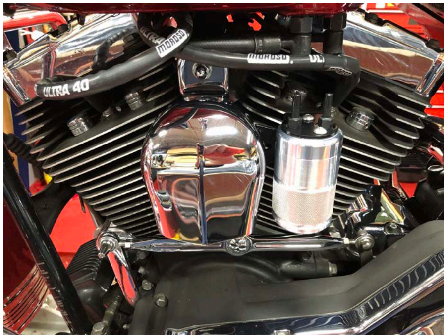
Step 13: Re-install horn / Air Oil Separator to motorcycle.
