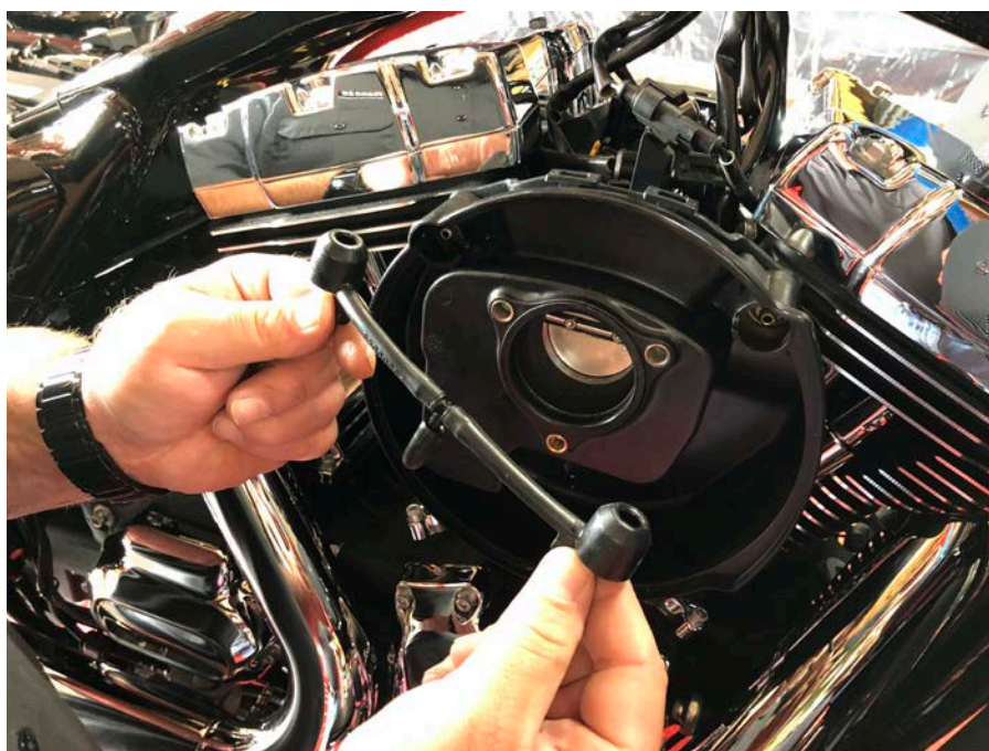
Step 2: Remove breather lines from breather bolts and air pan, set aside for future use.
