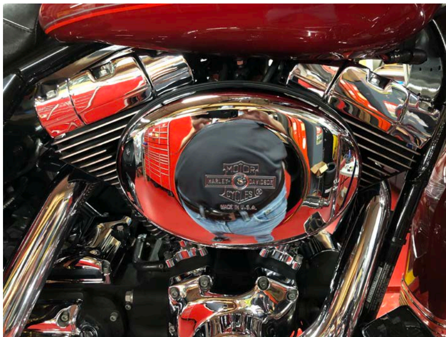
Step 28: Re-install air cleaner cover.
