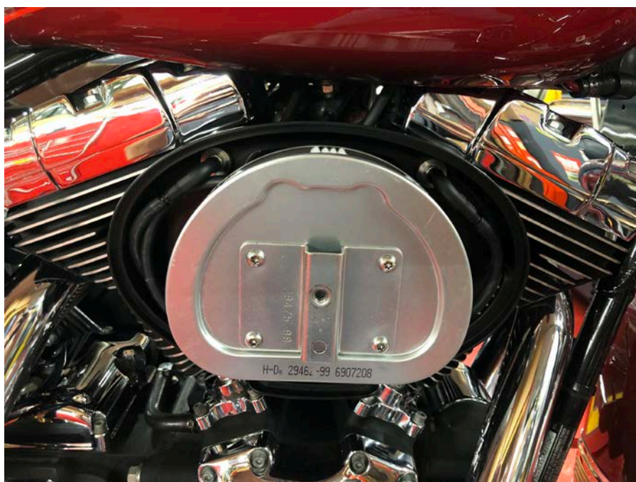
Step 27: Re-install air cleaner.
