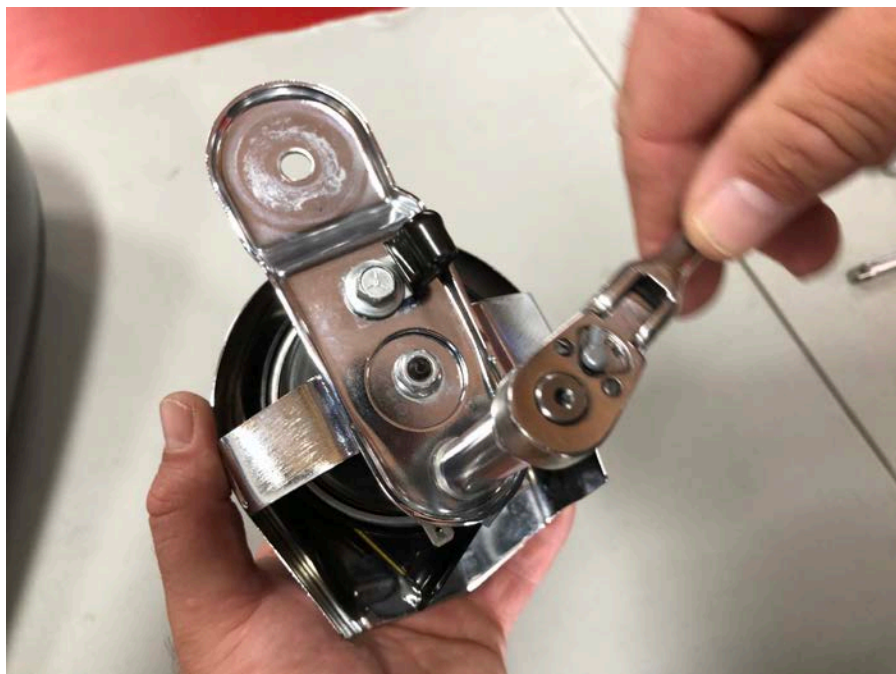
Step 28: Disassemble horn from horn bracket as shown.
