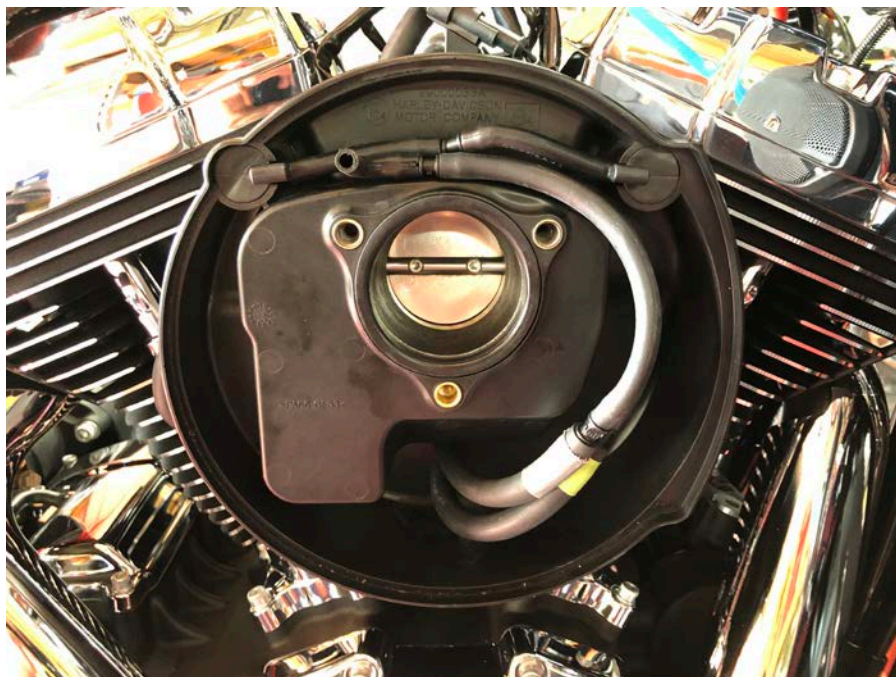
Step 24: Connect 6" line with 90 degree end to return line as shown.
