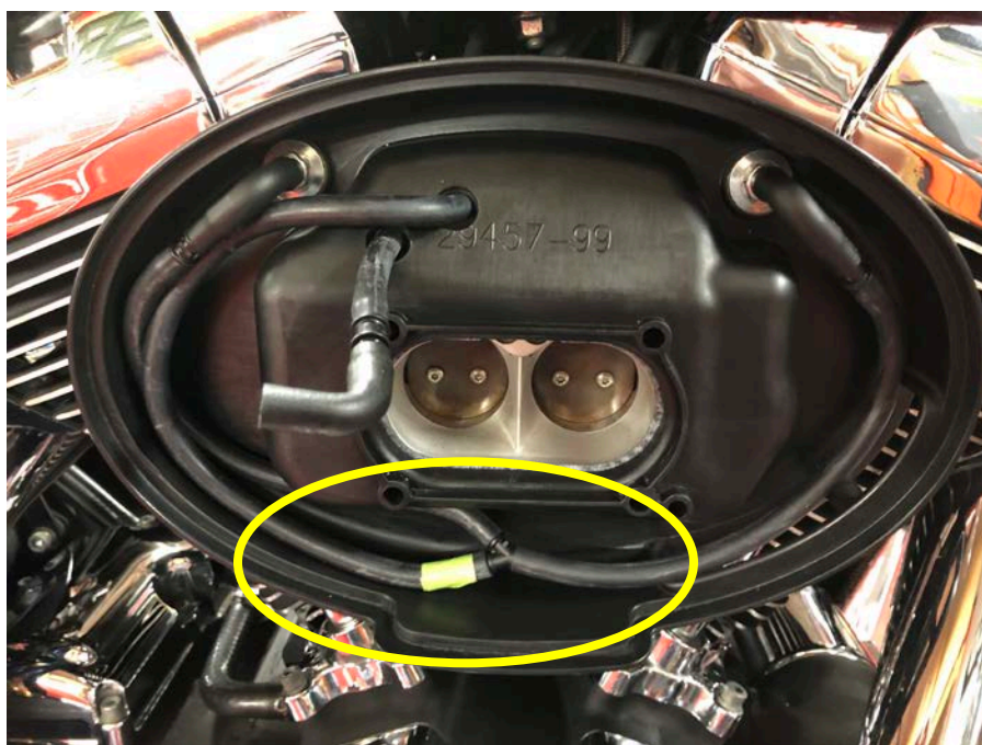
Step 24: Connect “Y” to breather line with masking tape identifier.
