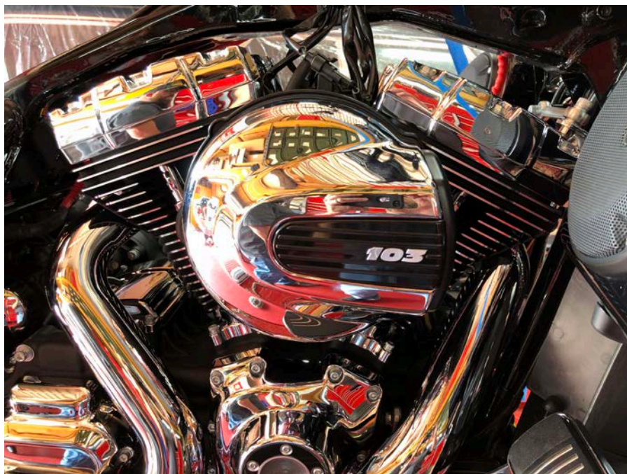
Step 26: Re-install air filter cover.
