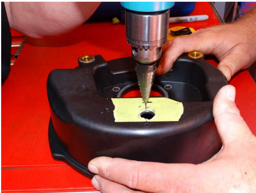
Step 7: Drill (2) ½" holes on center lines previously marked.
