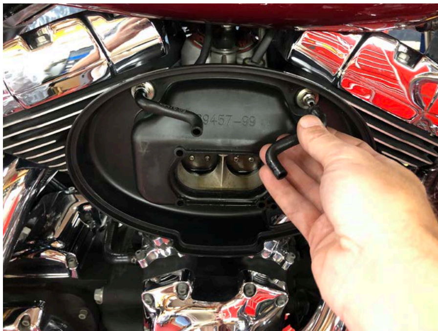
Step 2: Remove stock breather lines
