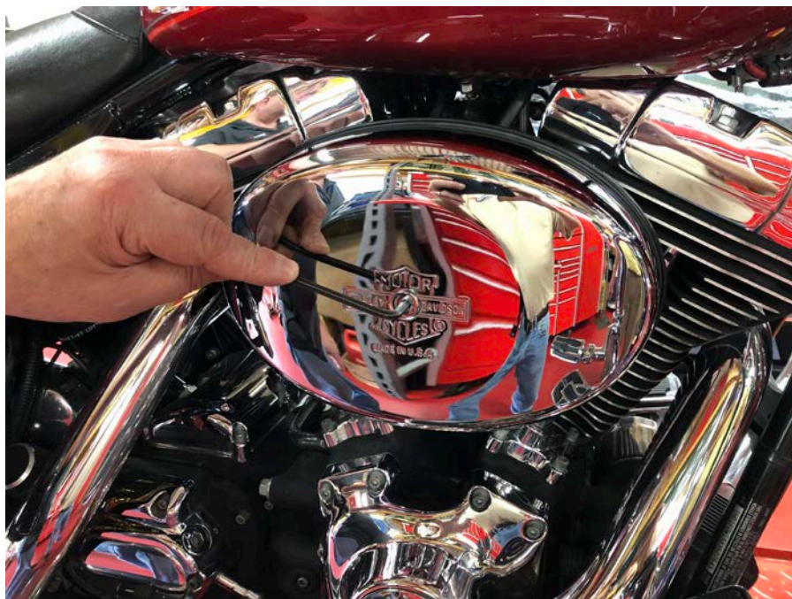
Step 1: Remove air filter cover and air filter.
