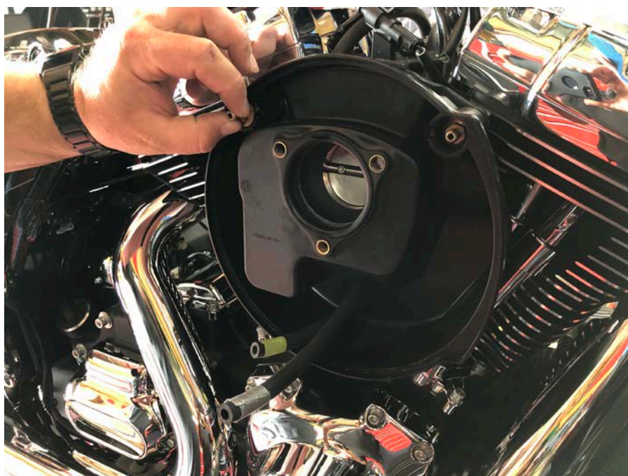
Step 16: Install head venting bolts do not tighten at this time.
