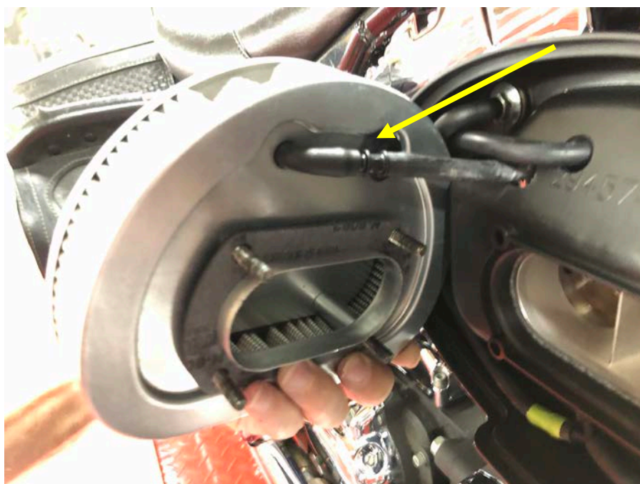
Step 26: Install 90 degree breather line into air cleaner.
