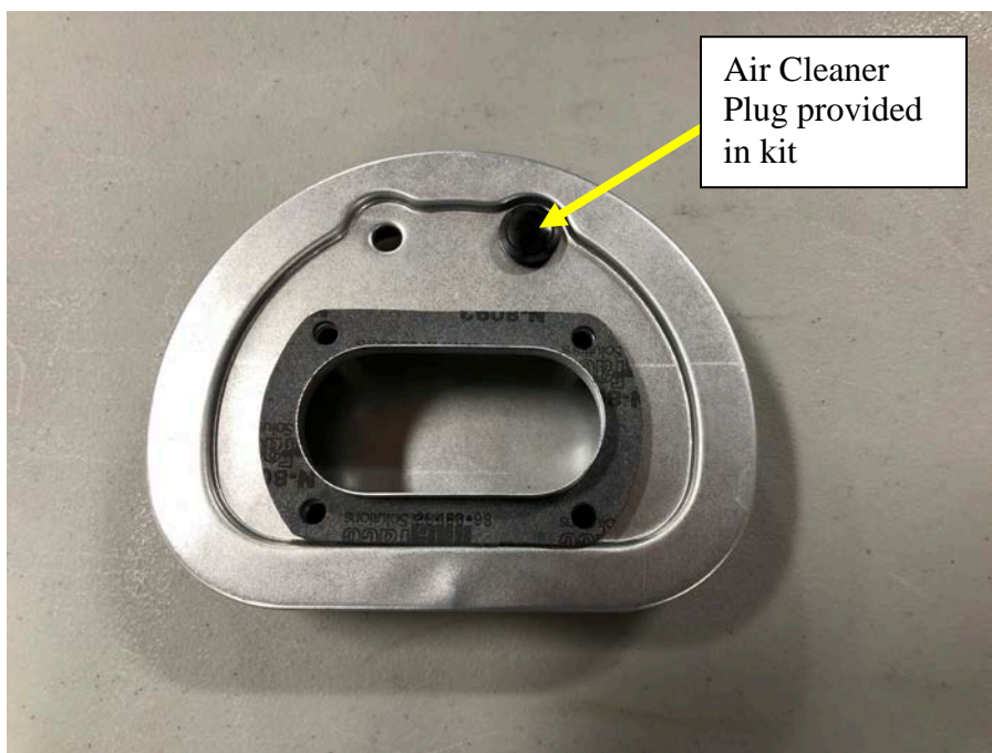
Step 25: Install plug into air cleaner as shown.
