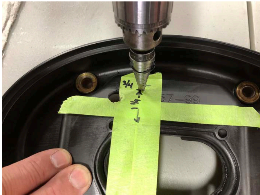
Step 7: Drill (2) 1/2" dia holes and deburr as needed.
