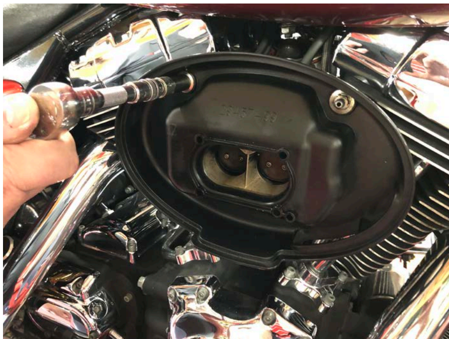
Step 3: Remove air pan.
