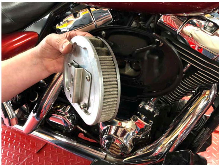
Step 1: Remove air filter cover and air filter.
