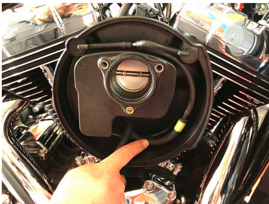
Step 23: Connect head breather line to breather line with masking tape identifier.
