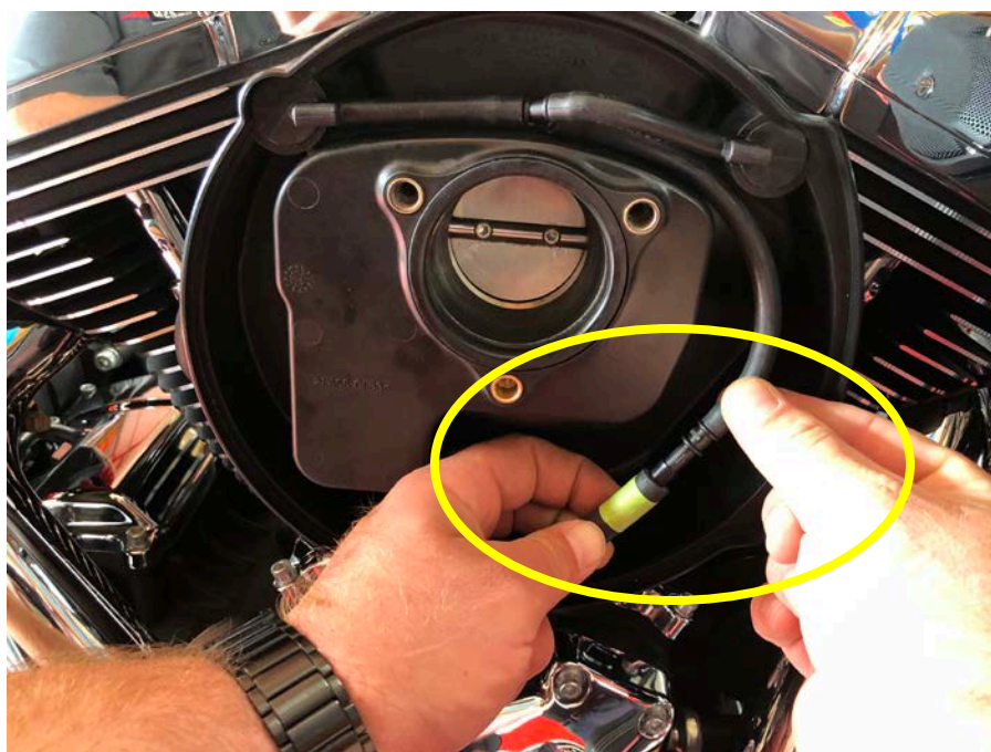
Step 23: Connect head breather line to breather line with masking tape identifier.
