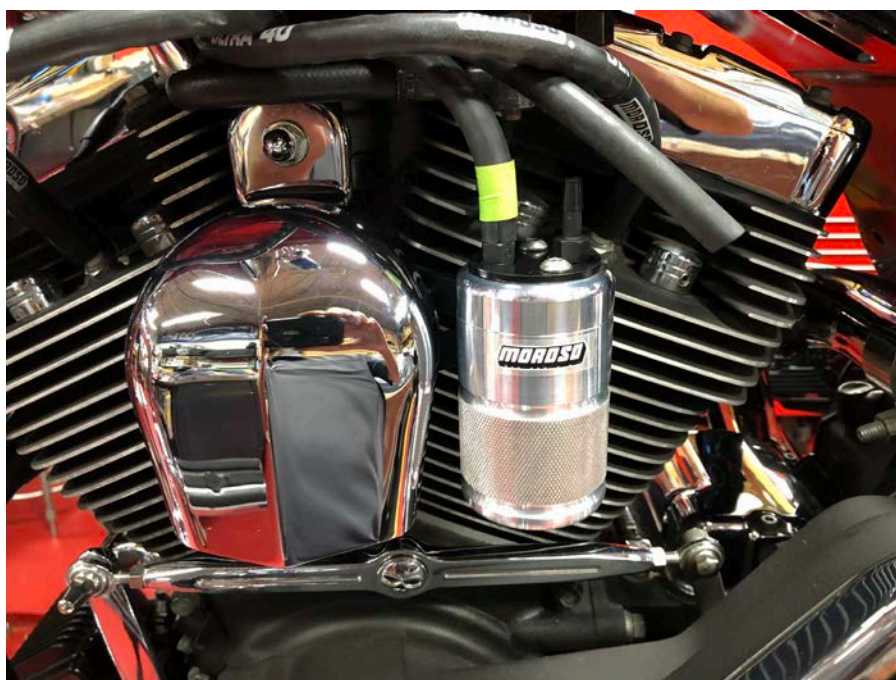
Step 29: Trim as needed and install crank case breather line with masking tape identifier to front barbed fitting as shown.
