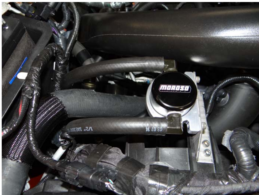
Step 22: Install hose to air Oil Separator, trimming of hoses will be required.
