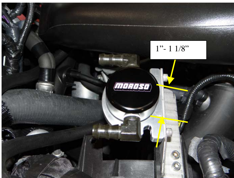
Step 21: Set height to 1" to 1 1/8, measured from billet clamp to top of Air Oil separator.
