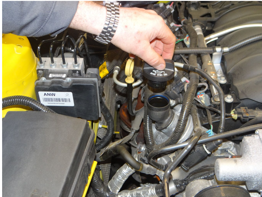
Step 2: Re-install oil fill cap.
