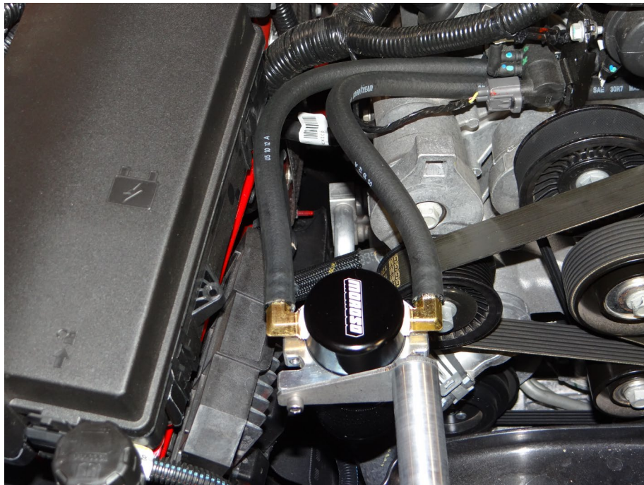
Step 11: Install 3/8 hoses to Air Oil Separator.
