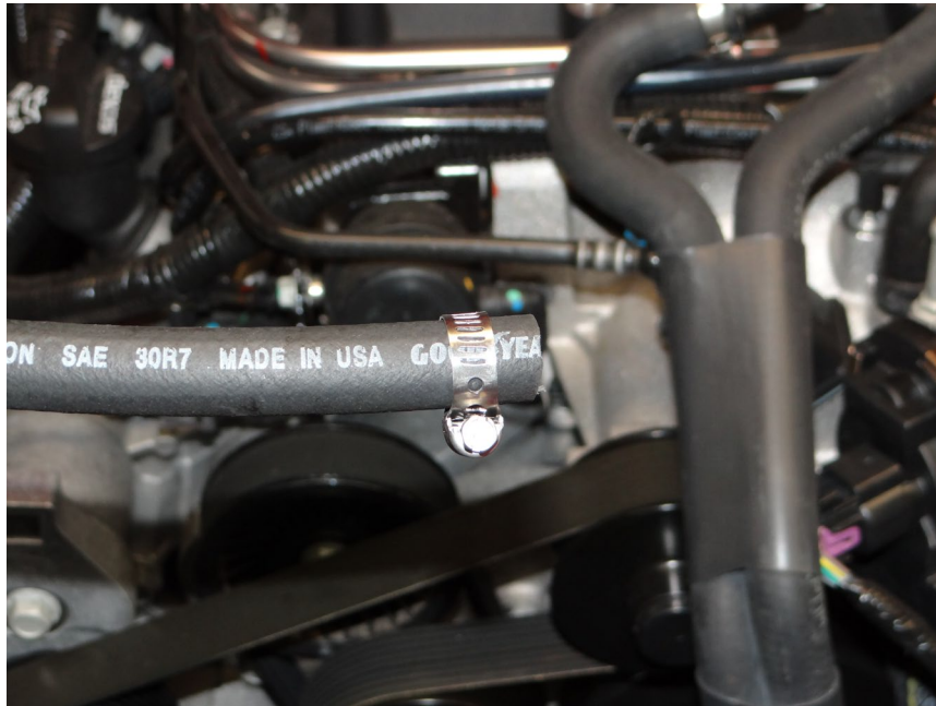
Step 6: Install hose clamp over 3/8 hose.
