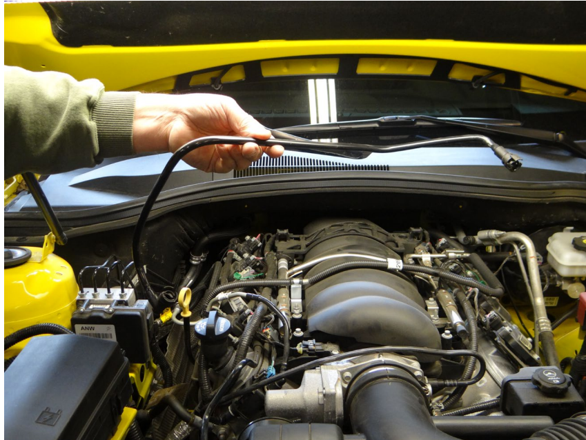
Step 6: Remove PCV line from vehicle.
