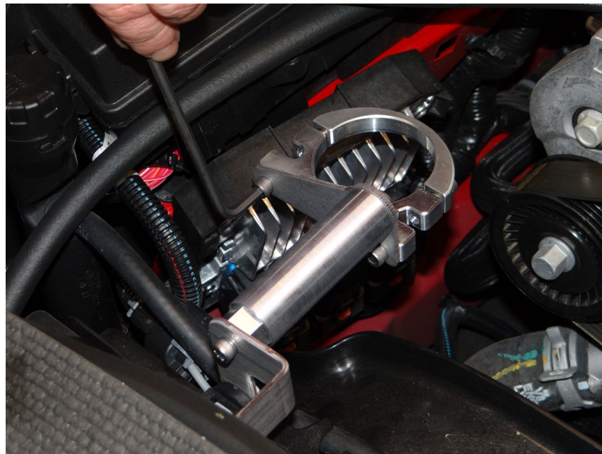
Step 7: Assemble billet clamp to stainless mount with relief facing down using (2) 1/4-20 SHCS.
