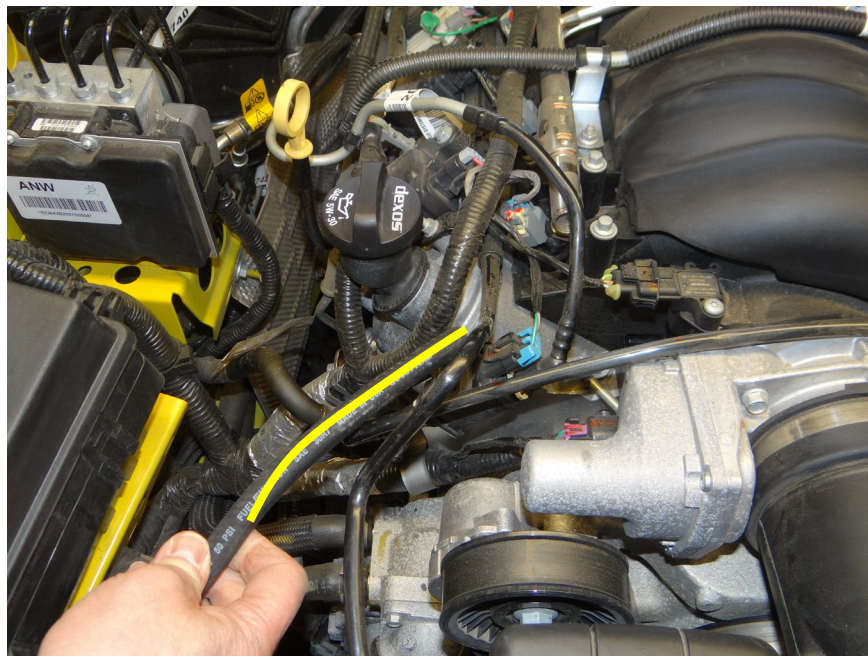
Step 7: Route 3/8 line from passengers side front of vehicle to drivers side rear valve cover as shown.
