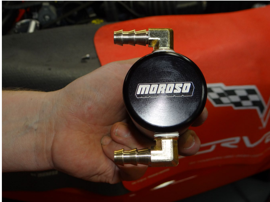
Step 8: Install barbed fittings as shown using Teflon tape.
