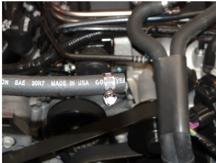
Step 3: Install hose clamp over 3/8 hose.
