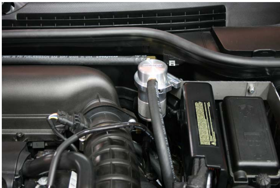
Step 37: Route throttle body hose to air oil separator and install hose over straight barbed fitting.
