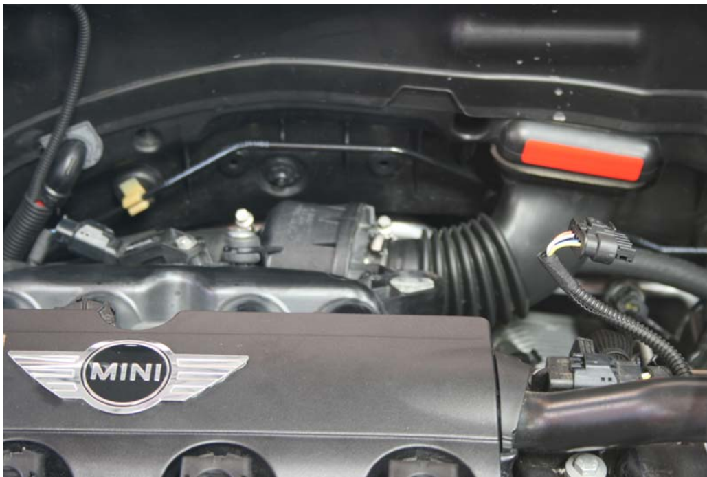
Step 22: Re-install by-pass valve.
