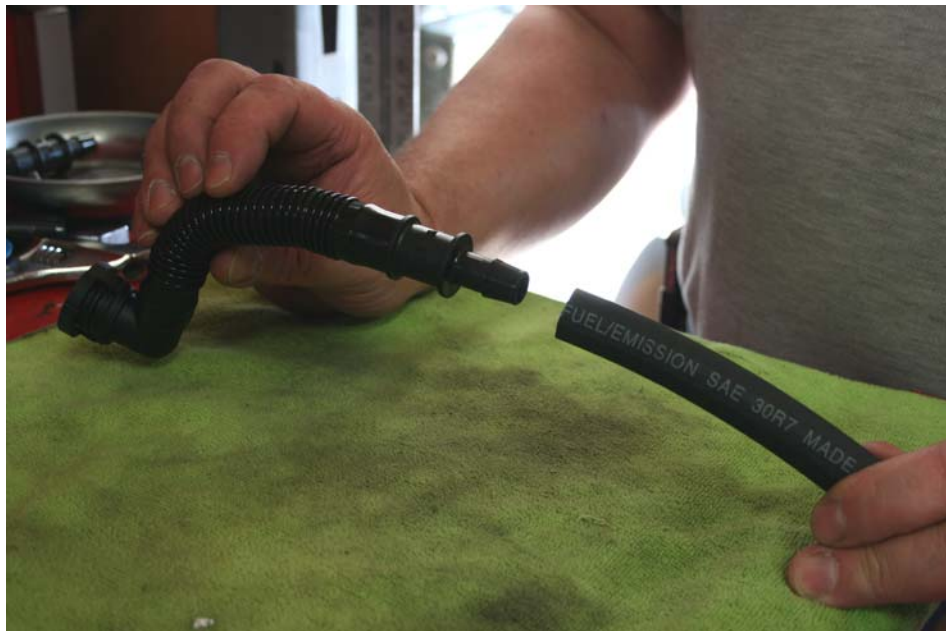
Step 16: Insert 1/2 side of coupling into 30" length of 1/2 ID hose.
