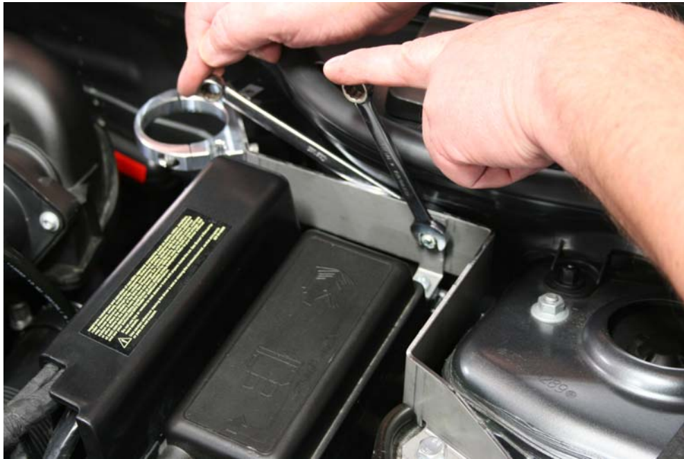
Step 33: Tighten fuse box tab hardware.
