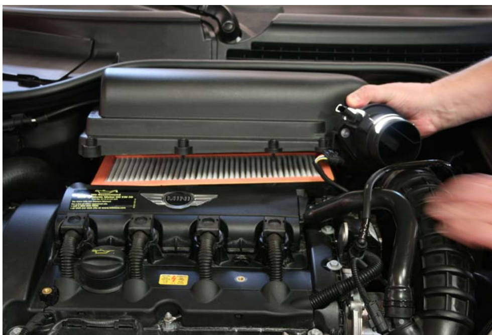
Step 4: Remove air box top from vehicle.
