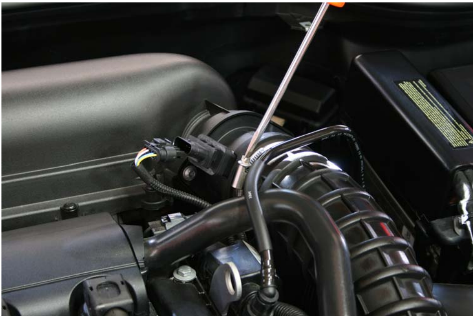
Step 2: Loosen air intake tube clamp.
