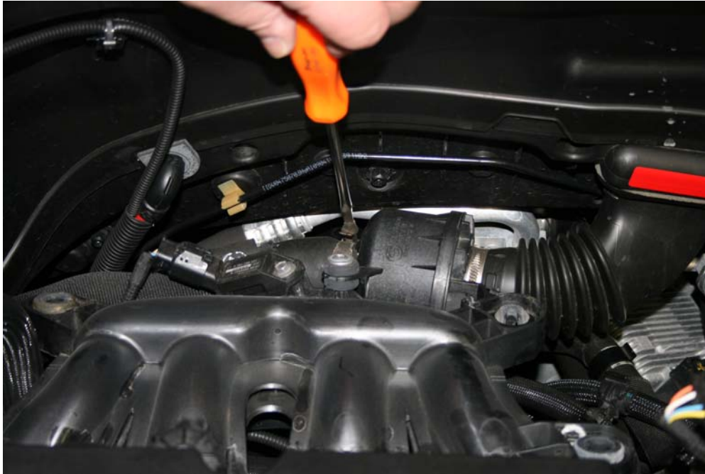
Step 9: Remove by-pass valve from vehicle as shown.
