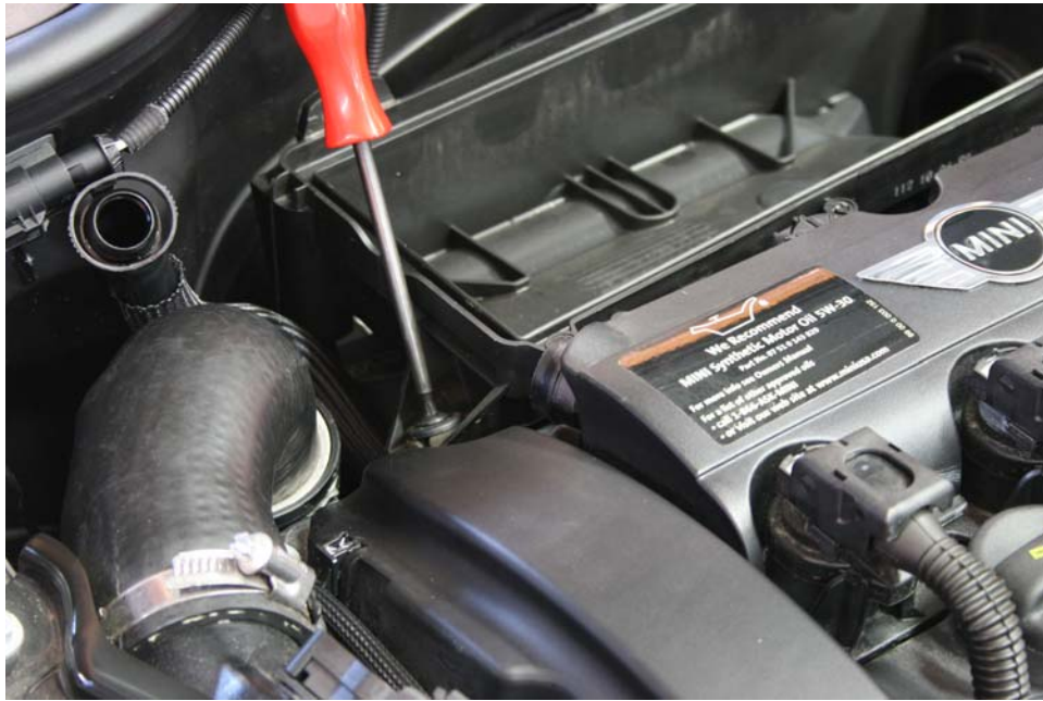
Step 8: Remove air box from vehicle as shown.
