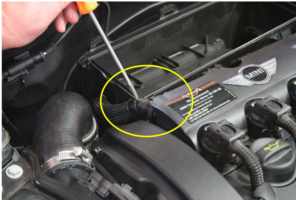
Step 7: Remove PCV line from valve cover.
