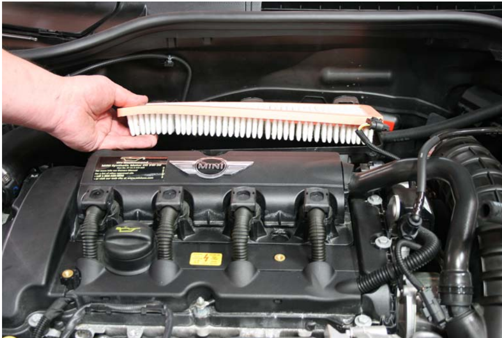
Step 25: Re-install air filter.
