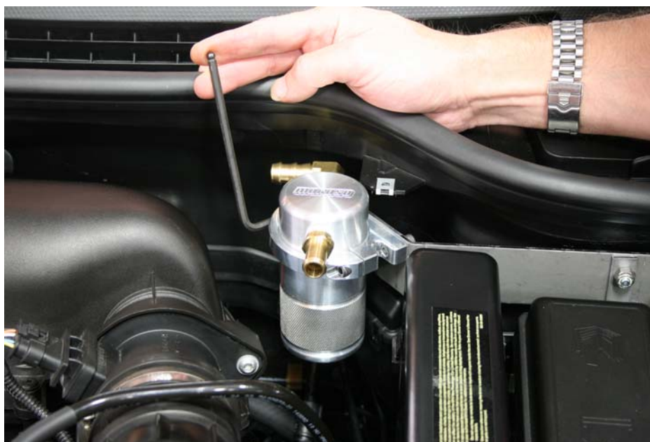
Step 35: Set Air Oil Separator in clamp 1" to 1 1/8" from top of billet clamp to top of air oil separator and tighten.
