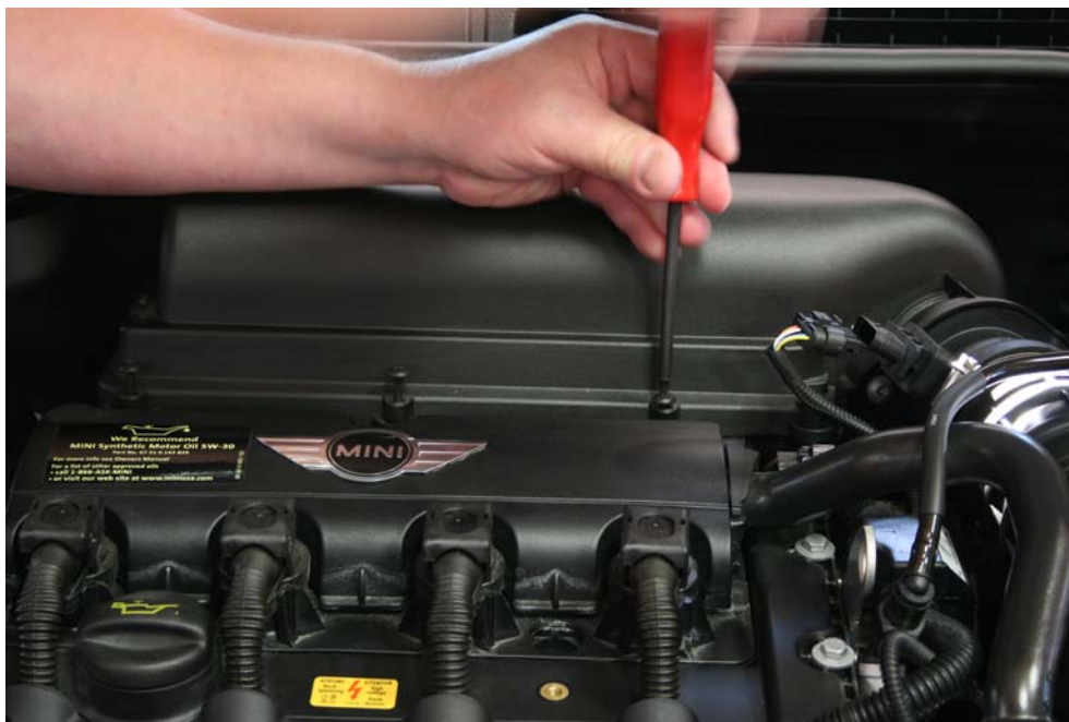
Step 3: Unscrew / Remove air box mounting hardware.
