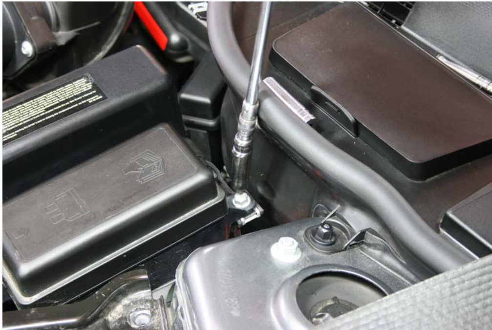
Step 31: Remove fuse box mounting bolt.
