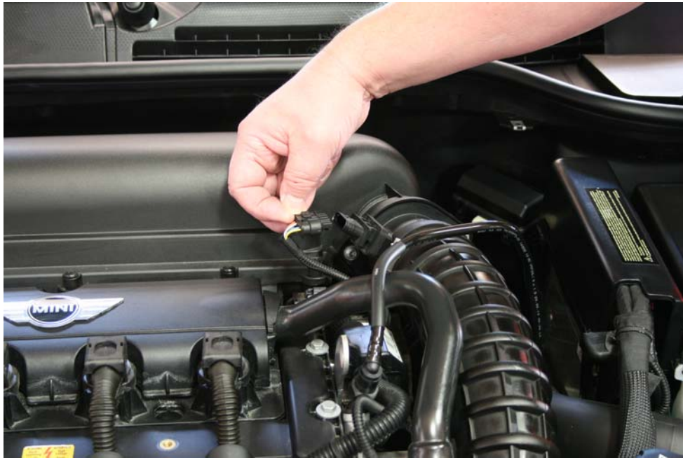
Step 1: Remove mass airflow sensor plug.
