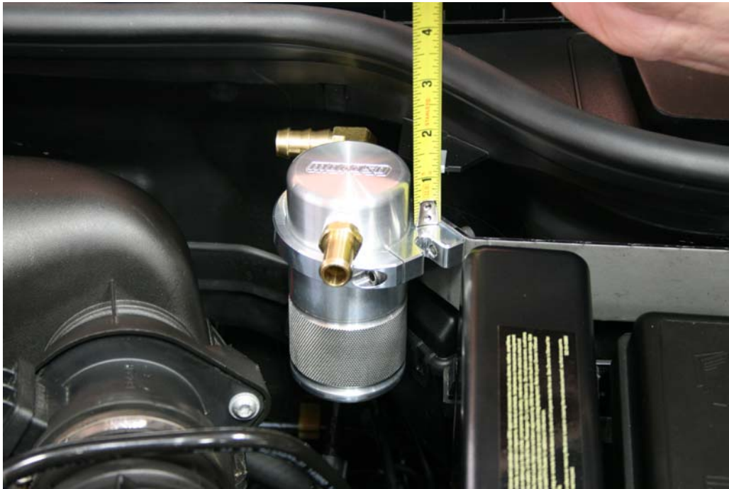
Step 35: Set Air Oil Separator in clamp 1" to 1 1/8" from top of billet clamp to top of air oil separator and tighten.
