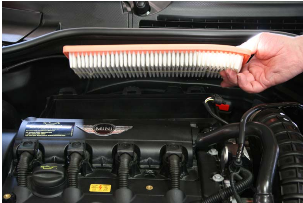
Step 5: Remove air filter.
