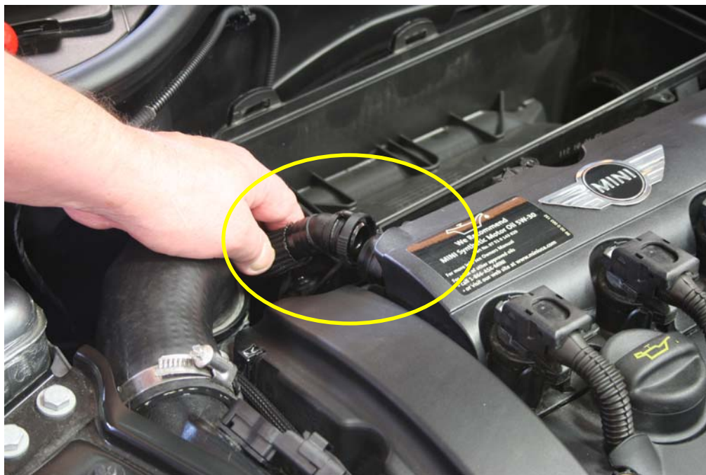
Step 7: Remove PCV line from valve cover.
