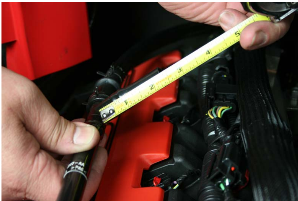
Step 4: Cut remainder of radius from PCV line leaving approximately 2 1/4" to 2 1/2" long straight area.
