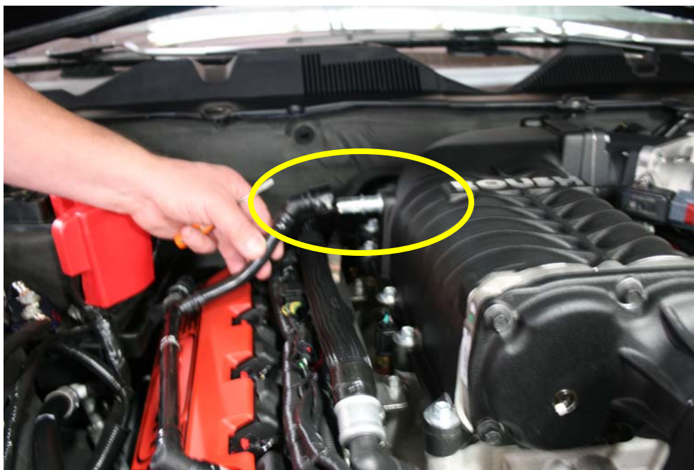
Step 2: Remove PCV line from Super Charger.
