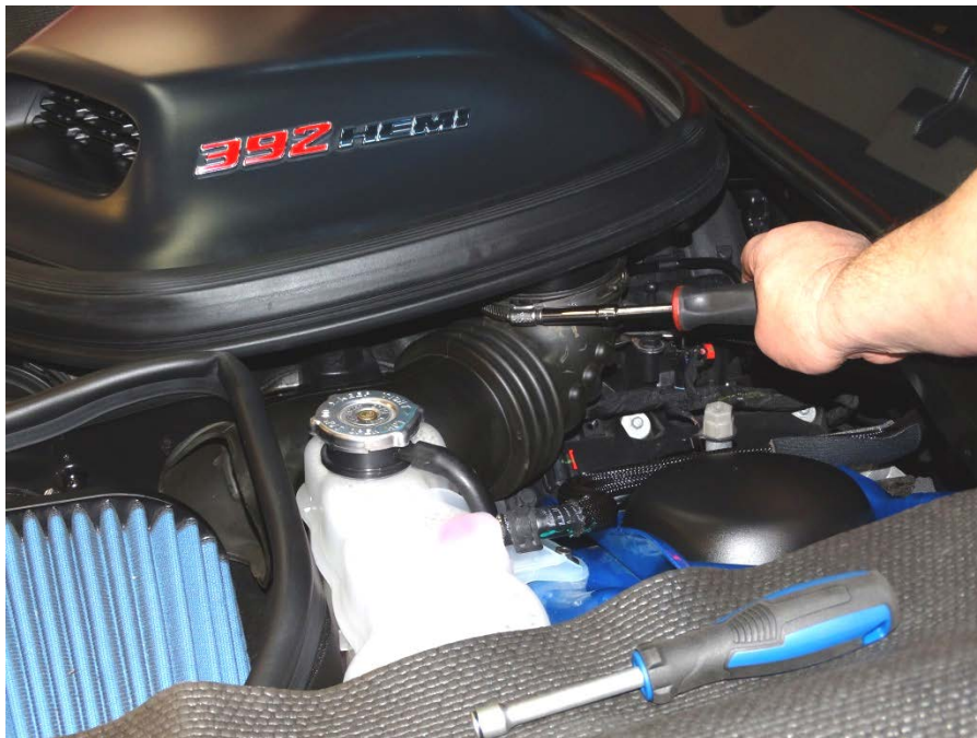
Step 2: Loosen air intake clamp.
