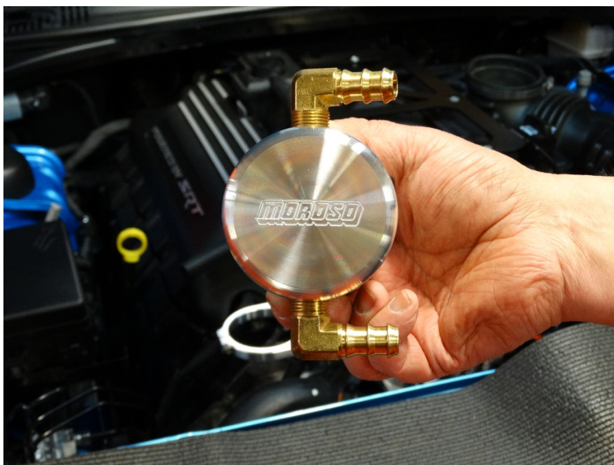
Step 16: Assemble air all separator as shown using Teflon tape on all fittings.
