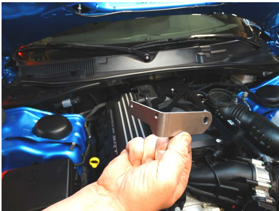
Step 6: Locate stainless steel mounting bracket provided in kit.
