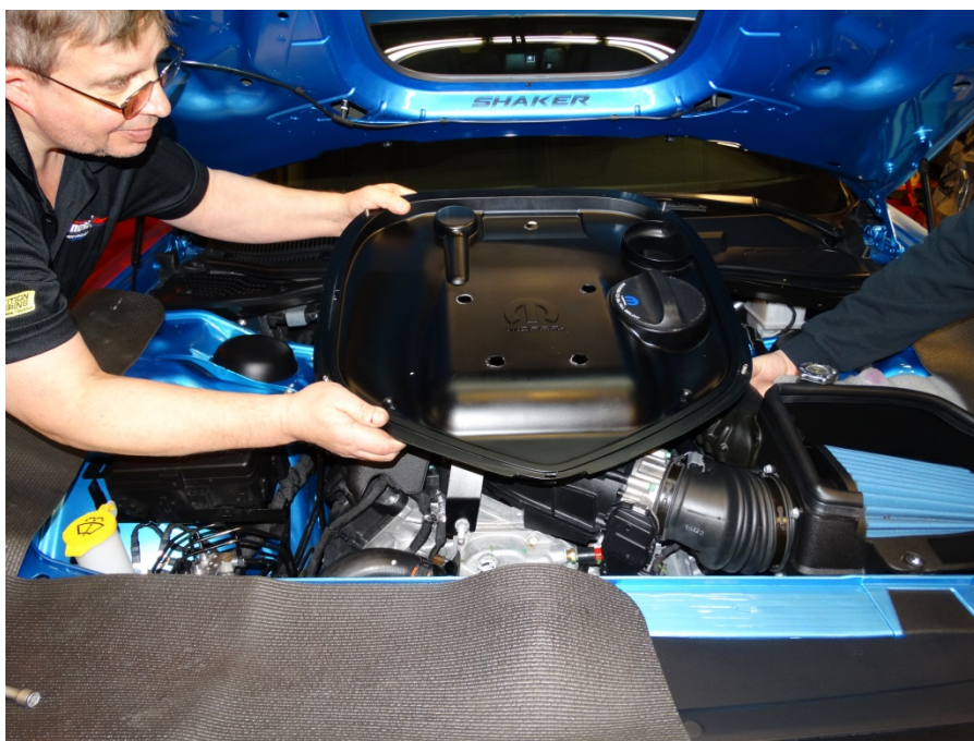
Step 5: Remove plenum from vehicle.
