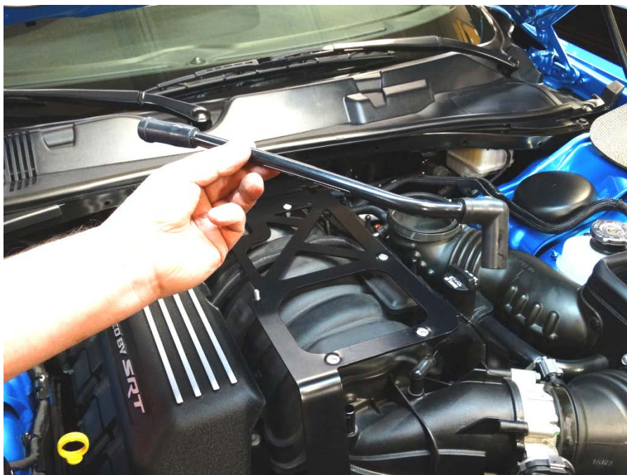
Step 8: Locate and remove PCV line from vehicle.
