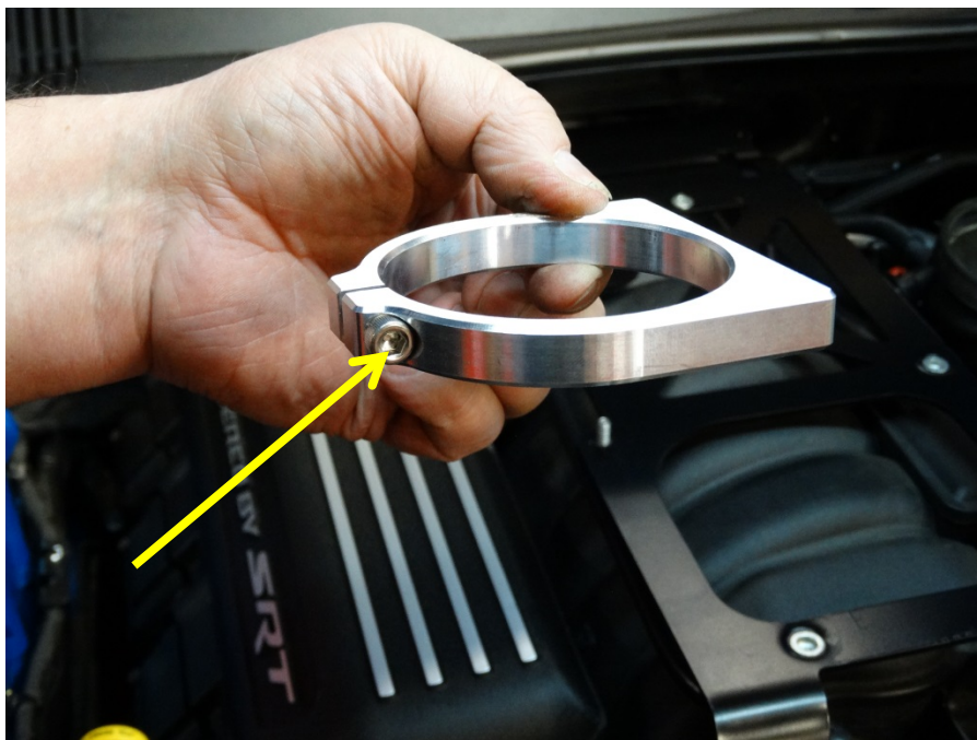
Step 14: Install \frac{1}{4} -20x1 SHCS in billet clamp, do not tighten
