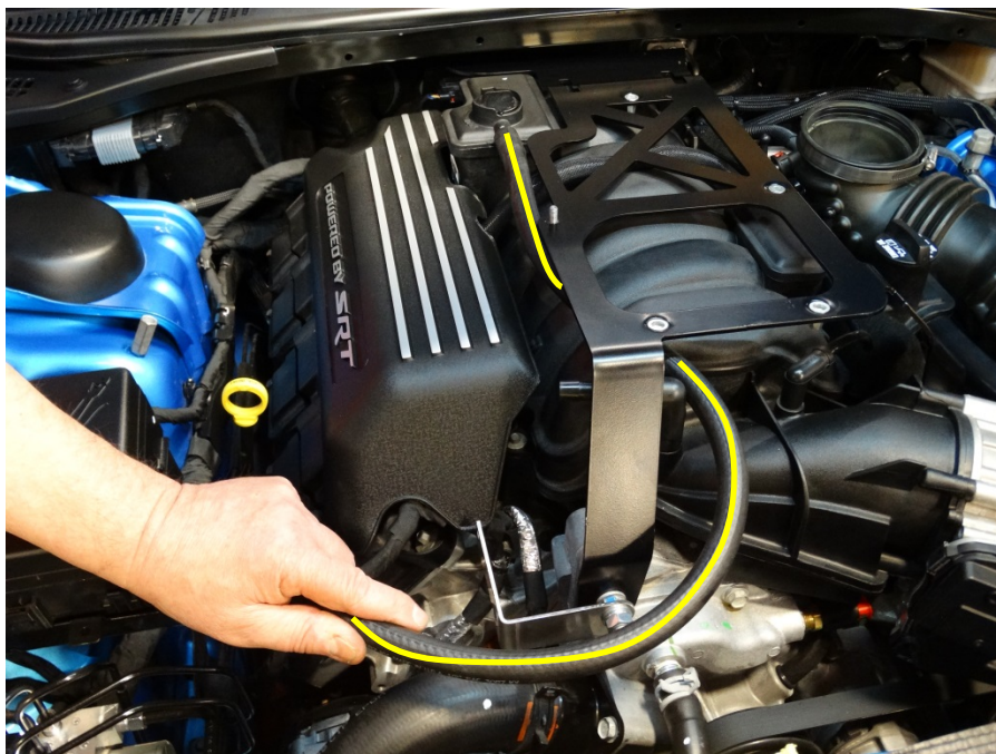
Step 12: Install long length of hose provided in kit as shown.
