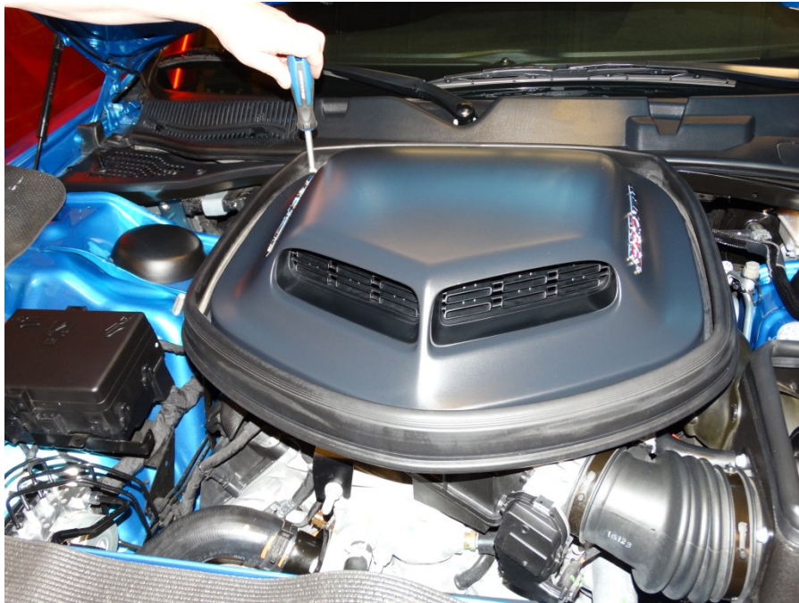
Step 1: Remove Shaker intake fasteners.
