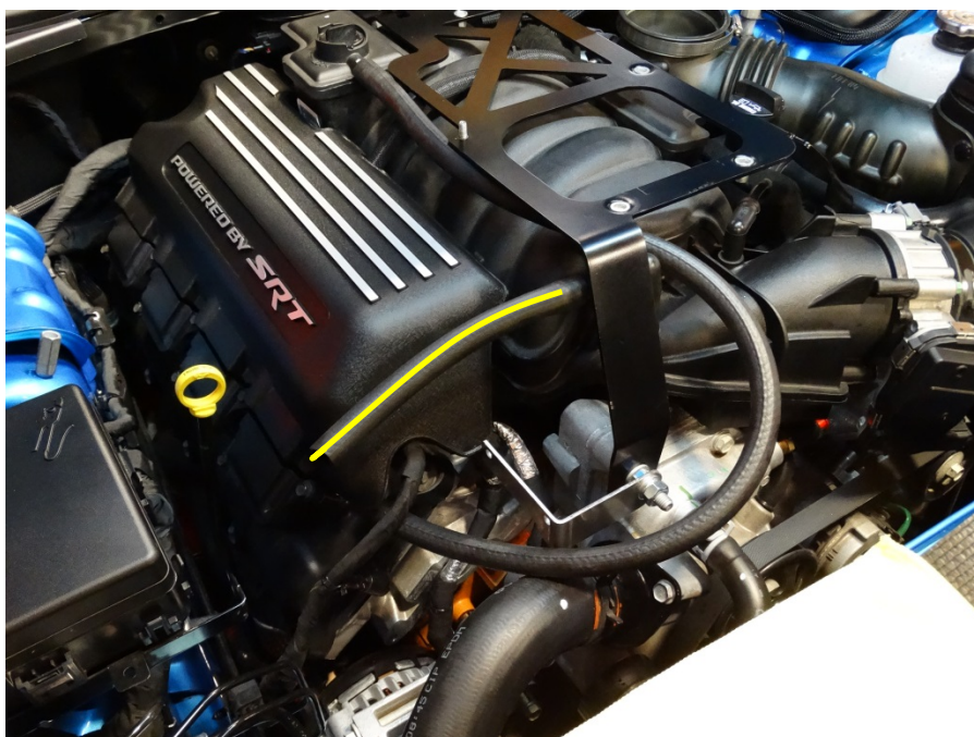
Step 13: Install short length of hose provided in kit as shown.
