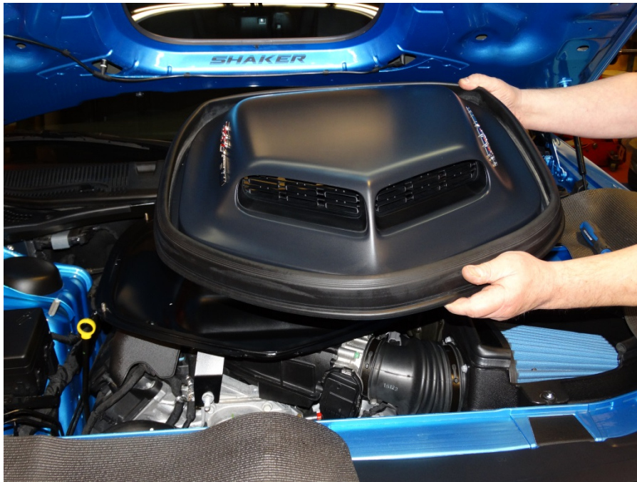
Step 3: Remove Shaker intake from vehicle.
