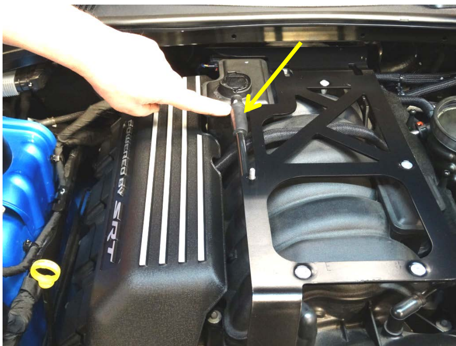
Step 8: Locate and remove PCV line from vehicle.
