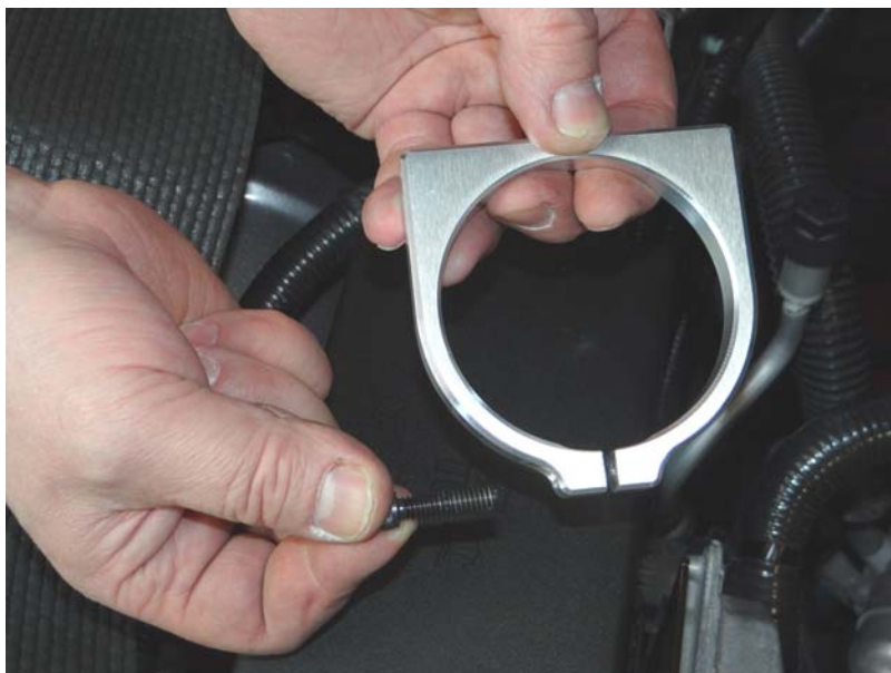
Step 9: Install 1/4-20 x 1" SHCS into billet clamp as shown.
