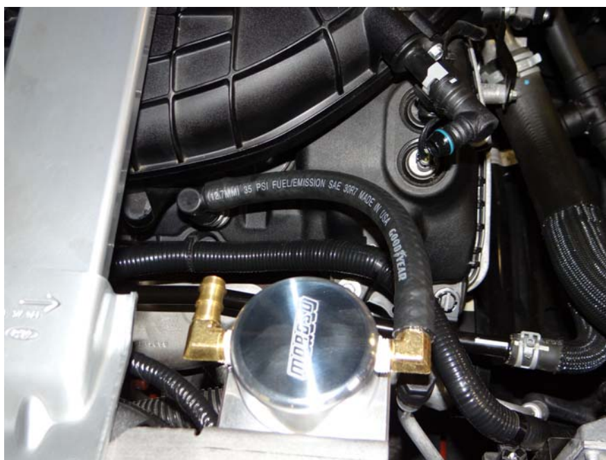
Step 14: Install other end to Air Oil Separator as shown.
