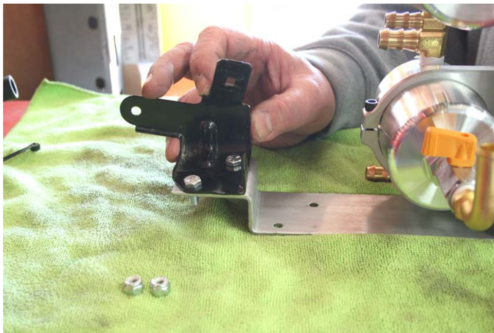
Step 42: Install wiring harness bracket to Air Oil Separator bracket using supplied Hex bolts and nylock nuts as shown.
