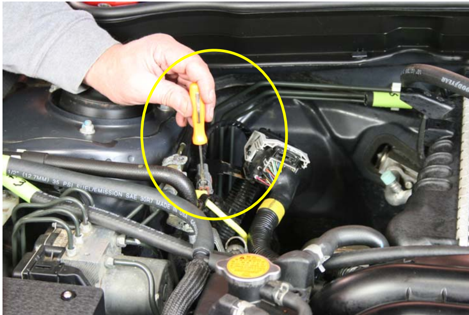
Step 36: Unplug small 4 pin connector as shown.
