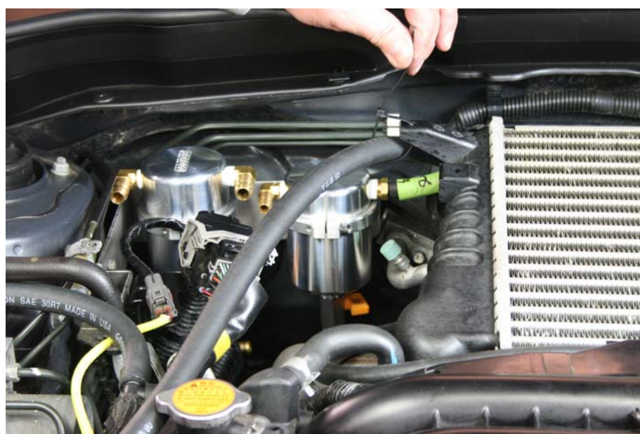
Step 47: Wire tie hose #1 to inter cooler.
