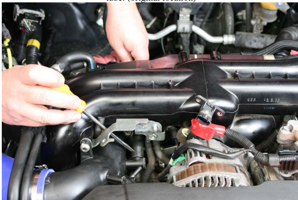
Step 11: Reinstall original breather line removed in step 5 and 6 to nipple on air intake tube. (original location)
