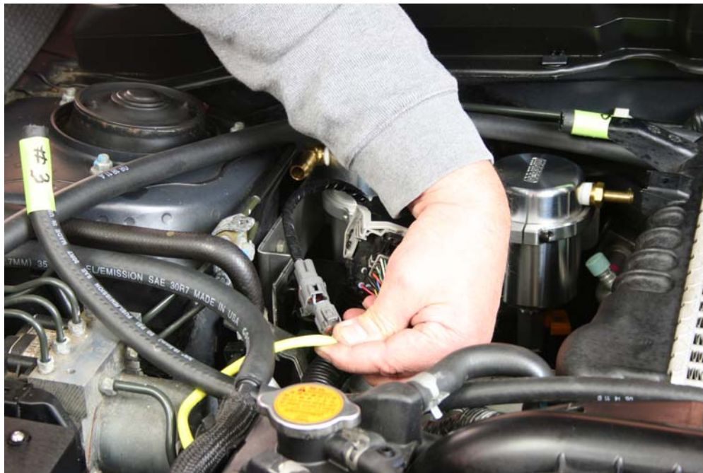
Step 45: Reinstall 4 pin plug on bracket.
