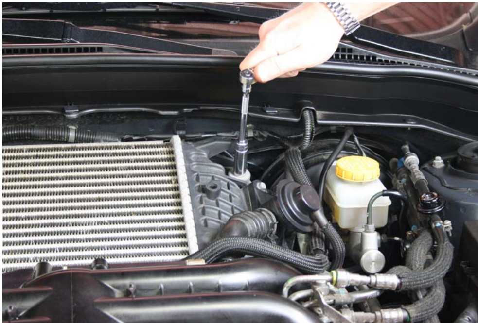
Step 1: Remove intercooler from vehicle.
