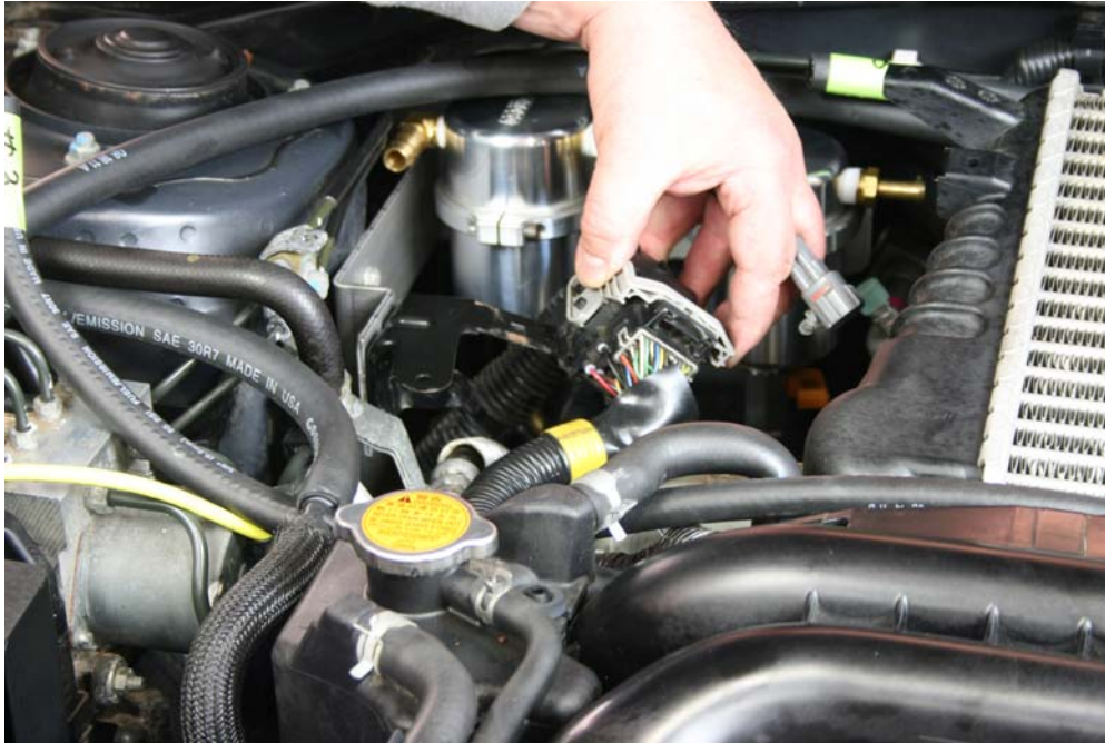
Step 44: Reinstall wire harness plug on bracket.
