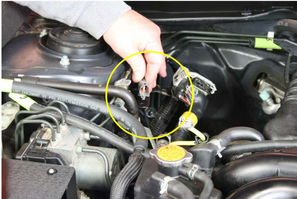
Step 38: Remove plug from bracket.
