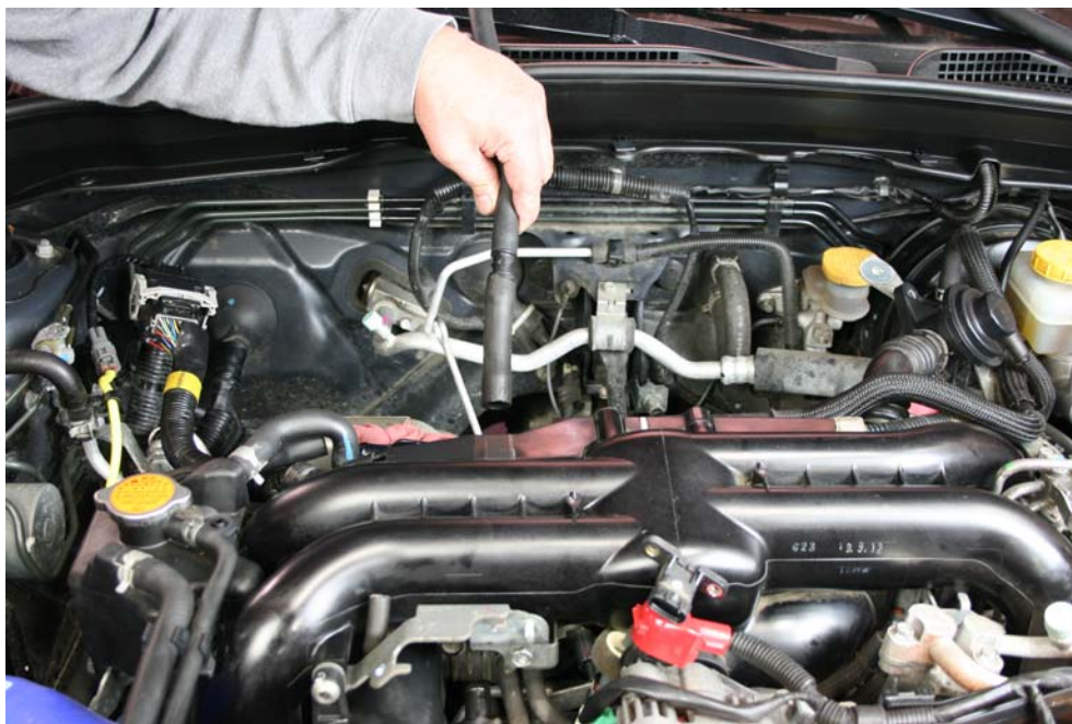
Step 11: Reinstall original breather line removed in step 5 and 6 to nipple on air intake tube. (original location)
