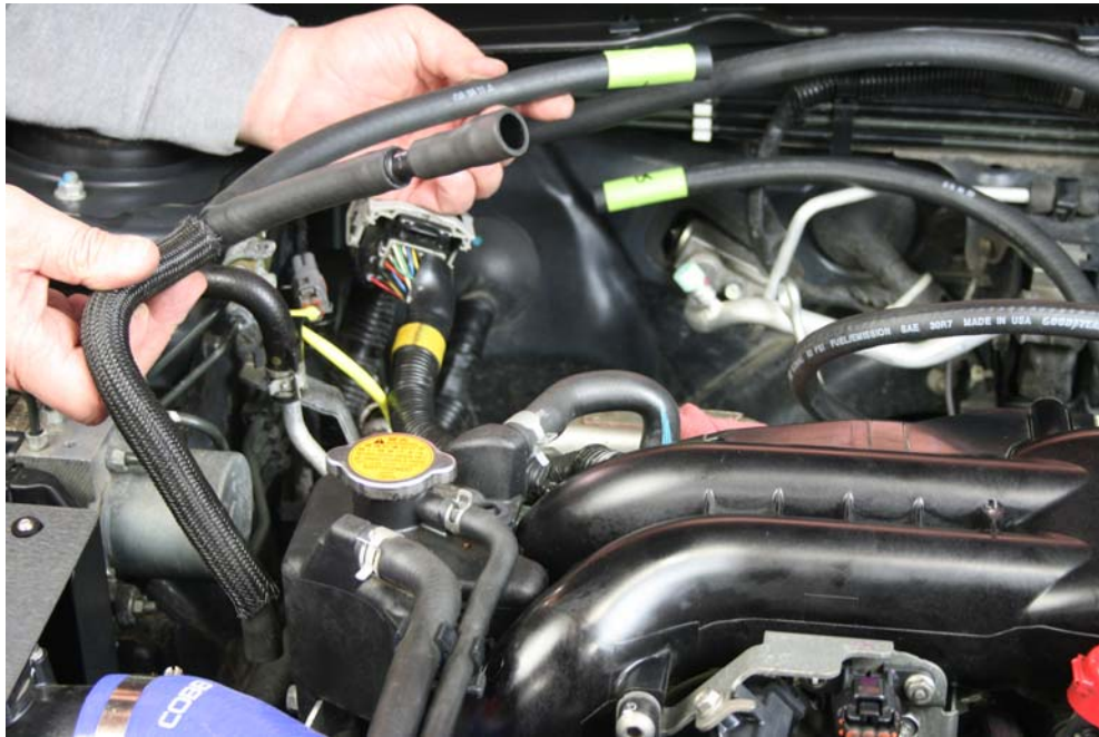
Step 32: Insert stock hose over nipple on valve cover.
