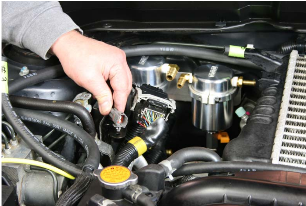
Step 45: Reinstall 4 pin plug on bracket.
