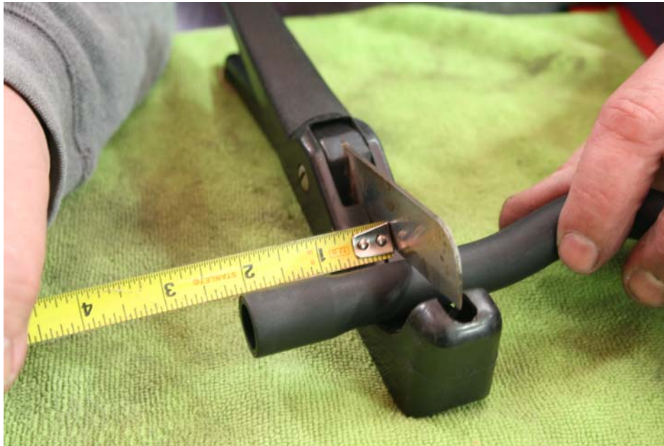
Step 24: Cut cross over end of tube at 2 1/8".
