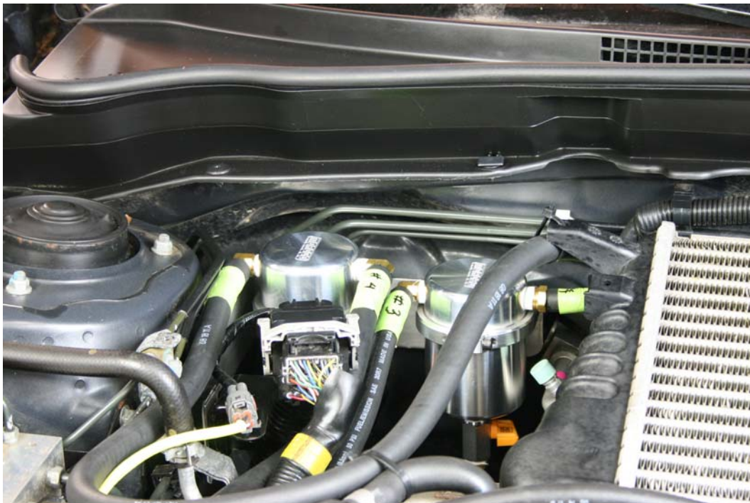
Step 50: Route hose #4 from valve cover crossover hose assembly to 1/2" 90 degree barb.
