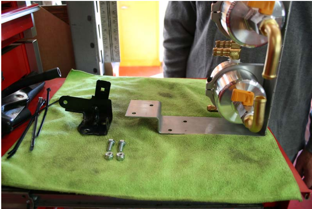
Step 42: Install wiring harness bracket to Air Oil Separator bracket using supplied Hex bolts and nylock nuts as shown.
