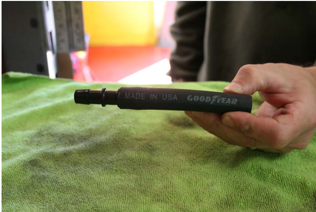
Step 25: Insert \frac{1}{2} coupling into end of 4 \frac{1}{2} long \frac{1}{2} hose.
