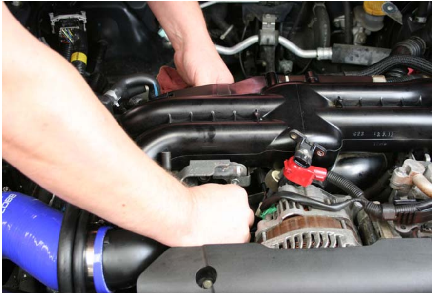
Step 5: Gently remove valve cover cross over tube from breather line
