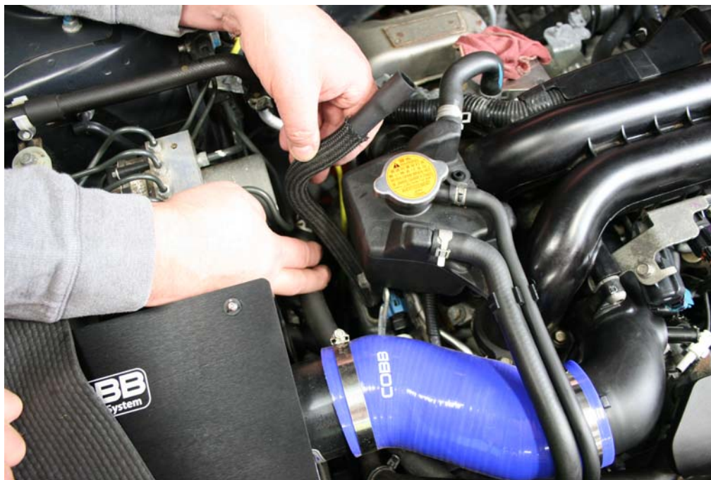
Step 22: Remove vent line from passenger side valve cover.
