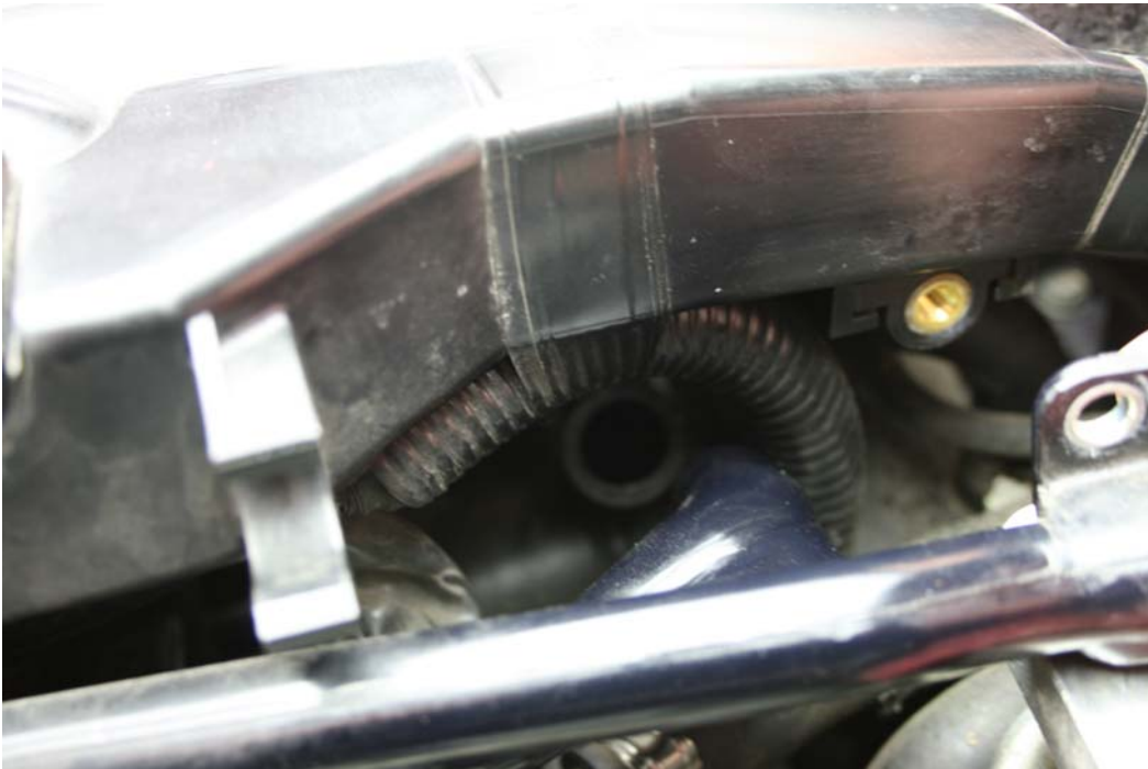
Step 5: Gently remove valve cover cross over tube from breather line
