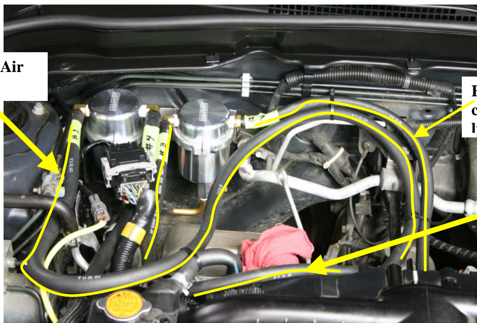
Final hose routing shown with Air Oil Separators installed and intercooler removed for clarity.
