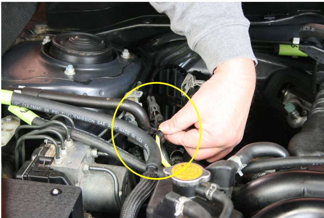
Step 37: Unclip wire retainer from hose as shown.
