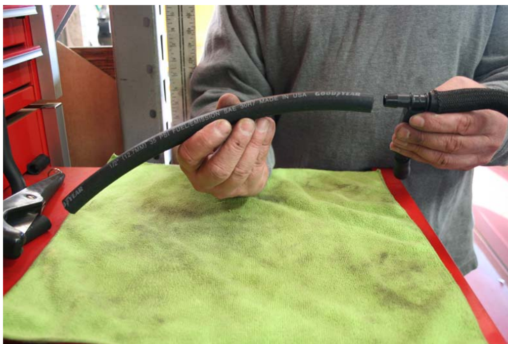
Step 30: Insert 13" long 1/2" hose over remaining nipple on tee as shown.
