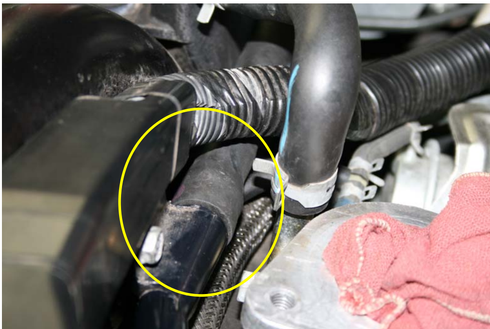
Step 33: Install 5/8" end of hose over crossover tube nipple.
