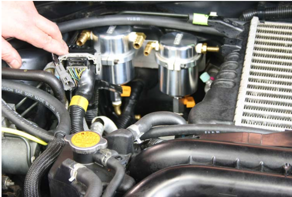
Step 44: Reinstall wire harness plug on bracket.
