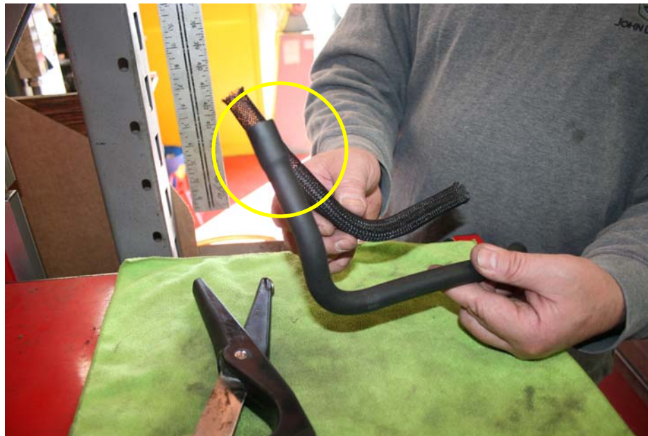
Step 23: Remove outer protector from vent line.
