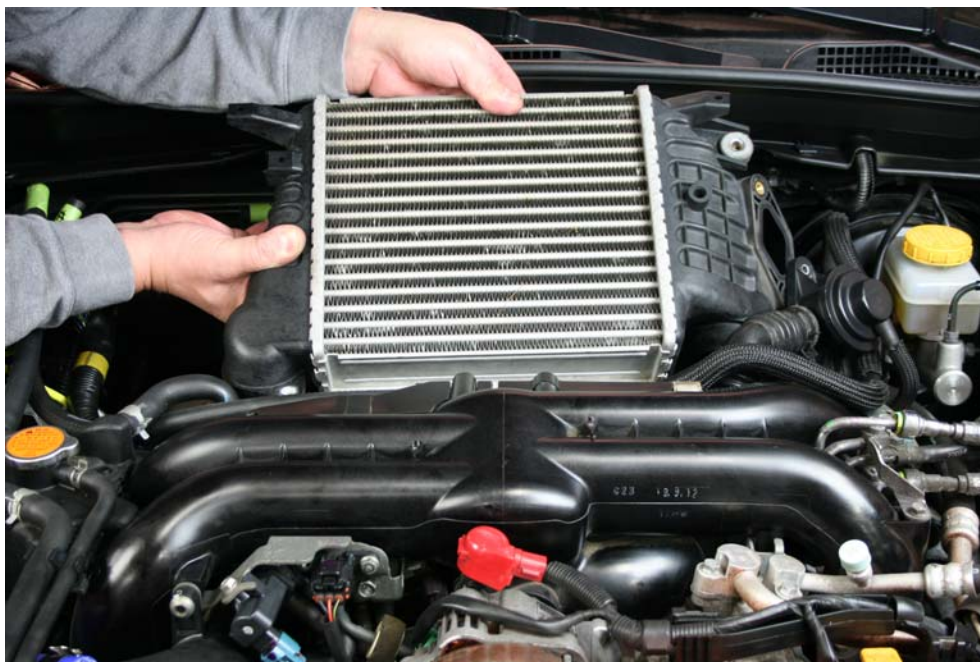
Step 34: Reinstall intercooler.
