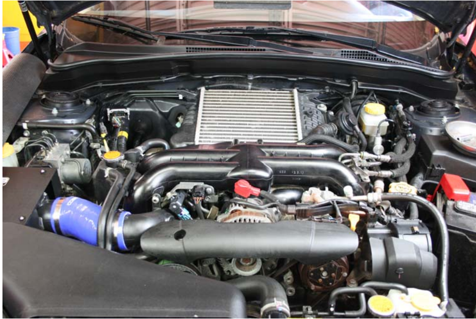
Step 1: Remove intercooler from vehicle.
