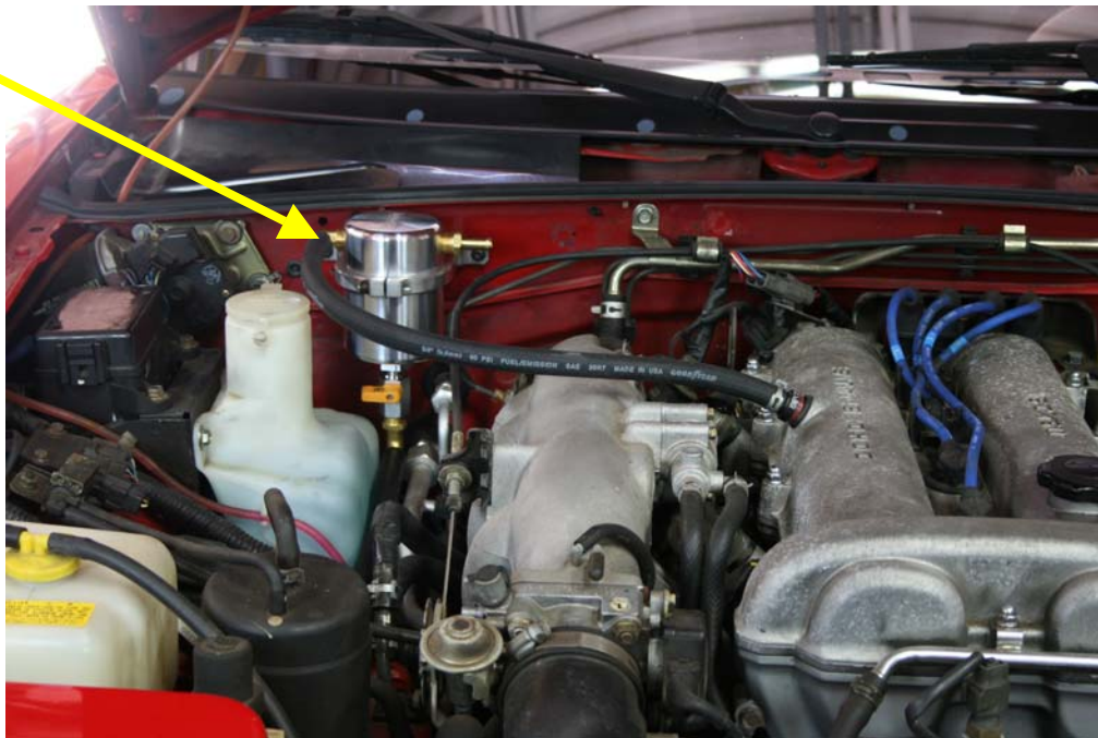
Step 20: Install other end of hose to Air Oil Separator as shown
