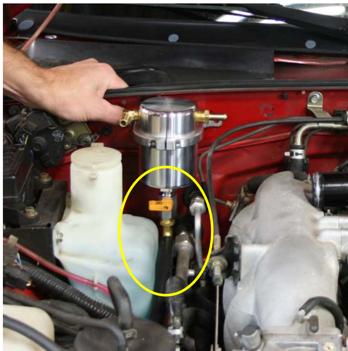
Step 5: Place Air Oil Separator against passenger side firewall as shown making sure drain hose and ball valve are orientated correctly
