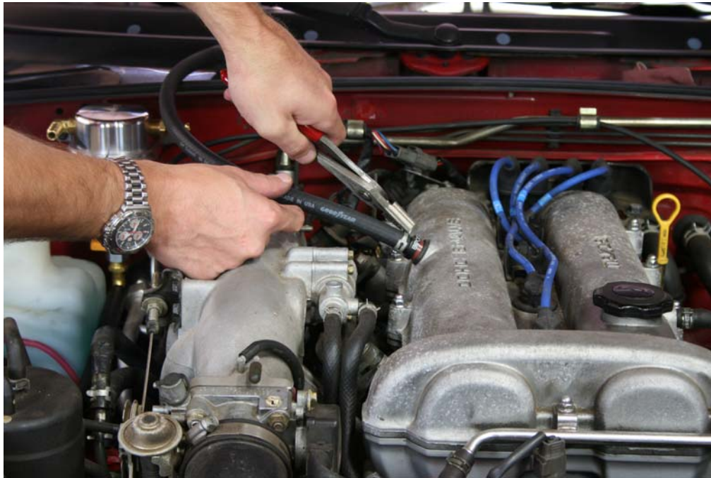
Step 19: Install hose clamp
