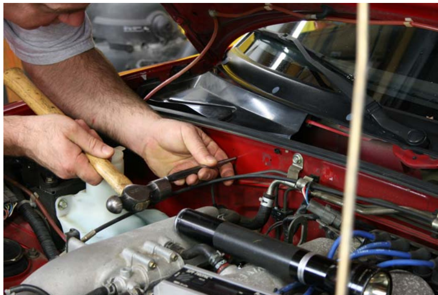
Step 7: Center punch hole locations previously marked
