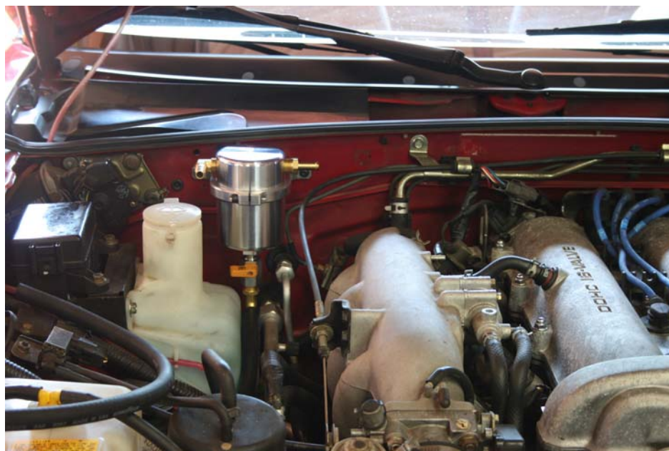
Step 13: Install Air Oil Separator on firewall
