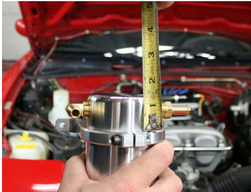
Step 3: Assemble billet clamp 1 1/4" down from top of Air Oil Separator
