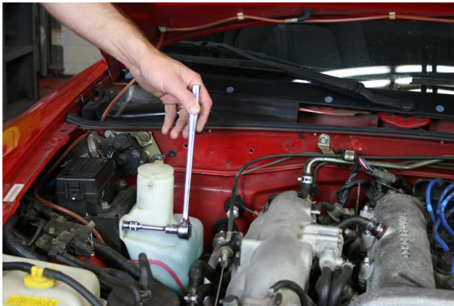
Step 11: Reinstall windshield washer tank mounting bolts
