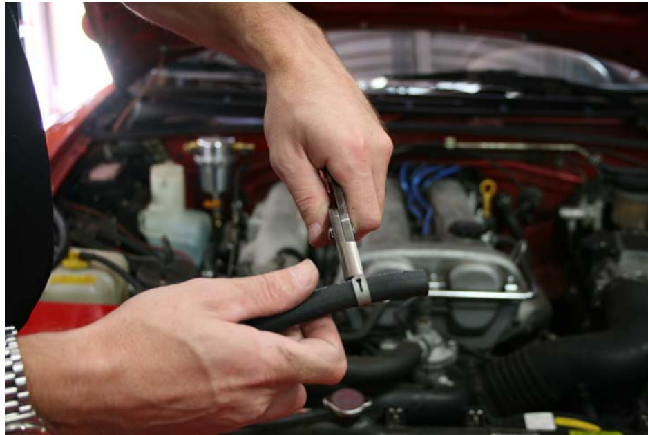
Step 17: Install (1) hose clamp on one end of 19" hose
