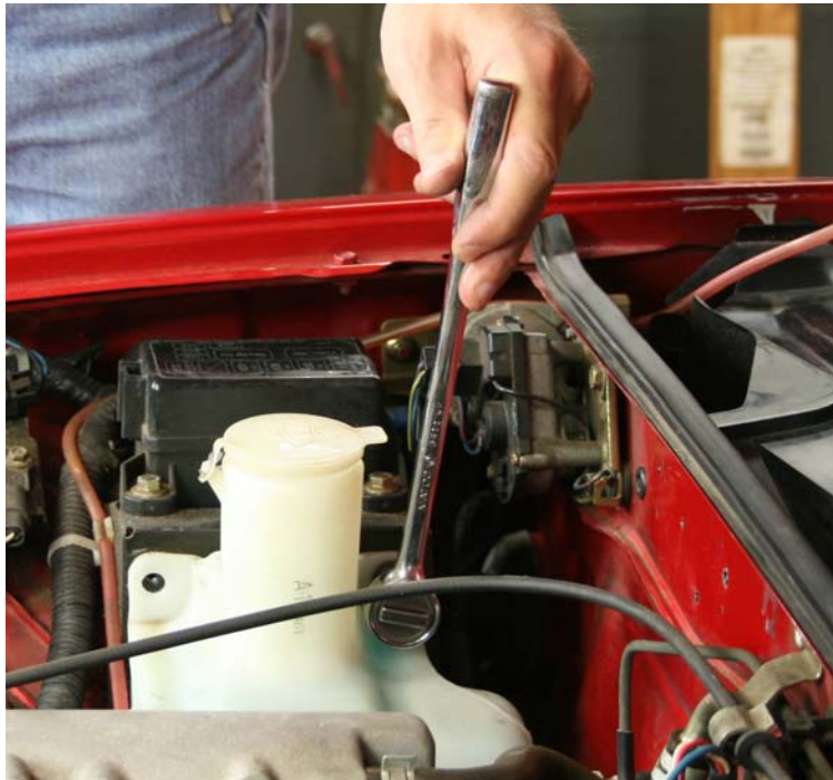
Step 8: Remove (2) mounting bolts from windshield washer bottle
