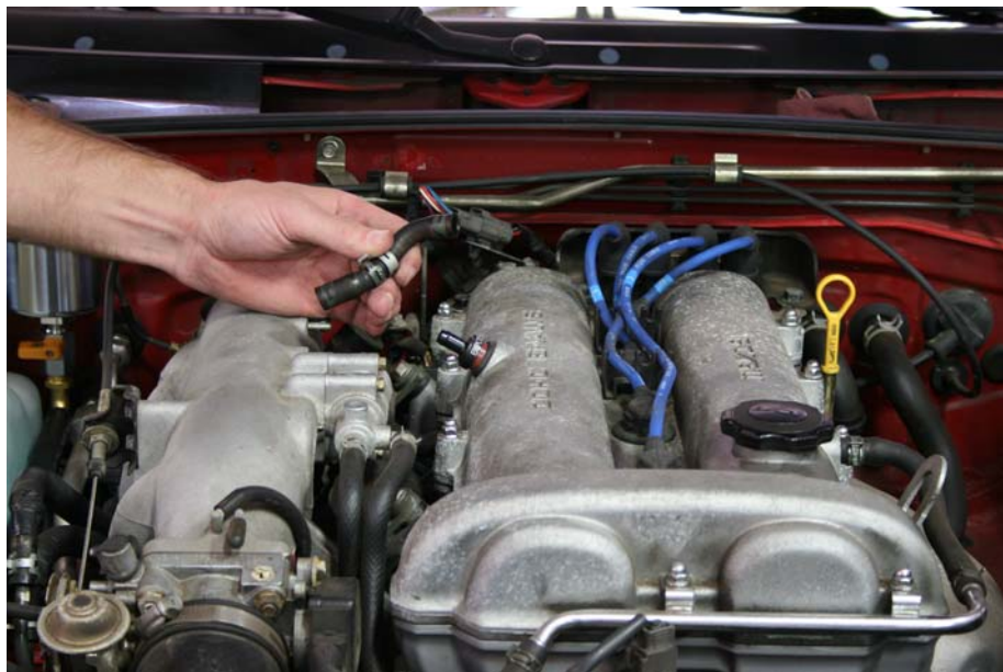
Step 16: Remove PCV line from vehicle, remove hose clamps for re-use
