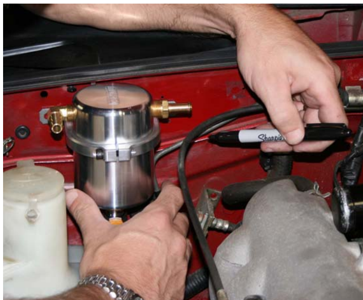
Step 6: Mark location of mounting bracket holes on firewall (2) places
