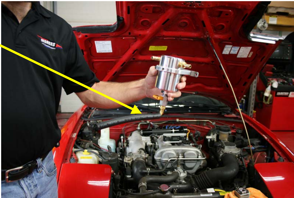
Step 4: Install 1/2 " hose over drain nipple
