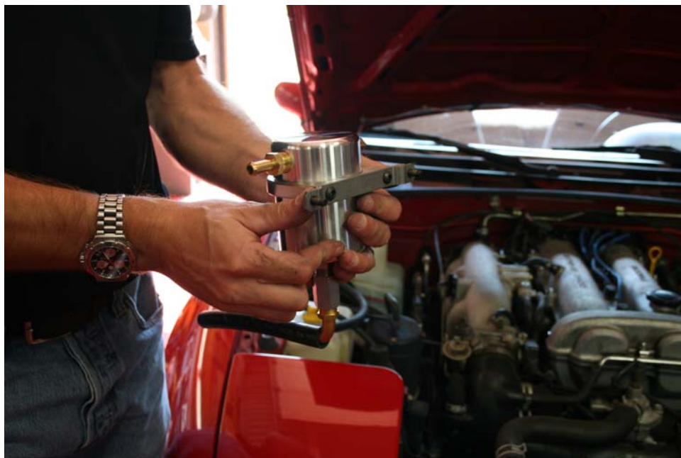
Step 12: Insert (2) 1/4 X 20 BHCS X 5/8 thru stainless mounting bracket holes
