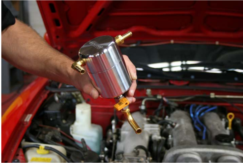
Step 2: Assemble Air Oil Separator as shown applying Teflon tape to all fittings
