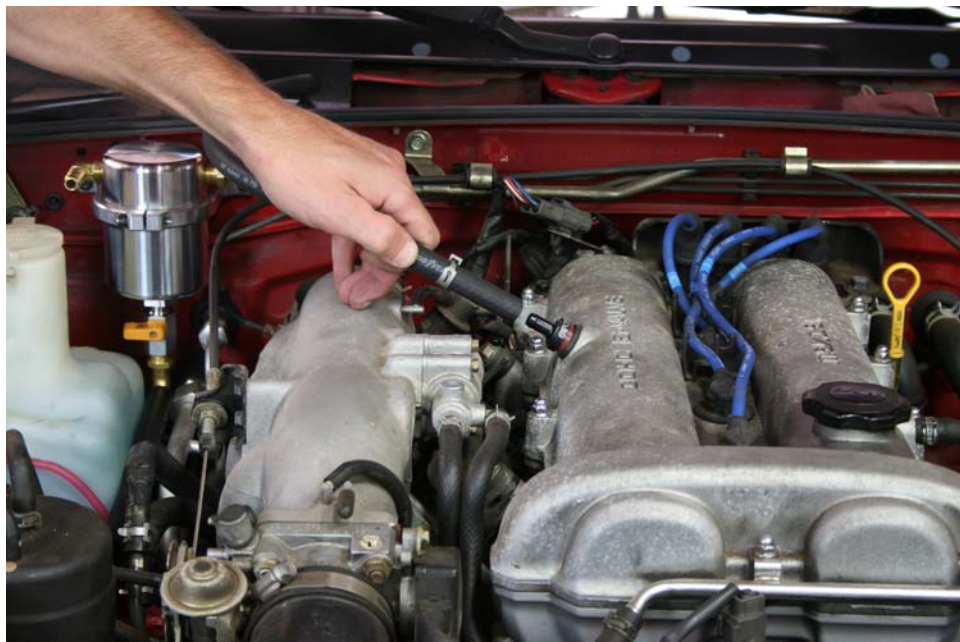
Step 18: Install hose over PCV nipple
