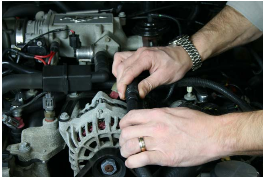
Step 25: Insert ½" hose over ½" coupling
