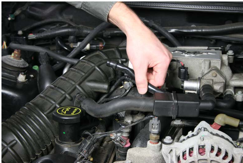
Step 2: Remove lines from Air Intake hose
