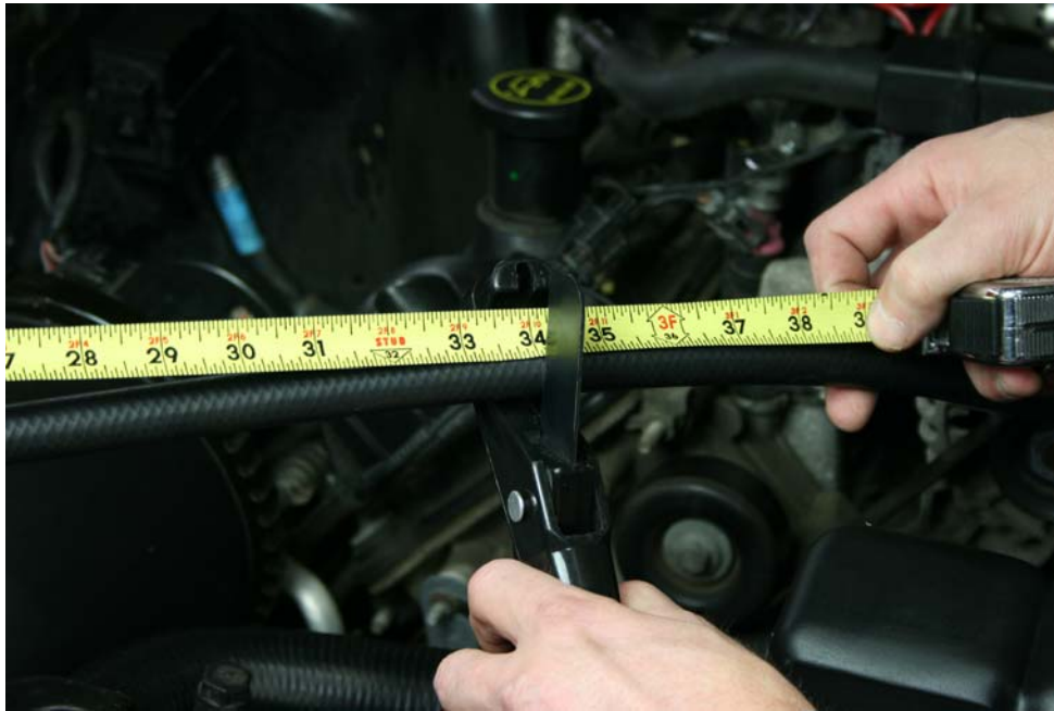
Step 14: cut 1 pc of ½" hose to 34"
