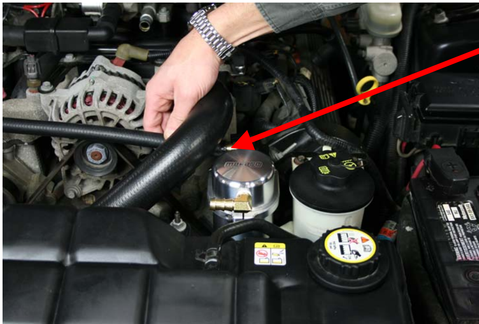
Step 15: Insert one end of ½" hose to rear fitting on Air Oil Separator
