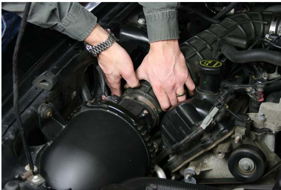
Step 28: Re-Install Air Intake hose to Air Box
