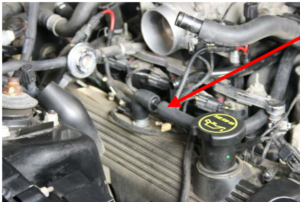
Step 19: Insert 1/2" hose over coupling
