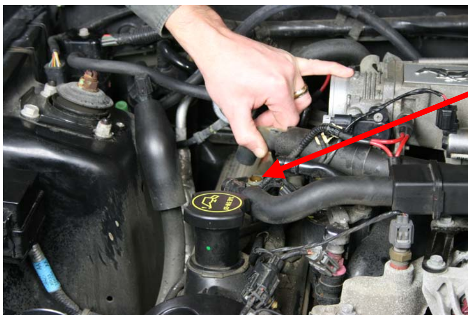
Step 6: Remove tube from PCV Valve
