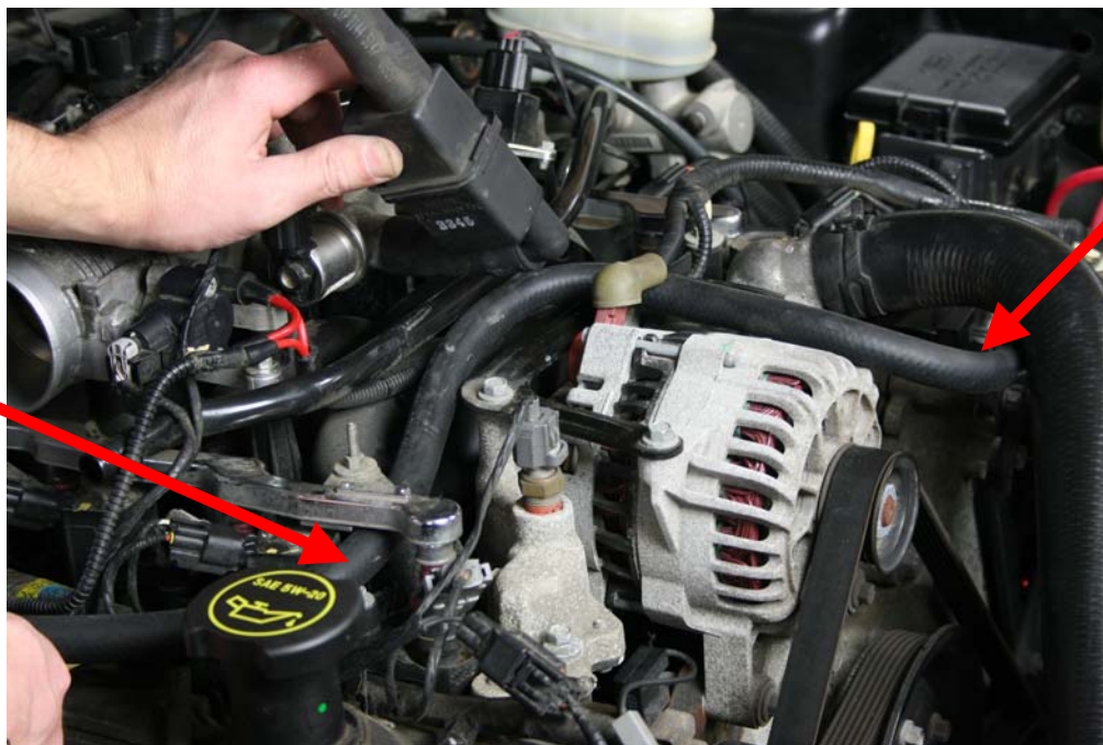
Step 16: Route ½" hose from Air Oil Separator to Valve Cover as shown
