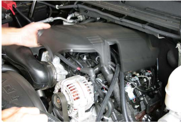
Step 22 Re-install intake cover
