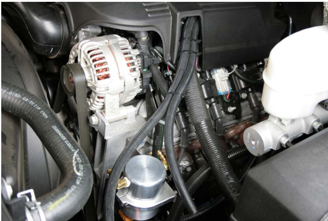
Step 23 Wire tie 3/8" lines as shown
