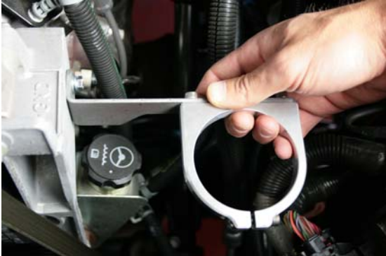
Step 18 Install billet / stainless bracket to upper hole on alternator bracket
