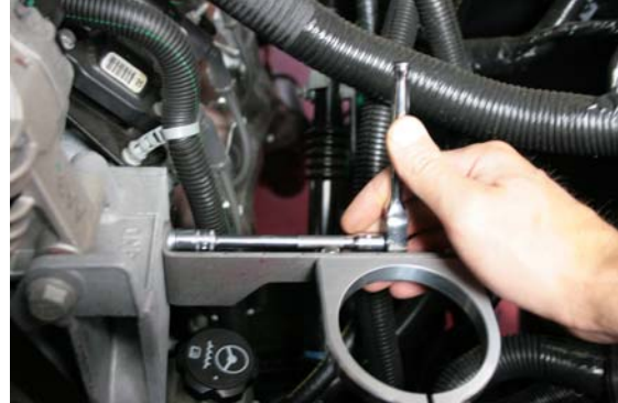
Step 18 Install billet / stainless bracket to upper hole on alternator bracket
