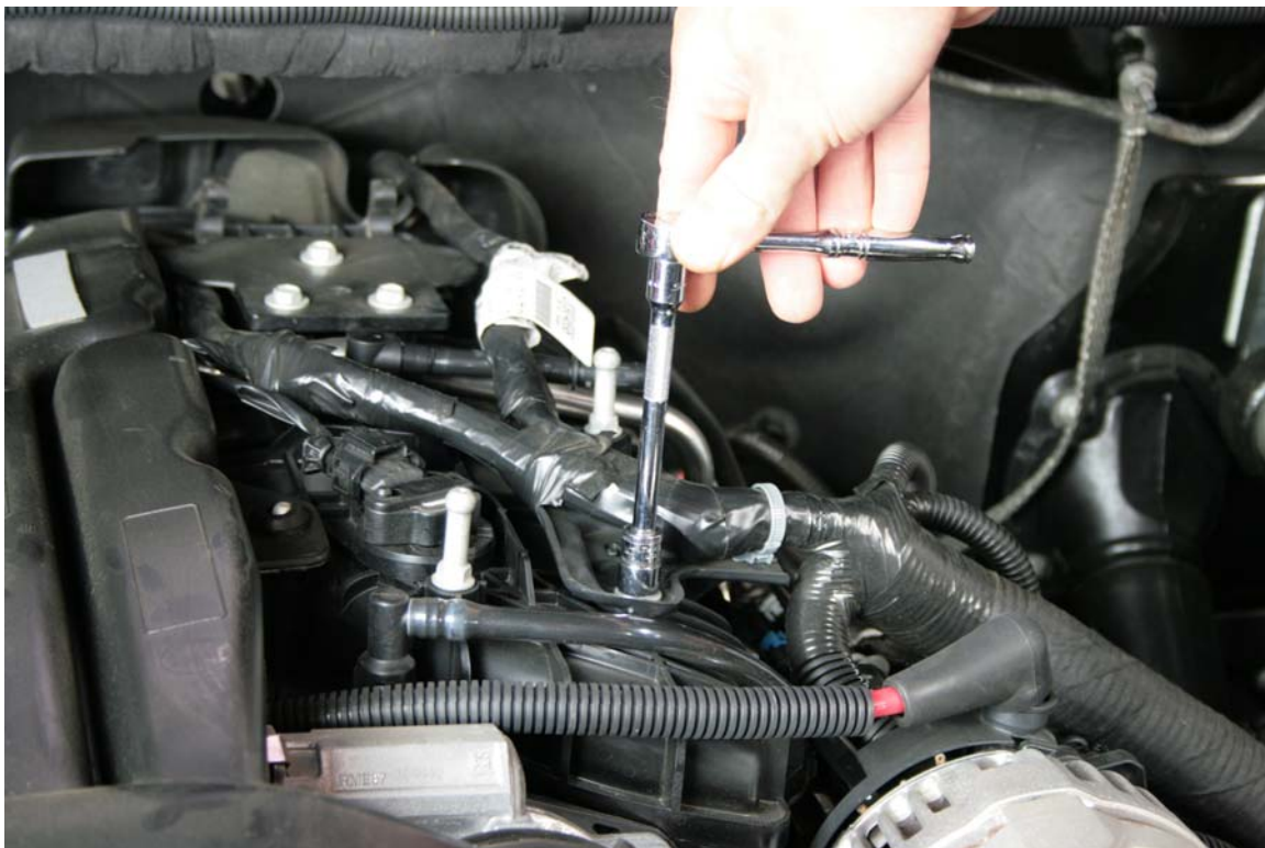
Step 15 Re-install wiring harness as shown
