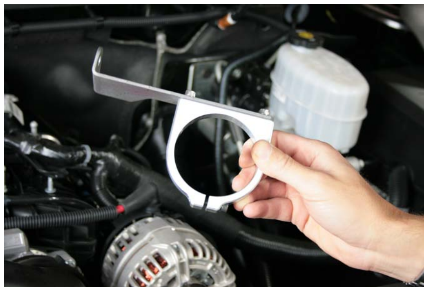
Step 17 Assemble billet bracket and stainless bracket as shown
