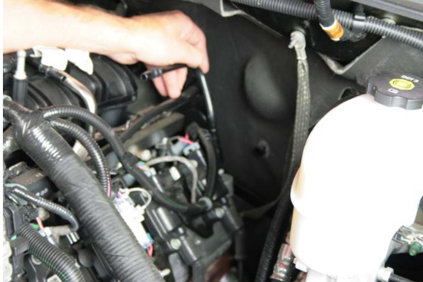
Step 16 Install female PCV tube in valve cover
