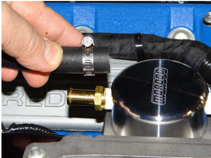
Step 19: Trim hose as needed, and install to Air Oil Separator using hose clamp.
