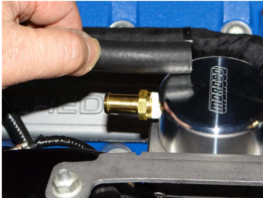
Step 19: Trim hose as needed, and install to Air Oil Separator using hose clamp.
