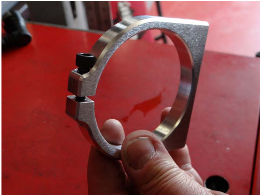
Step 8: Install 1/4-20x1 SHCS in billet clamp, do not tighten.
