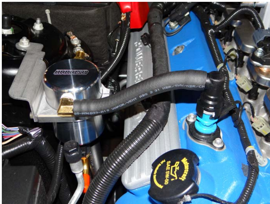
Step 18: Trim hose as needed and install to Air Oil Separator.
