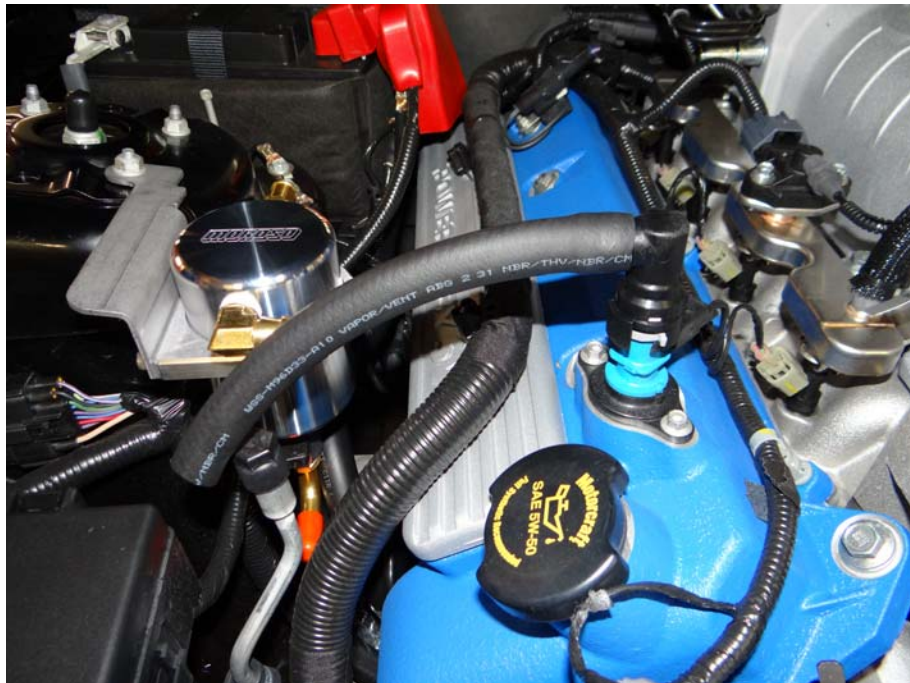
Step 14: Install 90 degree fitting to valve cover.
