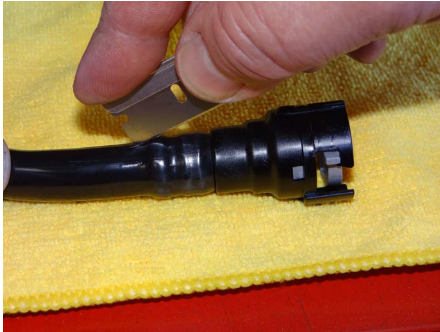
Step 5: Cut line from fitting as shown using razor blade.
