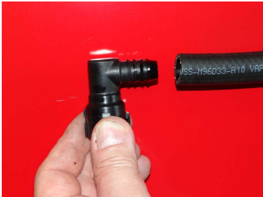
Step 11: Insert 90 degree fitting into 8" long 1/2" hose.
