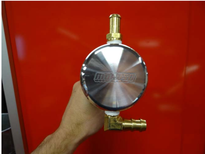
Step 15: Assemble Air Oil Separator as shown using Teflon Tape on all fittings.
