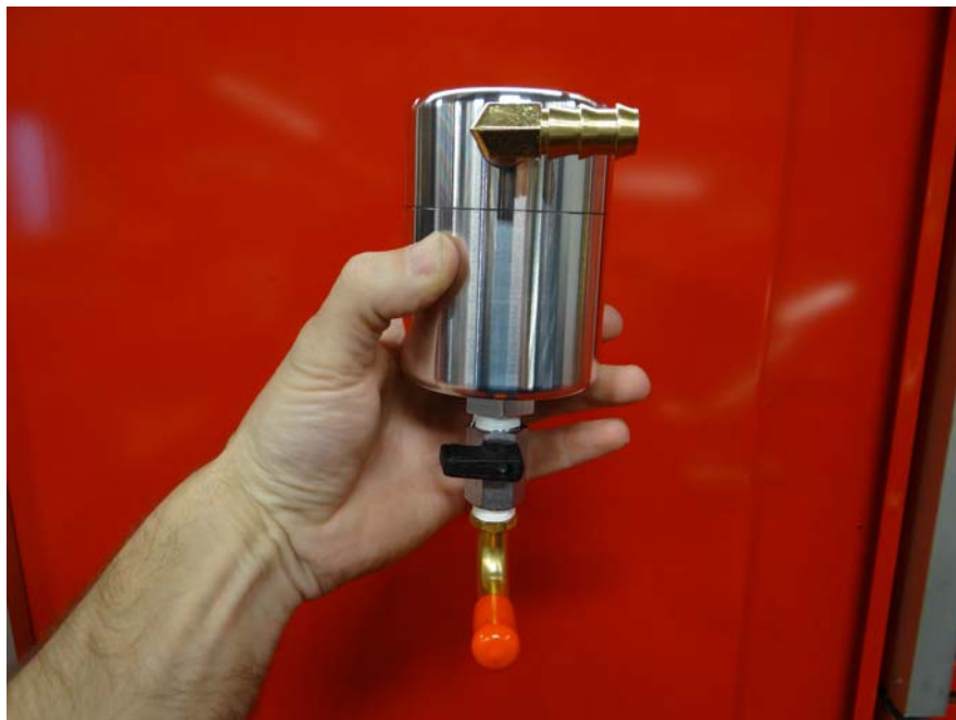
Step 15: Assemble Air Oil Separator as shown using Teflon Tape on all fittings.
