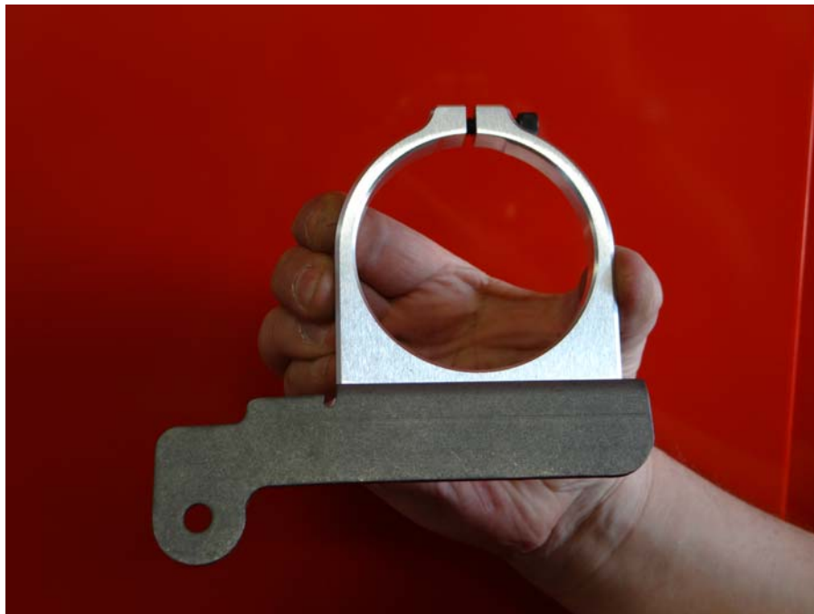
Step 9: Assemble billet clamp to stainless steel mount using (2) 1/4-20x5/8 SHCS.
