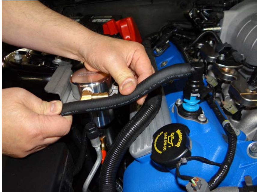
Step 18: Trim hose as needed and install to Air Oil Separator.
