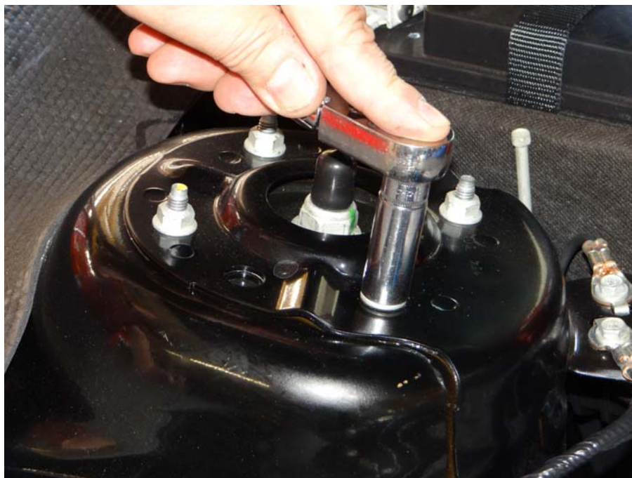
Step 7: Remove strut tower brace nut shown on passenger's side of vehicle.
