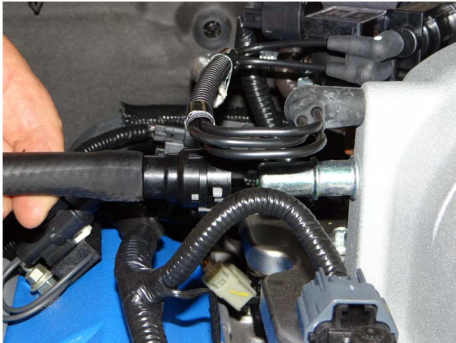
Step 13: Install straight fitting to intake.
