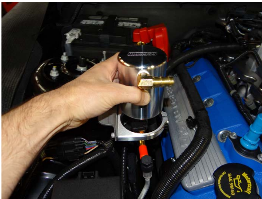
Step 16: Insert Air Oil Separator into billet clamp.
