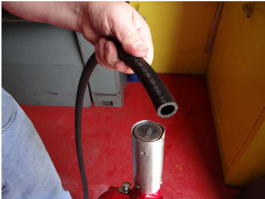
Note: heating with heat gun / hair dryer and lubrication is advised.
