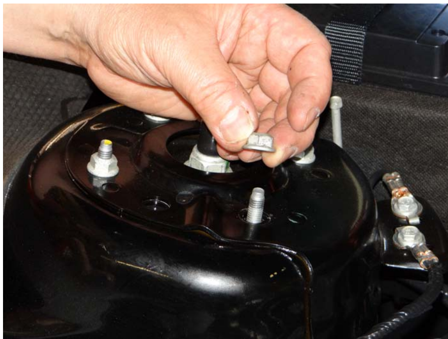
Step 7: Remove strut tower brace nut shown on passenger's side of vehicle.
