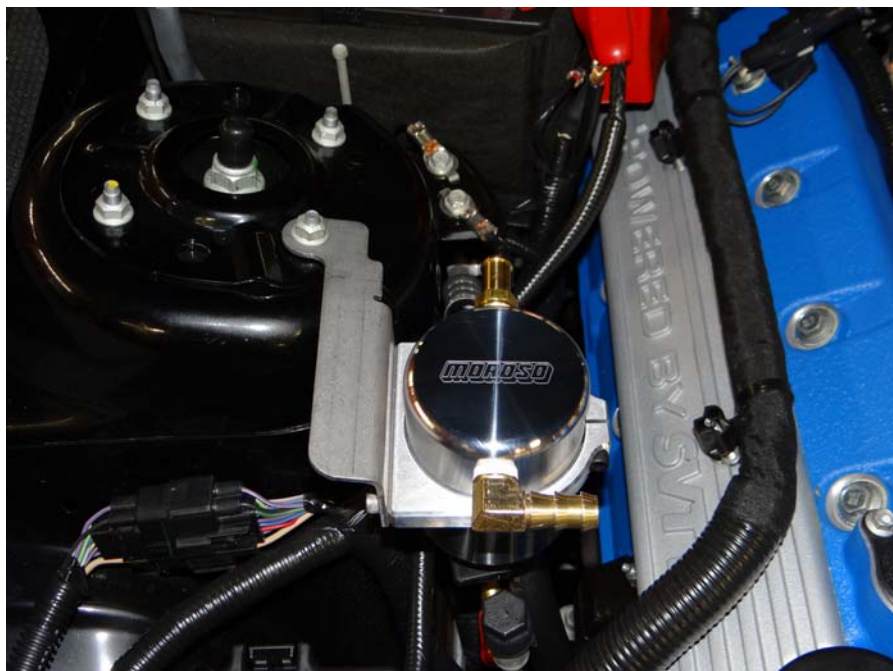
Step 17: Orientate Air Oil Separator as shown and tighten 1/4-20 SHCS.
