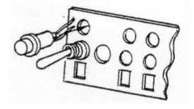
3. Install fuse holders from rear of panel
