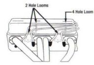
Use Silicone Spray Lube on plug wires to prevent cutting wires when installing into loom.
