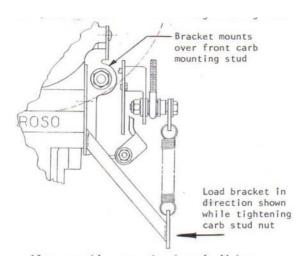
After assembly, move the throttle linkage through its full movement to insure the pump operating lever does not interfere or bind with the throttle return spring rod.
