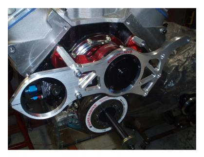
USING TWO 4.000" SOCKET CAPSCREWS, MOUNT THE OTHER SIDE OF THE BRACKET. PLACE THE SCREWS THROUGH THE BRACKET, THE TWO 2.700" SPACERS AND THE REAR ALTERNATOR SUPPORT AND THREAD THEM INTO THE SHORT, DRIVER'S SIDE STANDOFFS. DO NOT TIGHTEN THEM AT THIS TIME.
