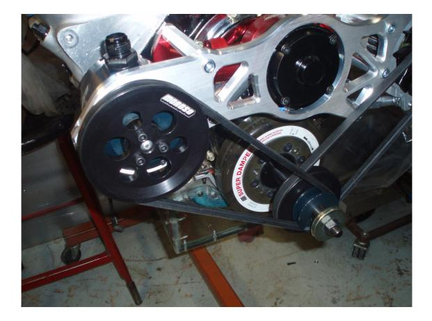
ENSURE THAT THE PULLEYS ARE IN ALIGNMENT. SWAPPING SPACERS ON THE DRIVE MANDREL CAN MAKE BIG ADJUSTMENTS. MOVING THE PUMP WITHIN THE BRACKET CAN DO MINOR ADJUSTMENTS.
