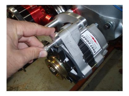
PLACE A 3/8" FLAT WASHER AND LOCK NUT ONTO THE ALTERNATOR BOLT AND LEAVE HAND-TIGHT. ONCE THE ALTERNATOR IS MOUNTED, USE A 5/16" ALLEN WRENCH AND TIGHTEN UP THE FOUR SOCKET CAPSCREWS THAT FASTEN THE MAIN BRACKET TO THE STANDOFFS.
