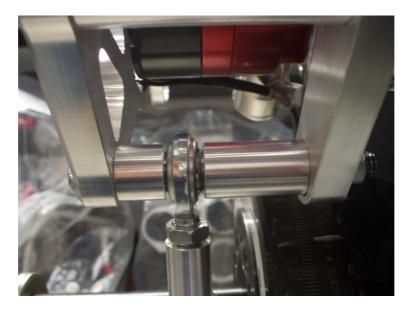
THE ALTERNATOR CAN NOW BE HUNG FROM THE UPPER MOUNTING HOLE IN THE MAIN BRACKET AS FOLLOWS. PLACE THE .590" SPACER INTO THE BORE OF THE REAR SUPPORT BRACKET AND HOLD IT THERE. WITH YOUR OTHER HAND, LIFT THE ALTERNATOR INTO POSITION BETWEEN THE BRACKETS, KEEPING THE SPACER IN PLACE. LET GO OF THE SPACER AND INSERT A 3.750 CAPSCREW THROUGH THE BRACKET, ALTERNATOR, SPACER AND REAR SUPPORT.
