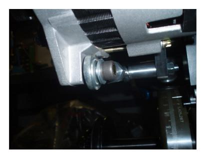
ONCE THE ADJUSTING LINK IS SECURED, THE DRIVE BELT CAN BE INSTALLED. TURN THE ADJUSTING LINK SO THAT IS AT IT'S SHORTEST LENGTH (ALTERNATOR TOUCHING WATER PUMP). WITH THE RECOMENDED 4.000 CRANK PULLEY (MOROSO PART#23523) INSTALL EITHER A 4L318 (31 ¾") OR A 4L320 (32") V-BELT (BOTH WILL WORK). ADJUST LINK TO ACHIEVE PROPER TENSION AND TIGHTEN BOTH JAM NUTS AND THE UPPER AND LOWER BOLTS.
