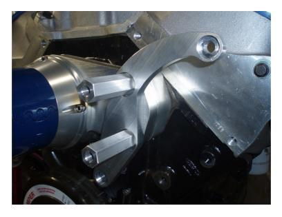
PLACE THE ALTERNATOR SUPPORT OVER THE STUDS ON THE DRIVER'S SIDE AND FASTEN IT DOWN WITH THE SHORTER, THREADED HEX STANDOFFS AS SHOWN. LEAVE ALL FOUR STANDOFFS HAND-TIGHT AT THIS TIME.
