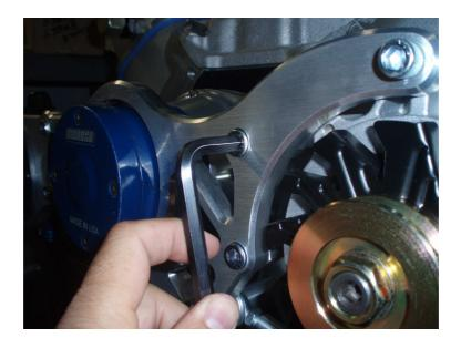
THE KIT PROVIDES BOTH AN 8MM AND A 3/8" FASTENER FOR THE LOWER LUG ON THE ALTERNATOR. THE ALTERNATOR IS TAPPED FOR 8MM THREADS SO, THE MATCHING FASTENER CAN BE USED AT THIS TIME TO COMPLETE THE INSTALLATION. FOR THOSE WHO WISH TO CONVERT TO A 3/8" BOLT, THE ALTERNATOR MUST BE DRILLED OUT. USE CARE AND MASK OFF ALL OPENINGS TO INSURE NO FOREIGN MATTER GETS INTO THE ALTERNATOR.
