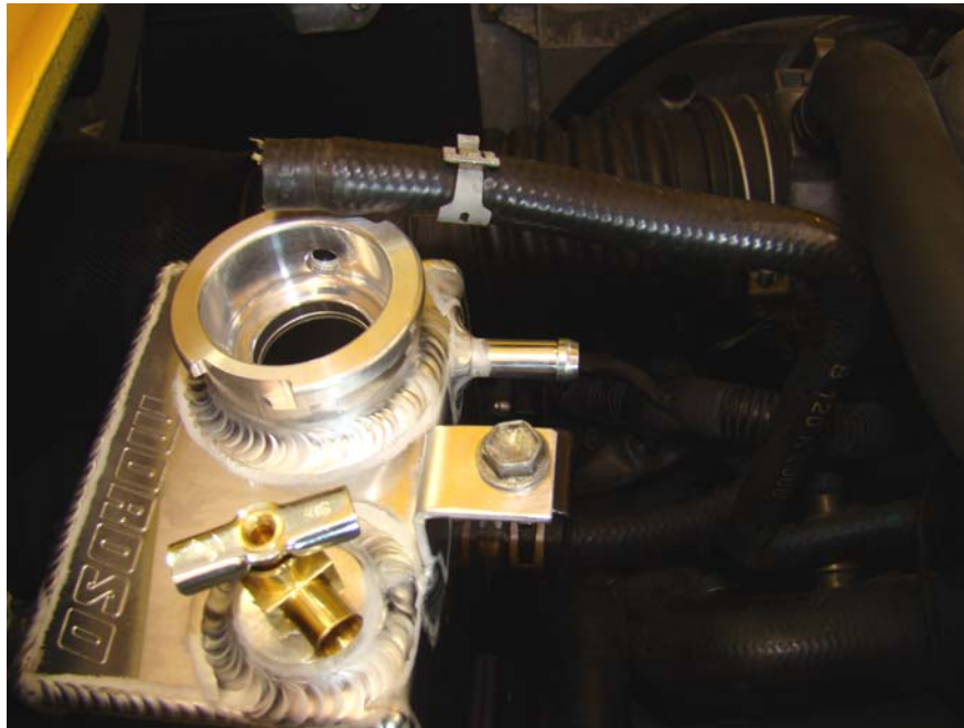
Step 24: Place line #2 next to tank as shown, mark desired length
