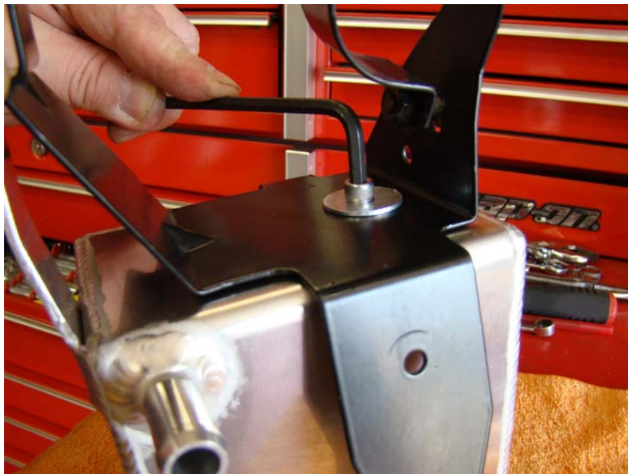
Step 15: Line up lower mount with stock mounting bracket hole
