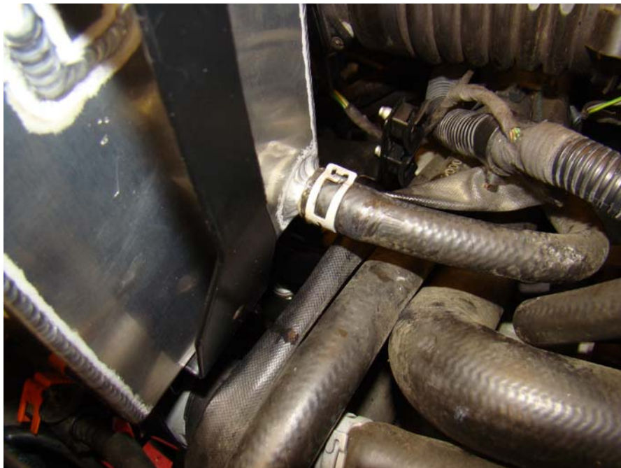
Step 23: Insert line #3 over nipple as shown and install clamp
