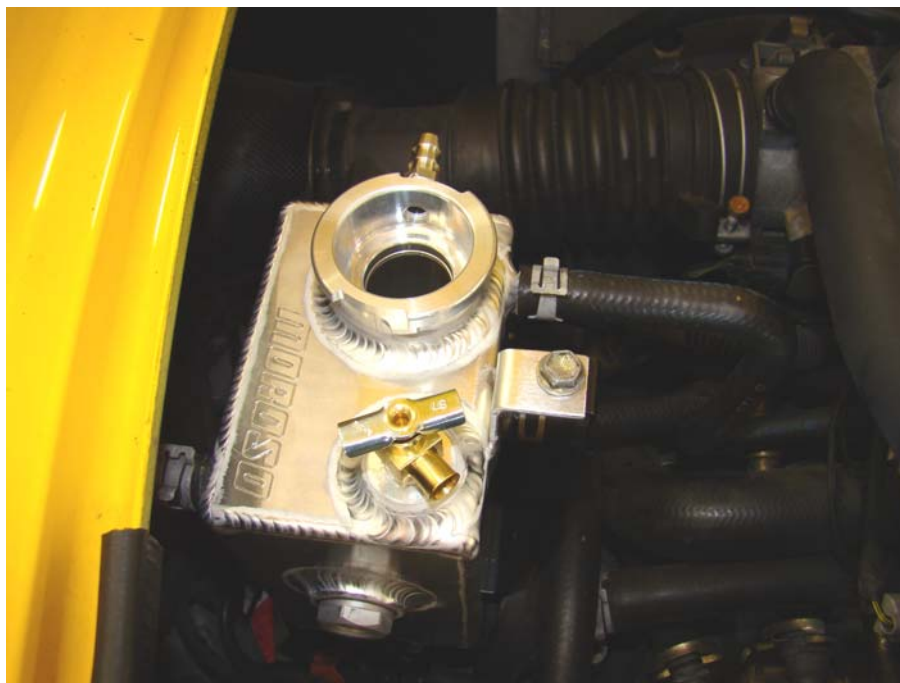
Step 26: Insert line #2 over nipple as shown and install clamp
