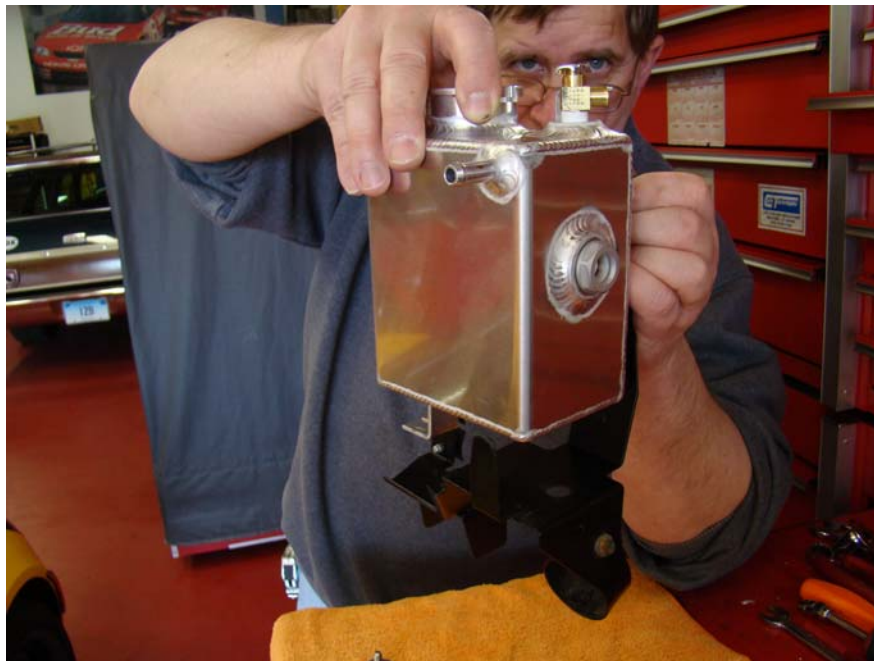
Step 12: Place coolant tank into stock bracket as shown
