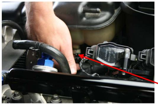
Step 5: Remove fluid sensor plug from bottom of tank (does not apply to all years)
