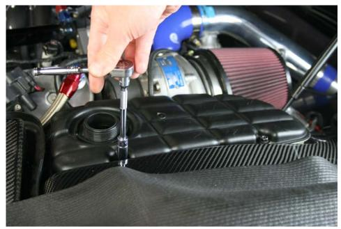
Step 3: Remove top (2) mounting nuts
