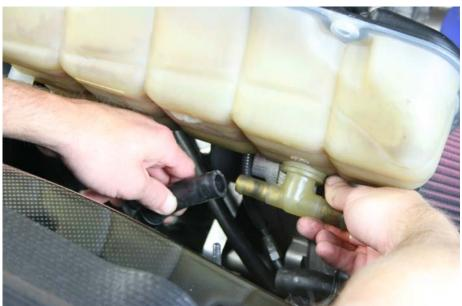
Step 7: Remove supply hoses from tank and remove tank from vehicle
