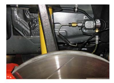
2. Be sure that the existing steel line connects to the end of the solenoid labeled "MC" and the other end of the solenoid goes to the side marked "Brake".
