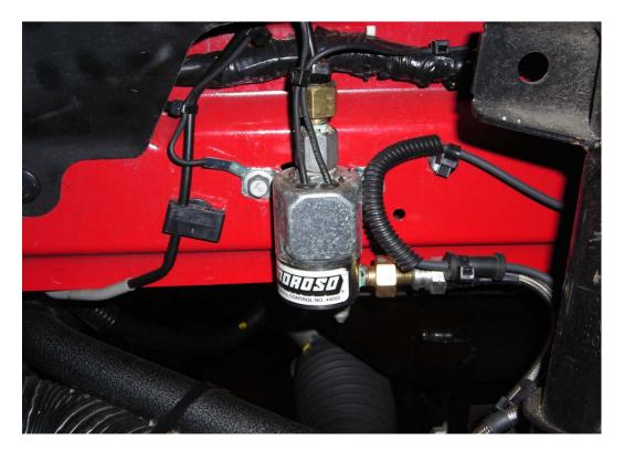
NOTE: Ground wire must be attached to mounting screw.
