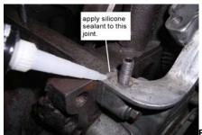
Apply silicone to the engine block at the rear housing cover and front timing cover seams as shown.
