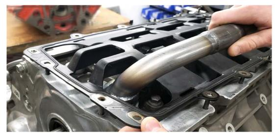
Step 7: Install the tray on the studs, and then lift the front of the tray while simultaneously inserting the pickup into the pump.
