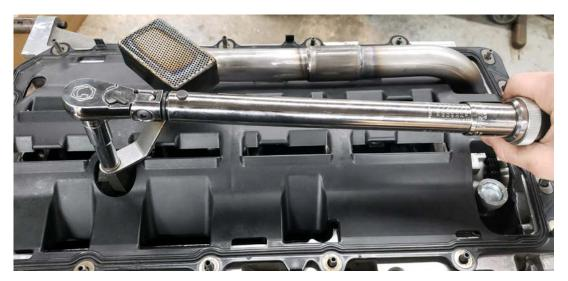
Step 9: Fasten the pickup bracket to the standoff using the provided 8mm flange head screw. Torque to 20 ft.-lbs.
