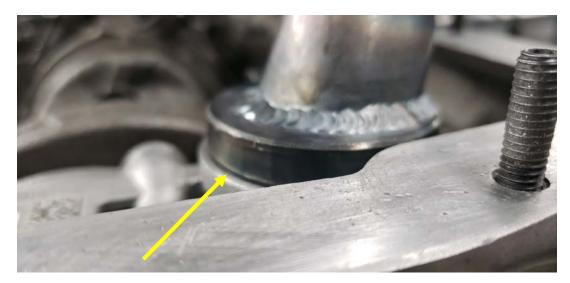
Step 8: Note: pickup must be fully seated in the oil pump.
