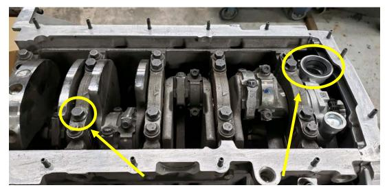
Step 1: Remove the highlighted main cap bolt, and O-ring from the pump.
