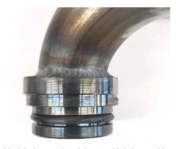
Step 6: Install the provided O-ring on the pickup and lubricate with engine oil before continuing.
